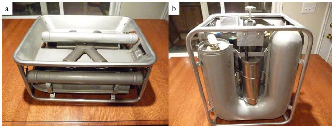
Figure 7.2: The M2 military burner viewed from the (a) side and (b) underside, which clearly shows the u-shaped fuel tank. Images are reproduced with permission from the photographer. Images were originally posted on [www.spiritburner.com](http://www.spiritburner.com).
