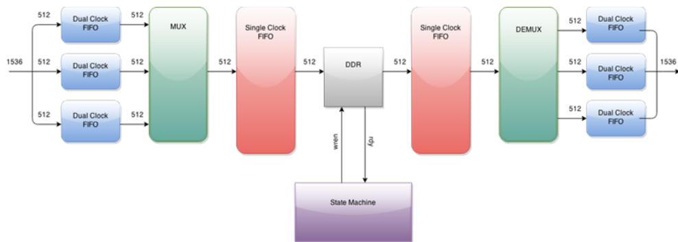
Figure 3.13: Modified frame buffer design and data path.
