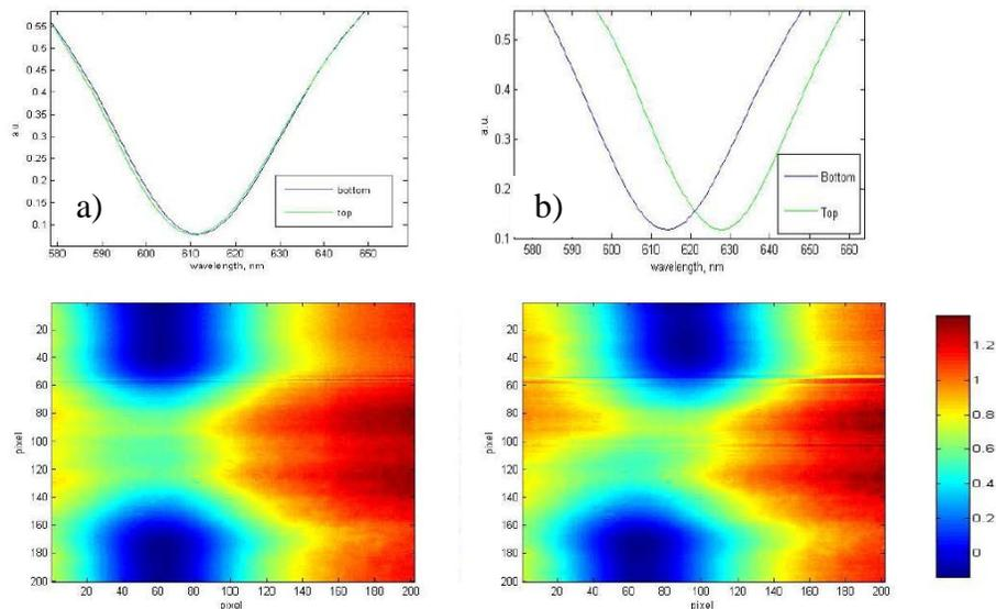
Figure 2. SPR data showing the functionalization of dual-pad sensor where a) is pre-electrografting and b) is post electrografting of diazonium salt onto the top pad. The top pad is the sensing pad while the bottom pad is the reference pad.
