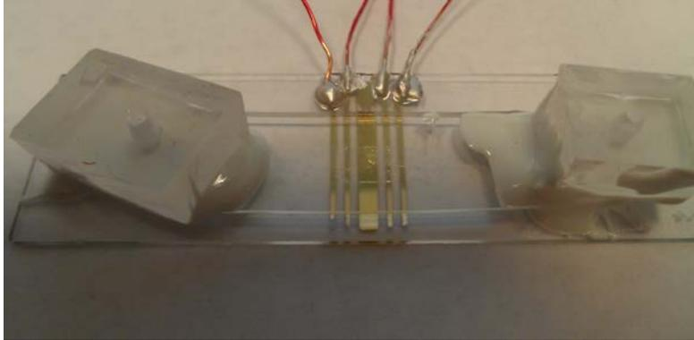
Figure 1. A picture of the EK-SPR sensor fully assembled. The first and last electrodes have independent voltages applied, while the middle two electrodes have the same potential applied to create appropriate electric fields.
