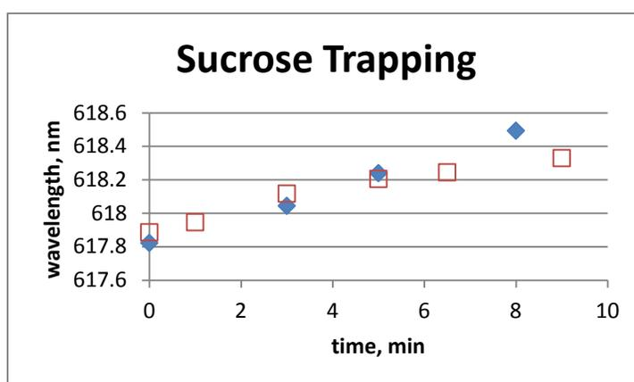
Figure 3. Data showing the capture and increase in concentration of a sucrose solution in varying electric fields. The solid diamonds represent an electric fields of  $600 \text{ V cm}^{-1}$  and the open squares represent an electric field of  $1900 \text{ V cm}^{-1}$ . A 1.5x increase of concentration over 8 min was observed in the  $600 \text{ V cm}^{-1}$  electric field. Both trials had a flow rate of  $0.0500 \text{ mL min}^{-1}$ .
