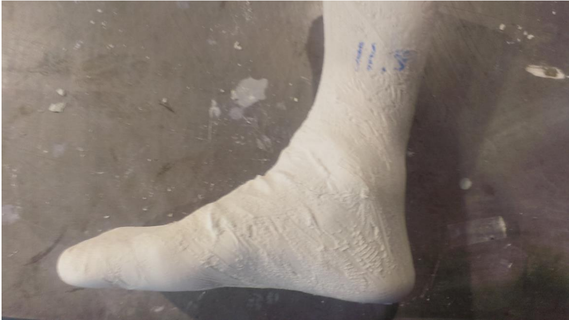
Figure 17: Image of an 11.5 size mold prior to sanding. Note the definition of the bottom and back of the mold.
