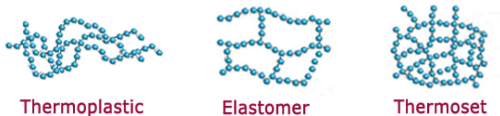
Figure 2: Image of the polymer chains forming thermoplastics, elastomers, and thermosets. [12]
