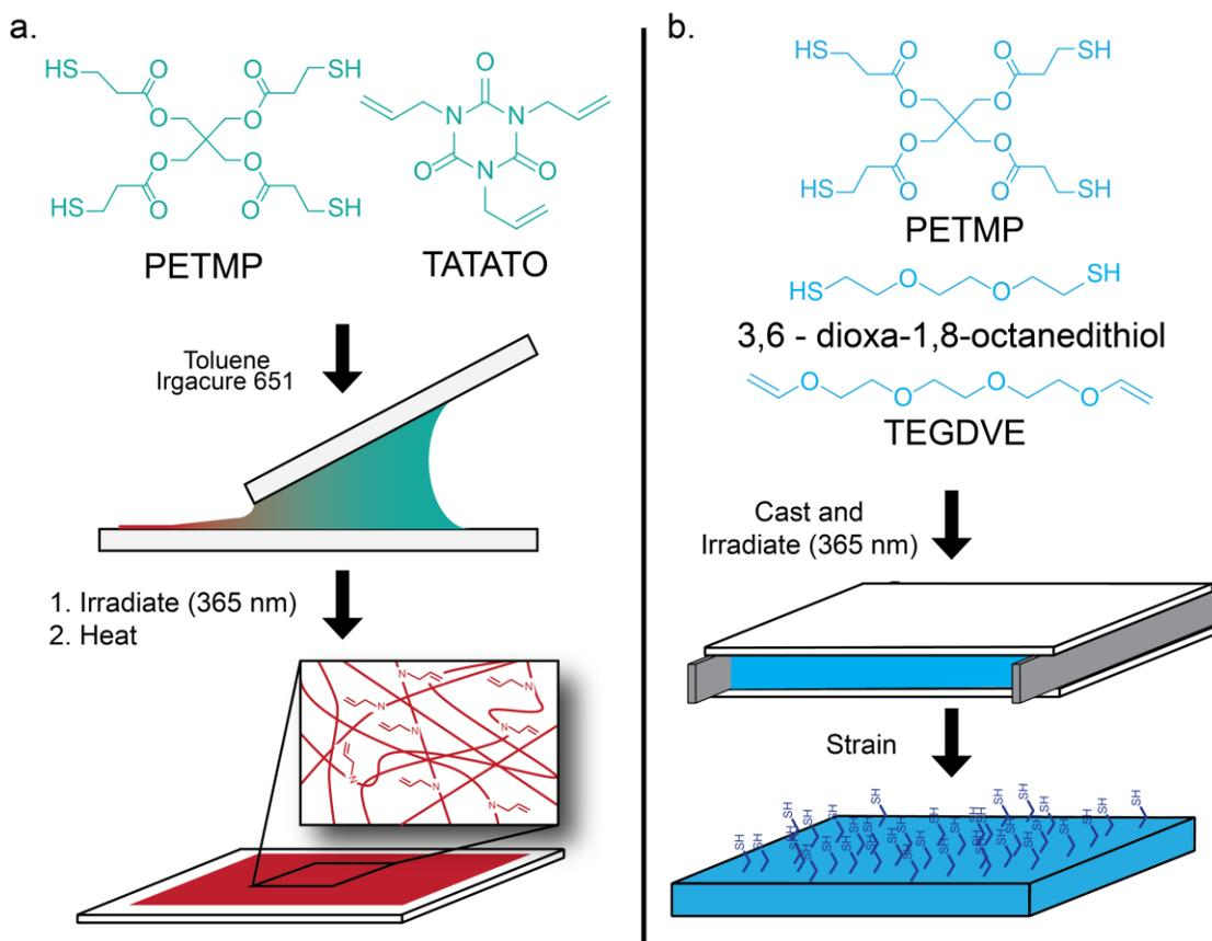
**Figure 4.2 Thiol-ene Film and Elastomer Formulation for Polymer Wrinkling.**
