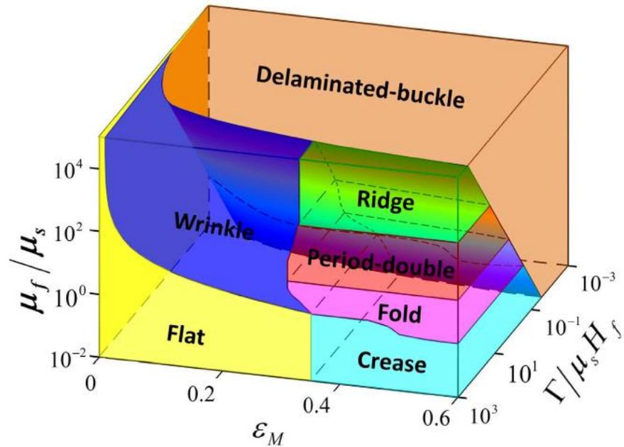
**Figure 1.3 Phase diagram for various wrinkling structures.** Type of topography is dictated by the film modulus to substrate modulus ratio ( $\mu_f/\mu_s$ ), the mismatched strain ( $\epsilon_m$ ) and normalized adhesion energy ( $\Gamma/\mu_s H_f$ ). Image adapted with permission from Wang, Q. and Zhao, X. *Scientific Reports*, **2015**, 5, 8887. Copyright 2015 Nature Publishing Group. [51]
