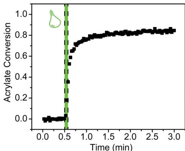
**Figure 3.4 Dark polymerization observed in the free radical polymerization.** Despite irradiating the thin film elastomer substrate for only 5 seconds (green highlighted region), acrylate conversion continues to rise for another 30 seconds before hitting a plateau conversion. This dark polymerization is likely due to diffusion limited radical termination.
