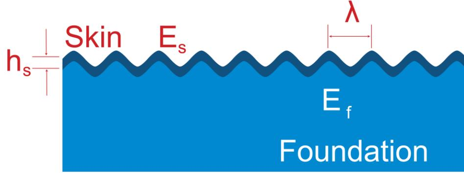
**Figure 1.1 Wrinkle Formation Schematic.** Wrinkles form when a thick foundation exerts lateral compressive stresses on a thinly adhered skin layer. Wrinkle wavelength is a function of skin (or film) modulus ( $E_s$ ), foundation (or substrate) modulus ( $E_f$ ) and thickness of the film,  $h_s$ .
