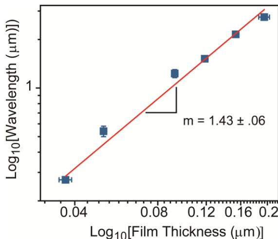
**Figure 4.7 Observed thickness scaling deviations of the wrinkle wavelength as film thickness approaches 40 nm; the wavelength scaling on thickness becomes  $\lambda \sim h^{1.43}$  instead of the expected  $h^1$ .**
