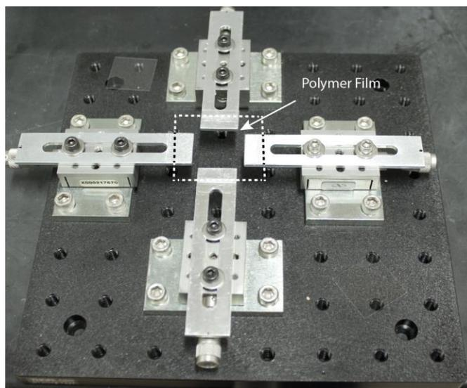
**Figure 2.1** Linear stage set up for uniaxial and biaxial strain. Polymers were cut, centered, and held in place with tape. Samples were then strained and released in a sequential manner.
