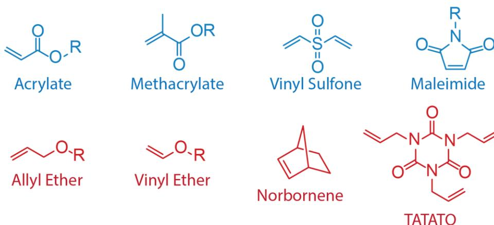
**Figure 1.5 Typical thiol and ene structures.** Number of functional groups and molecular architecture (i.e., ring structures) dictate thermomechanical properties of resultant crosslinked network. The blue enes are electron deficient enes, requiring the use of a nucleophile or base catalyst. The red enes are electron rich, requiring a radical initiator to catalyze the reaction. Many of these compounds are commercially available.
