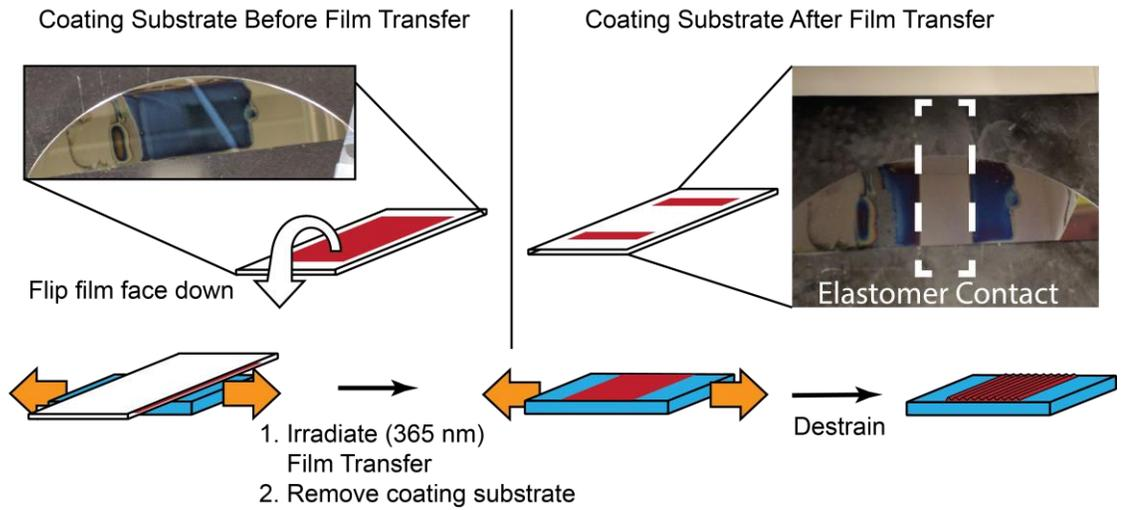
**Figure 4.3 Film Transfer of Flowcoated Film onto a Thiol-ene Elastomer for Wrinkle Formation.** a) Thin films are flowcoated and polymerized on a silicon wafer (or glass slide) and before they are placed in contact with a strained thiol-ene elastomer (b). Irradiation initiates reaction of the excess vinyls at the film interface with the excess thiols at the elastomer interface, to form a covalently attached laminate. The coating substrate is subsequently removed by submerging the entire
