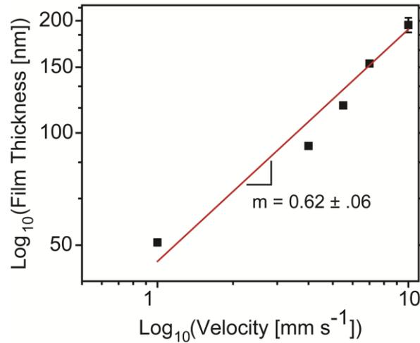
**Figure 4.5**  $\text{Log}_{10}(\text{Film Thickness})$  plotted as a function of  $\text{Log}_{10}(\text{Velocity})$  yields an 0.62 scaling, consistent with the Landau-Levich theory.
