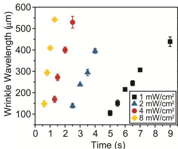
**Figure 3.5 Wrinkle wavelength vs Time and Intensity.** As light controls the film formation necessary to generate wrinkles, both light intensity and irradiation time dictate the size of wrinkle features. Increasing both the intensity and time will lead to increasing wrinkle wavelengths.
