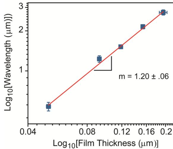
**Figure 4.6** As predicted by Equation 2, wrinkle wavelength scales with  $h$ .
