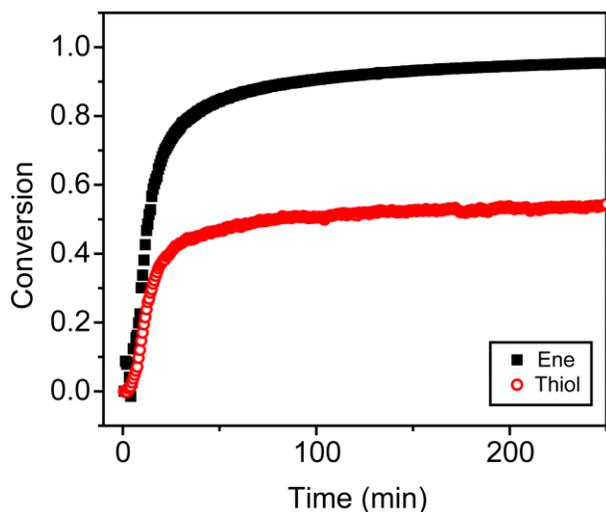
**Figure 3.3 Conversion data of thiol and ene during elastomer formation.** In situ FTIR measurements of the 1:2 PETMP:TEGDA system confirms quantitative conversion of thiol and roughly 50% conversion of the acrylates, which is consistent with the thiol:ene stoichiometry used in formulation.
