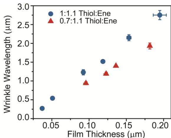
**Figure 4.8 Wrinkle wavelength vs film thickness for films of different moduli.** Wrinkle wavelength can be tuned through modulus of the thin films via monomer structure and/or thiol:ene stoichiometry. Thiol:ene formulations using 1:1.1 (modulus = 1.9 GPa) yield larger wrinkle wavelengths as compared to 0.7:1.1 formulations (modulus = 1.5 GPa). A similar concept can be applied to the elastomer substrate as well.
