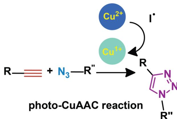
**Figure 5.2 Photo-Copper Catalyzed Azide Alkyne Reaction.** A photoinitiator radical reduces copper(II) to copper(I) which will trigger reaction between the azide ( $-N_3$ ) and alkyne ( $-C\equiv C$ ) resulting in the formation of the triazole ring.
