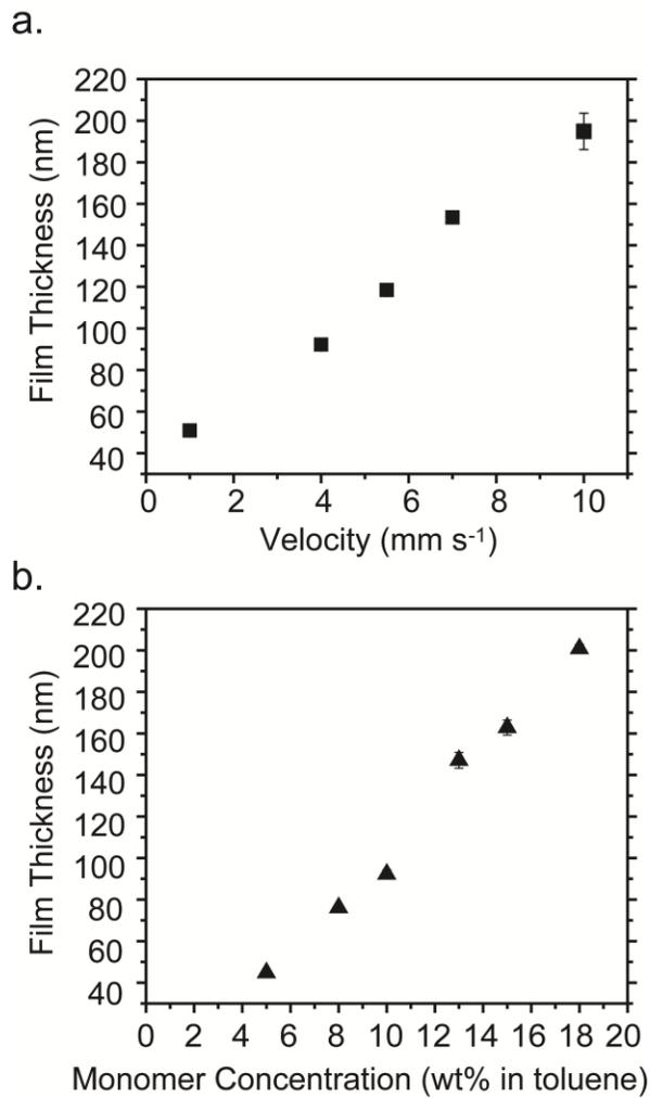
**Figure 4.4 Film thickness versus coating velocity and monomer concentration** A) Film thickness plotted as a function of velocity shows a linear increasing trend. As velocity increases, more monomer is left behind on the flowcoated substrate, thereby increasing the film thickness. B) The film thickness increases with increasing monomer concentration.
