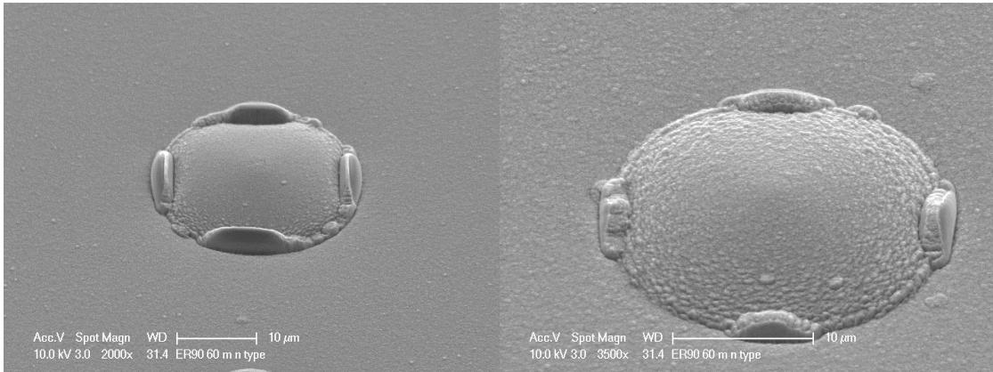
Figure 57 Result of 30/20/7.5 sccm of Ar/Cl<sub>2</sub>/O<sub>2</sub>. Pattern transfer is inconsistent across the sample.
