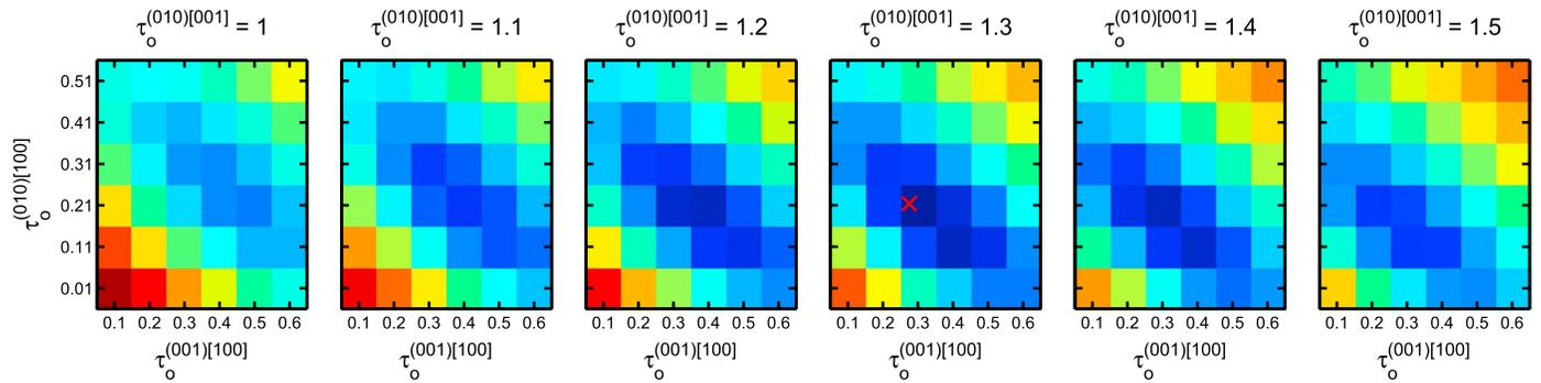
**Figure 4.** Sensitivity testing of the mechanical model to variations in the relative strengths of the three active slip systems,  $\tau_o^{\alpha}$ . Results are presented for the pseudo-Taylor model. The color scale indicates the total misfit between predicted strain rates and observed strain rates, as described in section 3.1. Colder colors indicate lower misfit. The red cross indicates the best fit set of parameters determined with the genetic algorithm.
