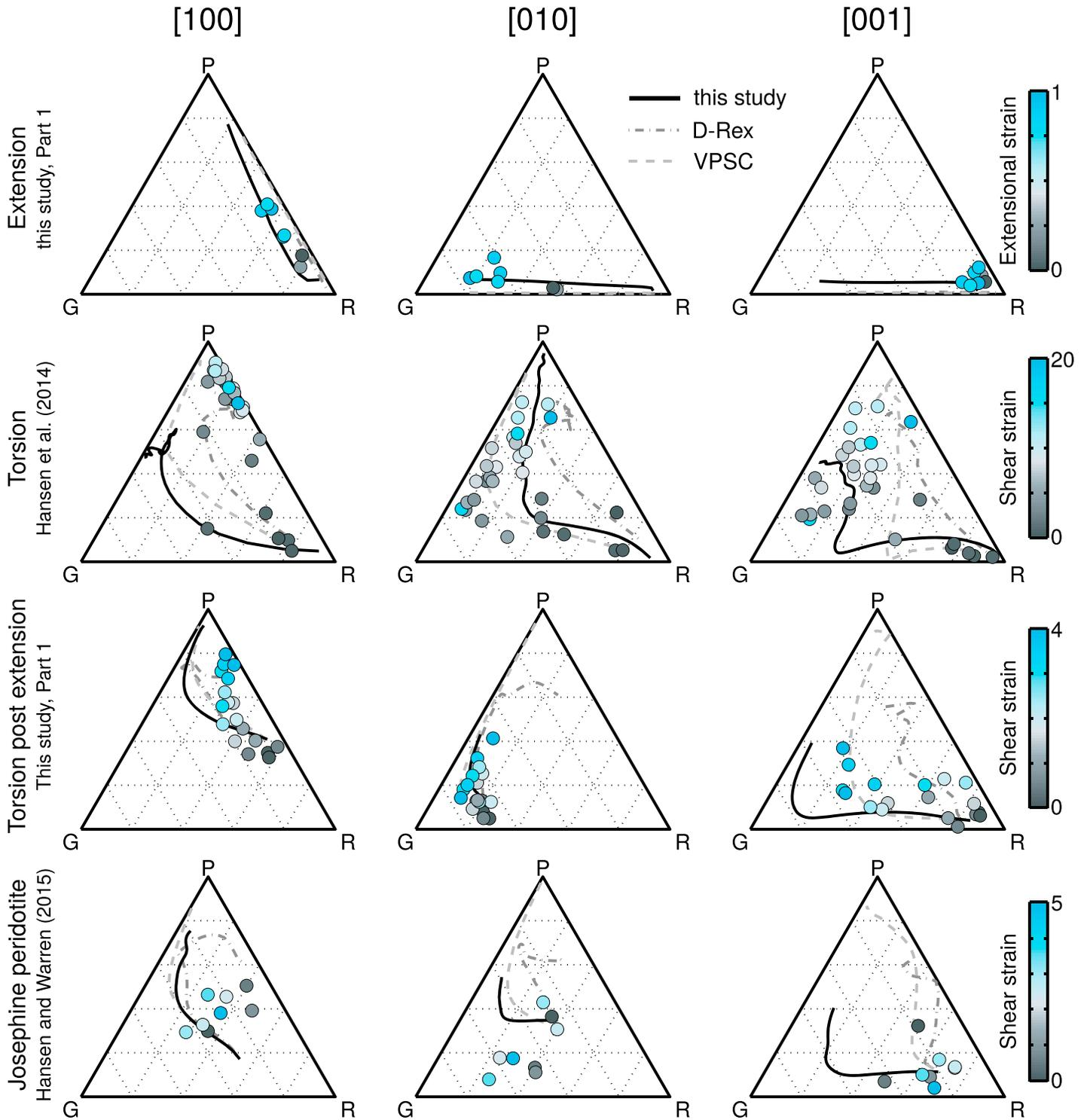
**Figure 9.** Comparison of texture shape from deformation experiments (circles) and numerical simulations (lines). Data sources are as in Figure 7. *P*, *G*, and *R* refer to the point, girdle, and random components of the axis distributions and are derived from the eigenvalues of the orientation tensor as described in the text. An animation of these data represented in pole figures is included in the supporting information (Movie S2).
