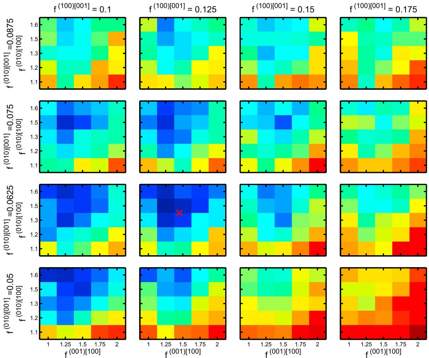
**Figure 5.** Sensitivity testing of the textural evolution model to variations in the relative rotation rates of the four active slip systems,  $f^\alpha$ . The color scale indicates the total misfit between predicted textures and observed textures, as described in section 3.2. Colder colors indicate lower misfit. The red cross indicates the set of best fit parameters determined with the genetic algorithm.
