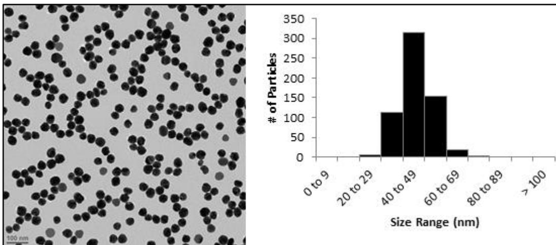
Figure 8: A) TEM micrograph of c-AgNPs in stock solution. Scale bar is 100 nm. B) Size Distribution of c-AgNPs in stock solution. Mean TEM diameter =  $44.9 \pm 7.2$  nm, n = 607.
