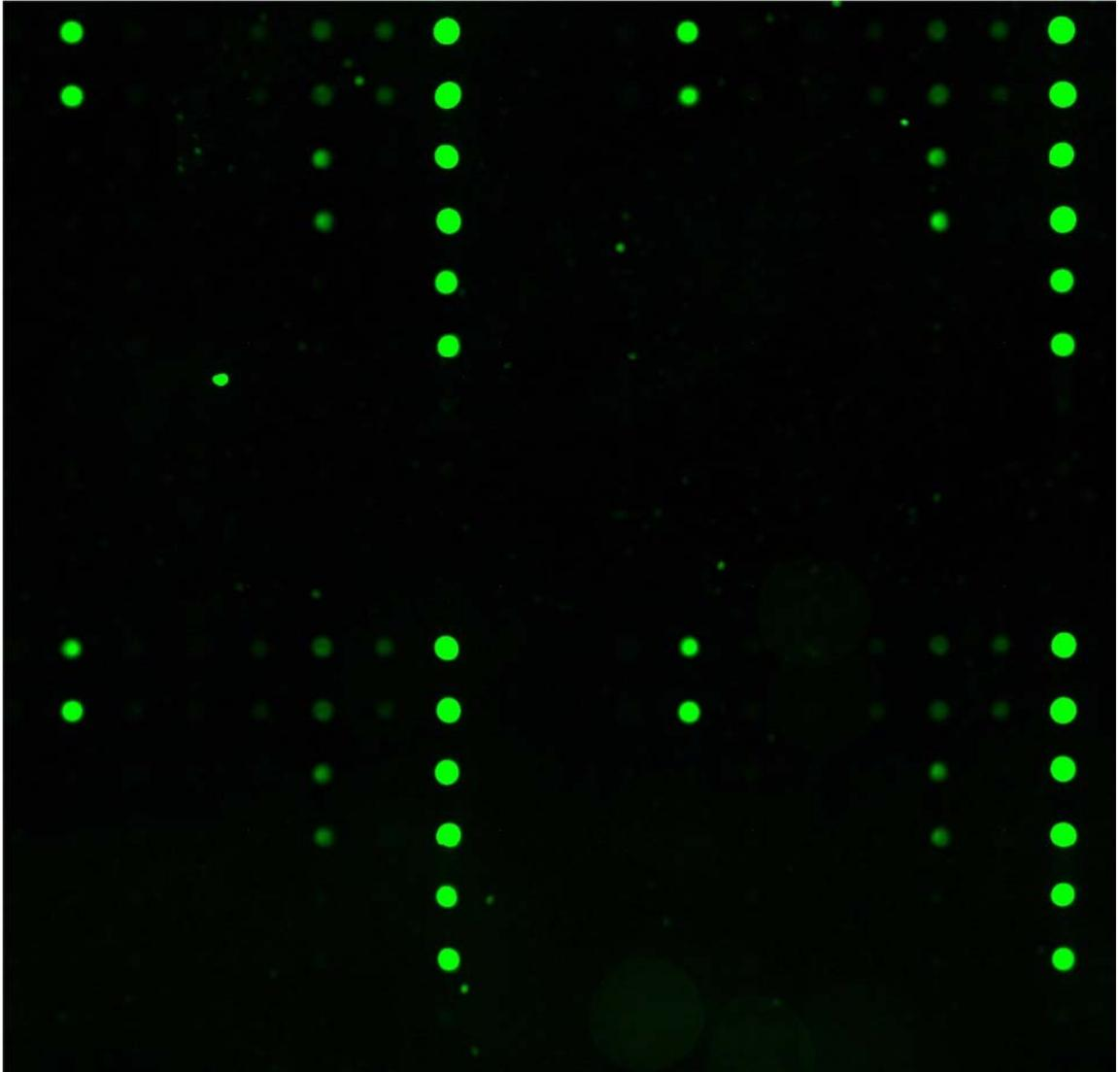
**Figure 3.17 Scanned Image of Unknown I Hybridized to the AI Microarray.** In a hybridization experiment with unknown I, 10  $\mu\text{g}$  of Alexa555 labeled aRNA was hybridized to the array at 50°C for 3 hr. Fluorescent signals are observed for matrix, NA1, and HA5 elements. The hybridization pattern is consistent with a type A influenza subtyped as H5N1 belonging to the Eurasian clade.
