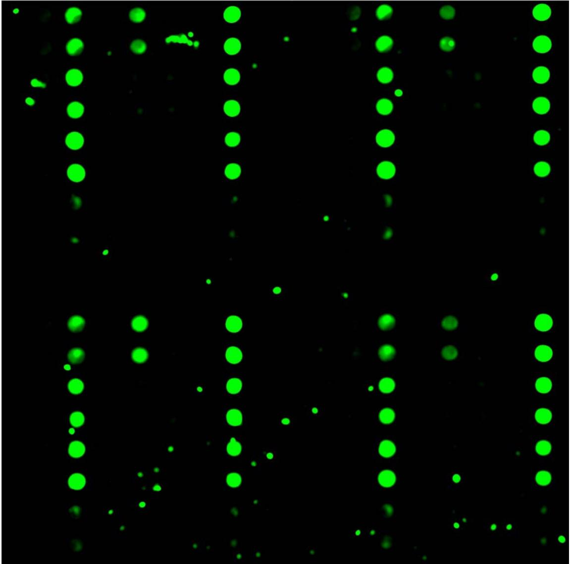
**Figure 3.13 Scanned Image of Unknown F Hybridized to the AI Microarray.** In a hybridization experiment with unknown F, 10  $\mu\text{g}$  of Alexa555 labeled aRNA was hybridized to the array at 50°C for 3 hr. Fluorescent signals are observed for matrix gene elements. The hybridization pattern is consistent with a type A influenza of undetermined subtype.
