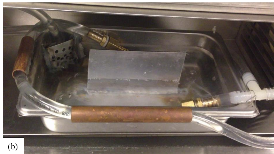
Figure 6.1 Water-assisted pulsed light treatment setup. (a) Water-assisted pulsed light experimental setup; (b) circulating flume washer.
