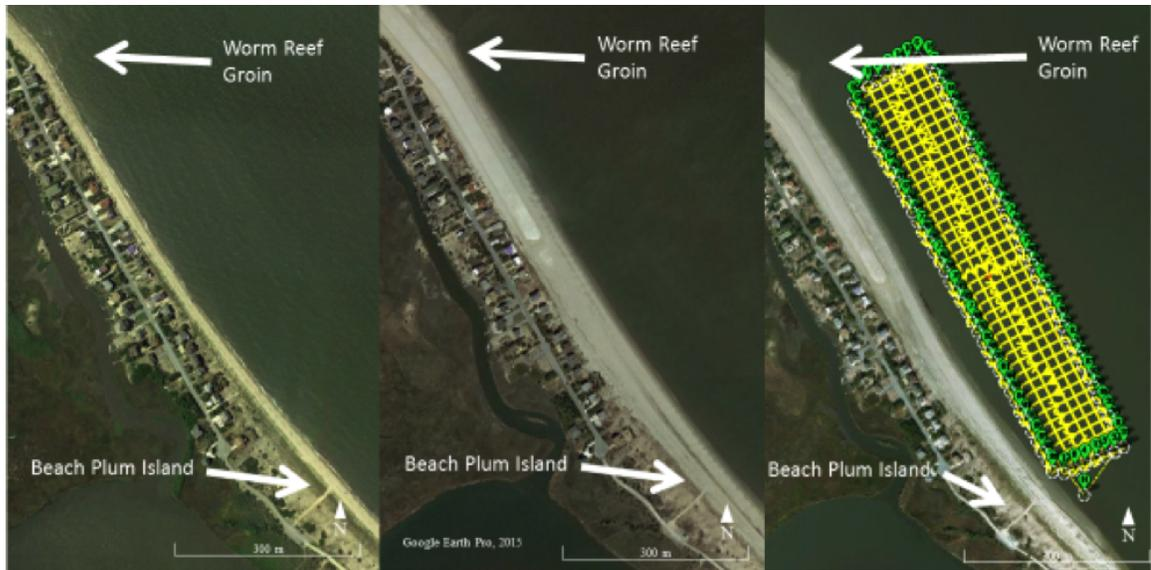
**Figure 2.1:** Pre-nourishment (2015), Post-nourishment(2017), 13.78 km path surveying over a 117,950-square meter area.
