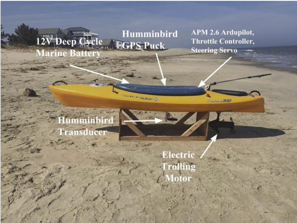
**Figure 1.1:** Bubbles' hardware configuration
