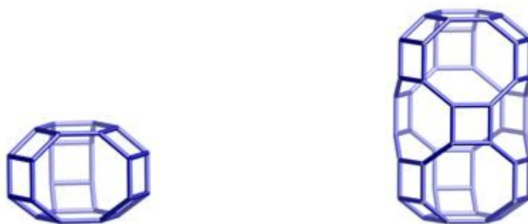
Figure 8.2. The composite building units ( gme -left, aft -right) of AFX zeolite
