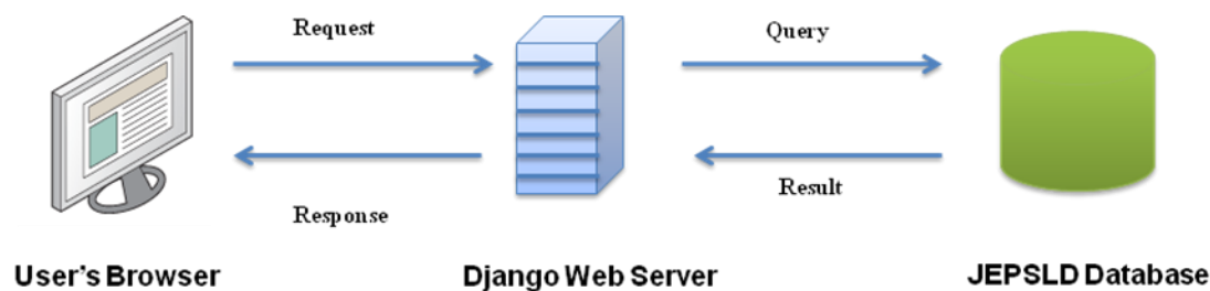
Figure 4.2: Architecture of the Django user interface and the JEPSLD database
