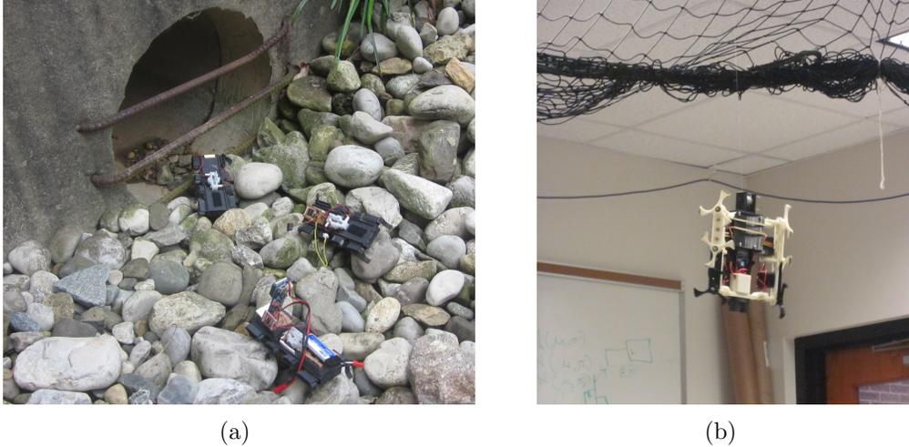
**Figure 1.3:** Examples of the domain of application of miniature legged robots. (a) Pipe inspection. (b) Building surveillance and intelligence.
