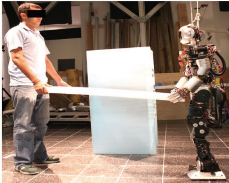
**Figure 6.1:** A human carrying an object with the humanoid robot HUBO (photo courtesy of Prof. P. Oh, Drexel University).
