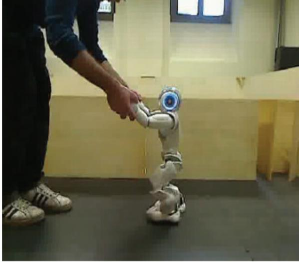
**Figure 2.2:** Guiding the motion of NAO via physical interaction. Photo adopted from [7].
