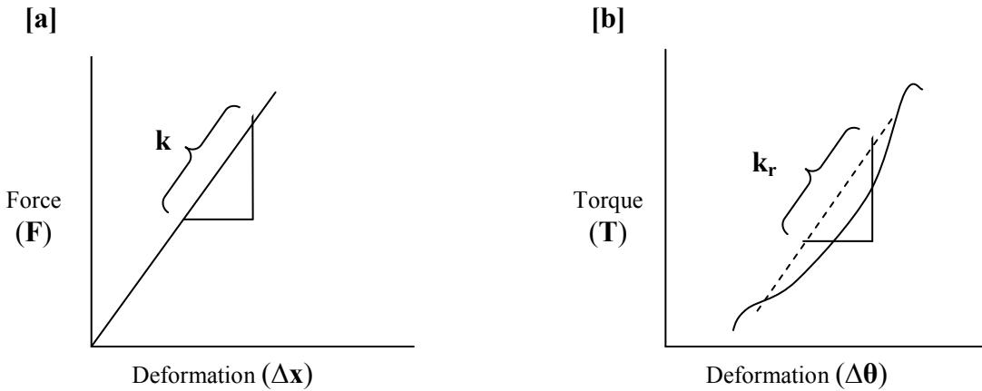
**Figure 1.1** Hooke's Law applied to (a) linear stiffness and (b) torsional stiffness.
