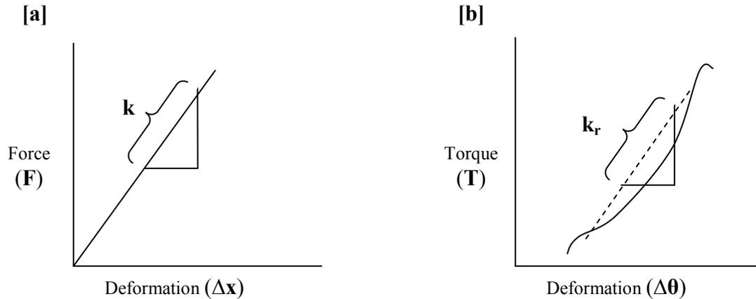
**Figure 1.1** Hooke's Law applied to (a) linear stiffness and (b) torsional stiffness.
