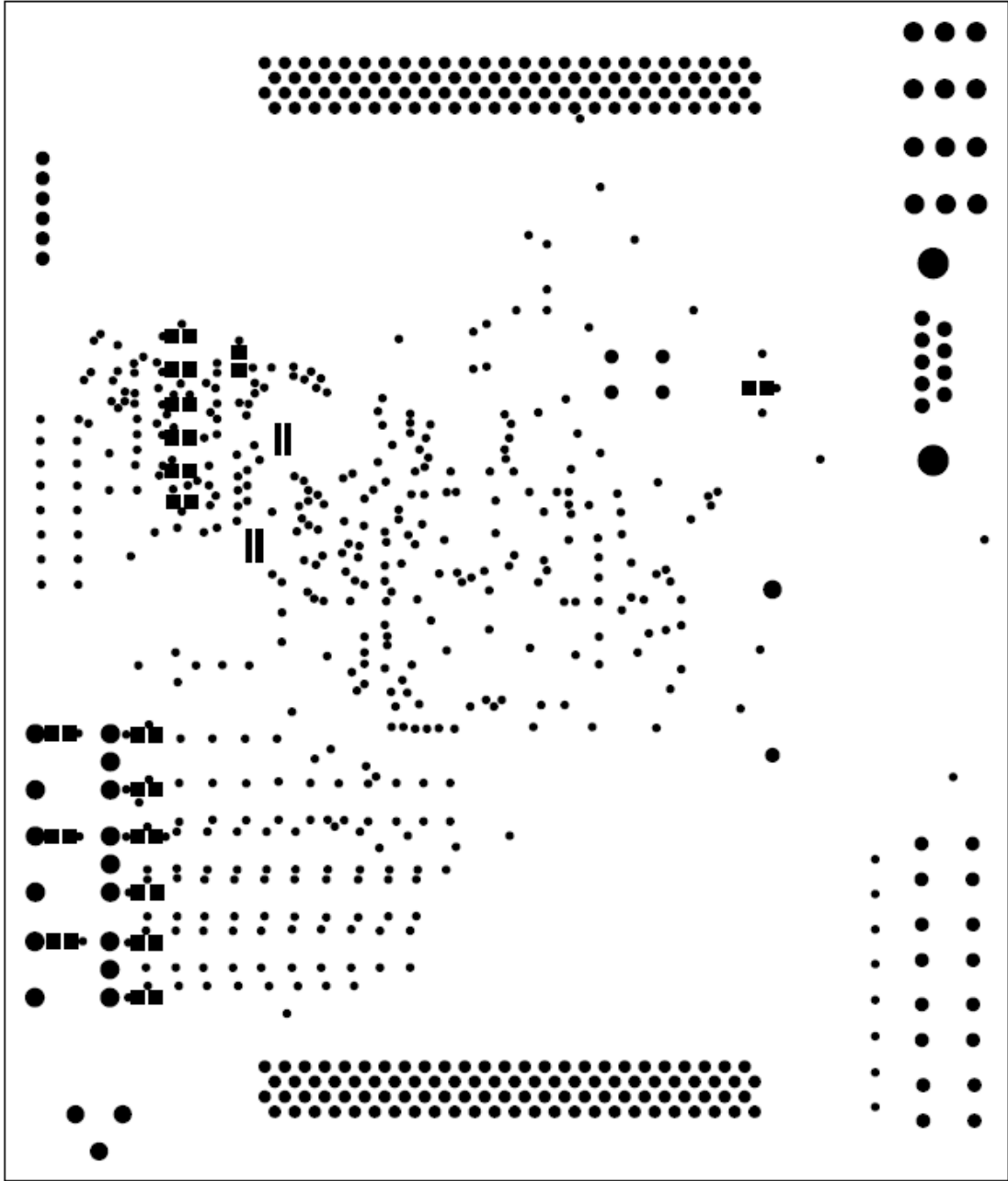
Figure 0-7 – PCB Bottom Soldermask Layer
