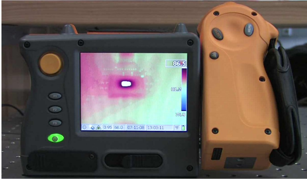
Figure 4-4 – FPGA Dissipating Heat Captured by the Thermal Imager
