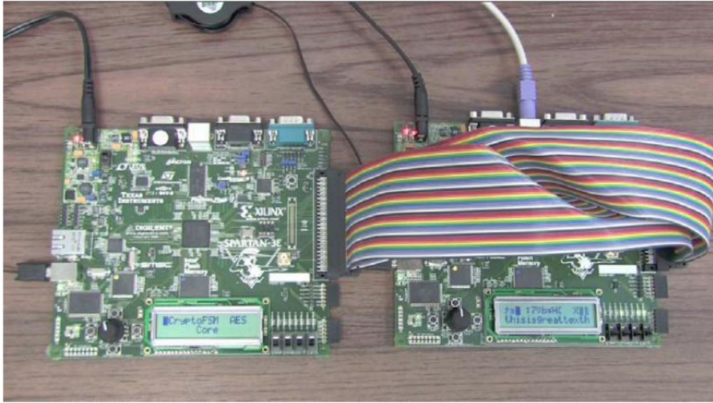
Figure 5-1 – Trojan Detection System Setup Using Spartan-3E Starter Boards
