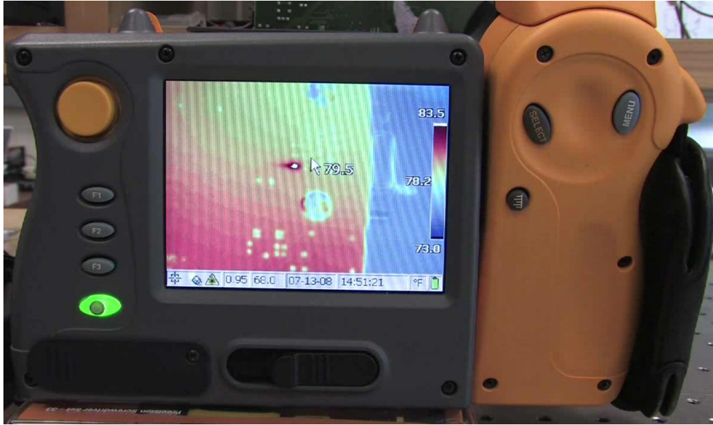
Figure 4-3 – Resistor Dissipating Heat Captured by the Thermal Imager
