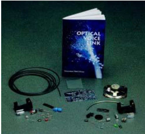
Figure 3-2 – Optical Voice Link Kit by Industrial Fiber Optics
