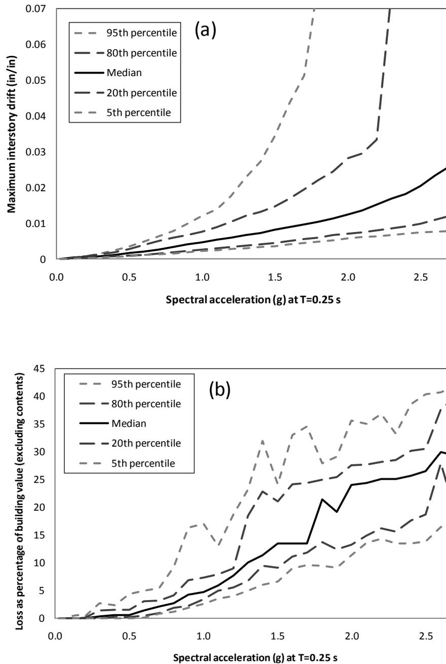
**Figure 6. (a) Maximum inter-story drift vs. ground motion intensity for the base case building, and (b) loss (in percentage of building value, excluding contents) vs. ground motion intensity for a single typical ground motion for the base case building**
