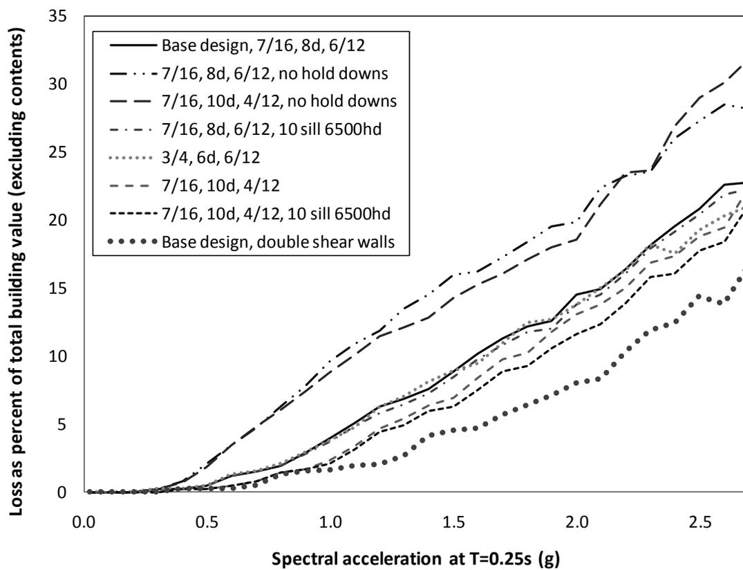
**Figure 4. Loss (in percentage of building value, excluding contents) vs. spectral acceleration at T=0.25s, median curve for 8 selected building variants (10 sill 6500hd refers to assembly type 10 in Table 1, with hold downs with an allowable uplift load of 28.91 kN (6500 lbs.))**
