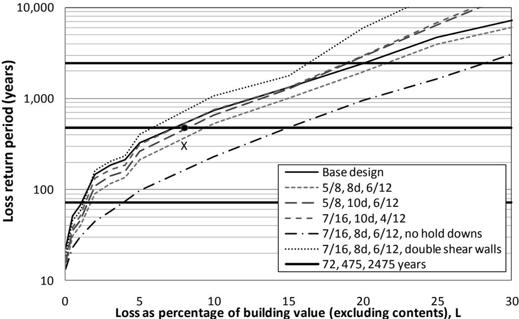
**Figure 8. Loss return period (years) vs. loss (in percentage of building value, excluding contents), for selected building variants**
