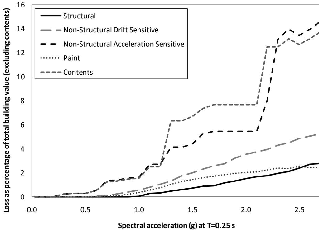
**Figure 5. Loss (in percentage of building value, excluding contents) vs. spectral acceleration at T=0.25s, median curve for each major assembly type, base case building**
