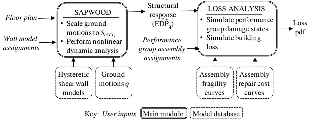
**Figure 1. Schematic of new seismic loss simulation model for woodframe buildings, as applied for a specified building variant  $B$ , and ground motion intensity  $S_{a(T1)}$**
