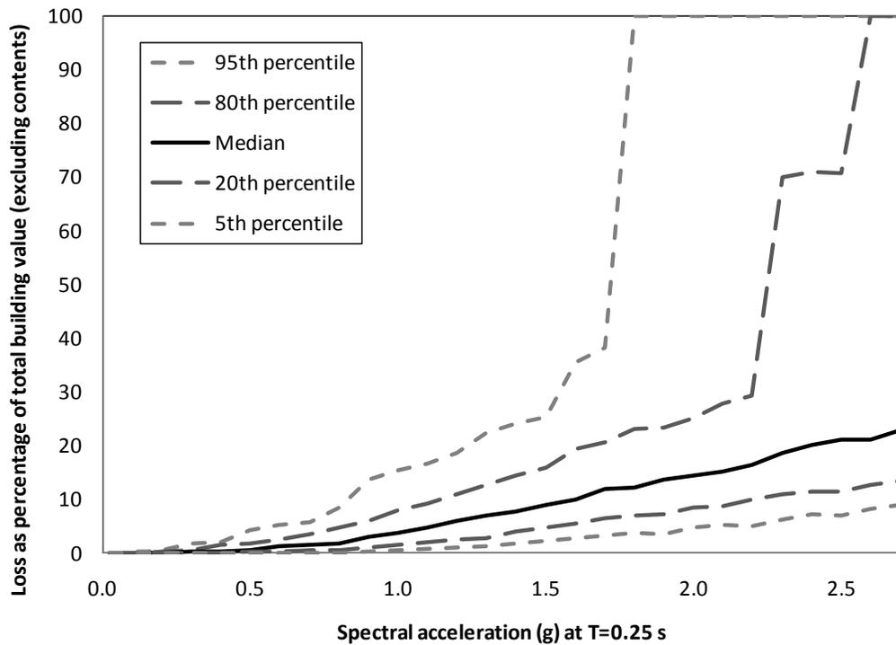
**Figure 3. Loss (in percentage of building value, excluding contents) vs. spectral acceleration at T=0.25s, median with percentiles for the base case building**
