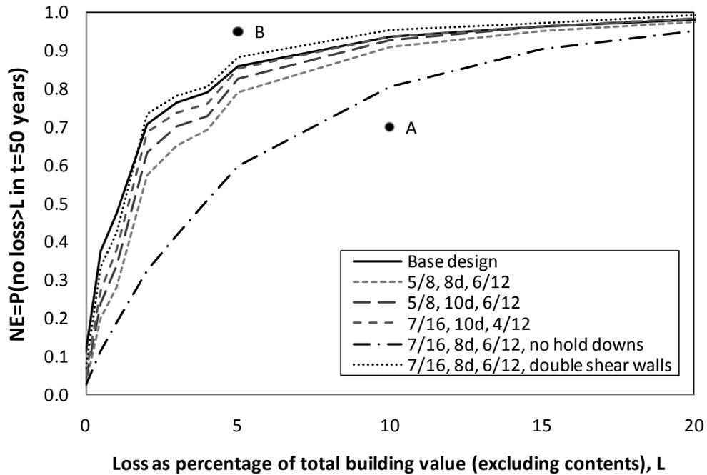
**Figure 7. Probability loss does not exceed loss L (in percentage of building value, excluding contents) in t=50 years vs. Loss L, for selected building variants**
