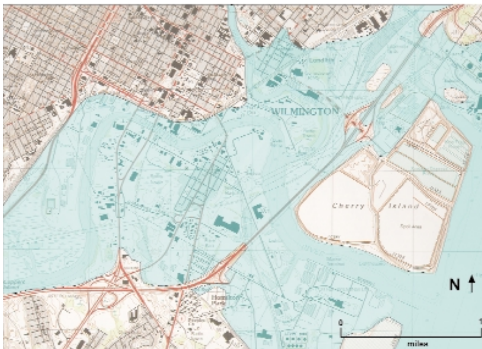
Figure 18: Portion of Wilmington-South quadrangle map (USGS, 1993) showing areas of Wilmington along the Delaware and Christiana flooded during the storm surge of the Hurricane of 1878 and that could be flooded by a similar storm today.
