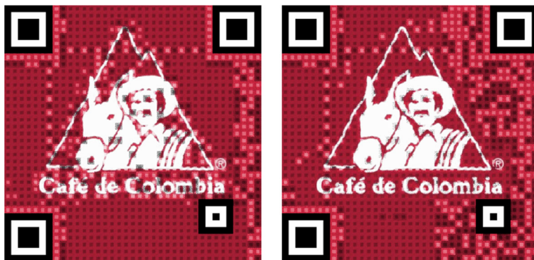
Fig. 4 Binary standard aesthetic QR code generated to reduced only contrast as proposed in [31] (left) and binary baseline QR code Q_b generated using the proposed binary QR code adaptation method (right). QRnet with equal parameters ( P_{max} = 0.3 and R = 0.5 ) was used in both cases for QR code image embedding
