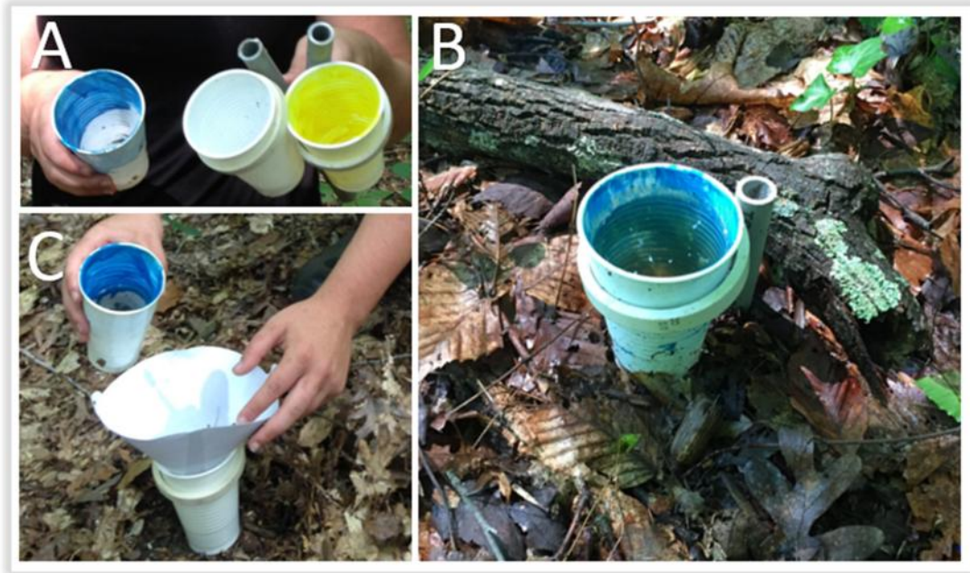
Figure 1.2: Cup trap design A) Cups were painted fluorescent blue, fluorescent yellow or left white. B) PVC stands were used to prevent cups from tipping C) Insects were removed by pouring cups through a paint strainer.
