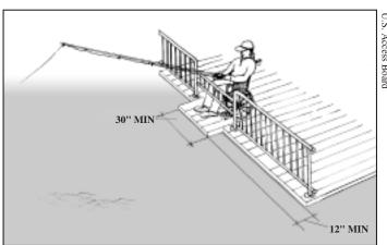
Figure 1. A 12-inch deck extension without edge protection.
