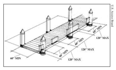
Figure 2. Clear spaces are needed along the length of a pier to provide access to a boat slip for people with disabilities.
