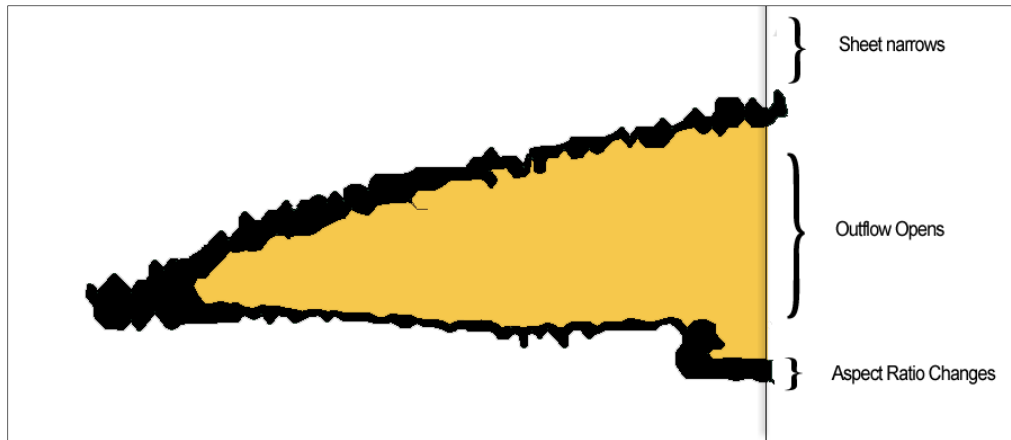
Figure 34 A breakdown correlating the in-plane reconnection geometry to the x-line contour. Regions in white correspond to regions where the current sheet is not yet narrow enough to support reconnection. The black band represents the transition region between 'slow' and 'fast' reconnection. It is in that region. In the yellow region the diffusion region has attained a fixed aspect ratio of approximately 10:1, which means that open outflows have developed.
