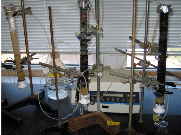
Figure 1 Unsaturated column set-up. Columns present were a sand only control, 10% PL biochar with sand, and 10% WD biochar with sand. Flow of 1 \text{ mL min}^{-1} was applied to the top of the columns using a peristaltic pump and effluent collected from tubing connected to the bottom of the columns.
