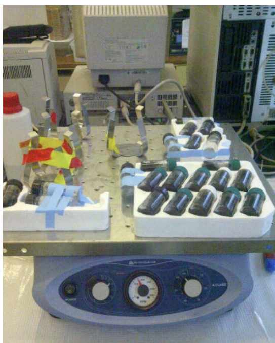
Figure 2 Batch experiment shaker set-up. Vials with 0.2g biochar and 10mL of NH 4 Cl solutions were prepared and shaken horizontally at 150 rpm for 24 hours to reach equilibrium of NH 4 + adsorption.
