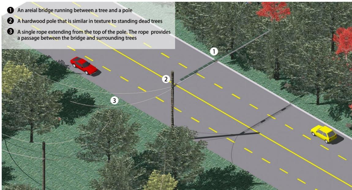
Figure 6.13: 3D View of an Aerial Bridge Web
