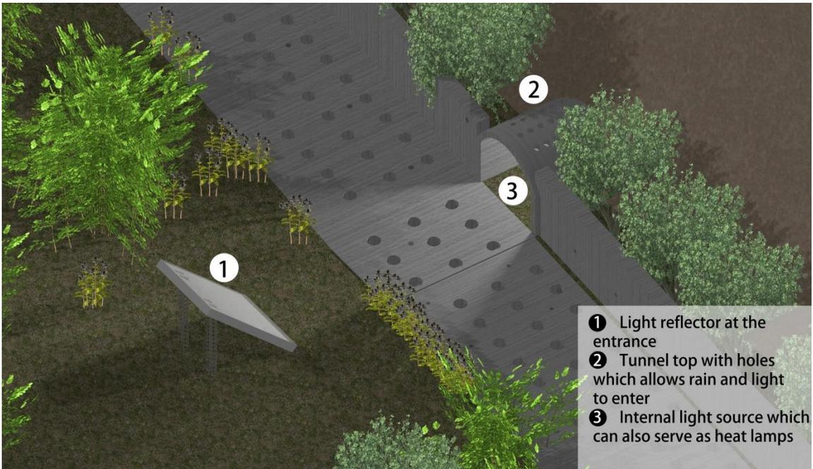
Figure 6.34: Lighting System for *R. pipiens* Tunnel
