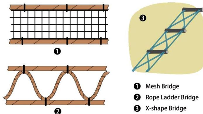
Figure 6.10: Models of Squirrel Aerial Bridge. Taken from: RSNE, 2016, p. 2.
