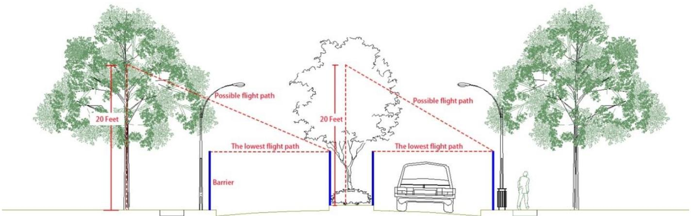
Figure 6.19: Height of Barrier for a Median Strip and Trash Bins
