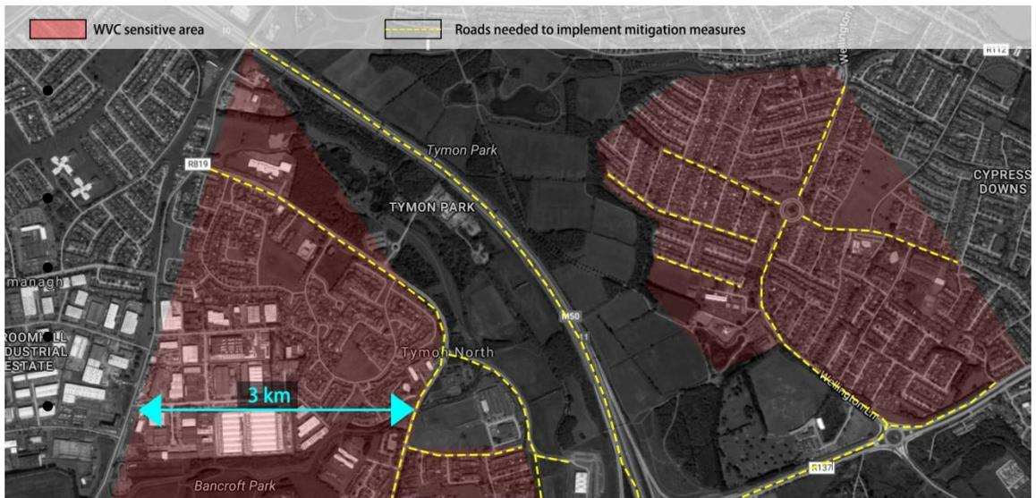
Figure 6.17: Using the Maximum Flight Distance to Define WVC Hotspots
