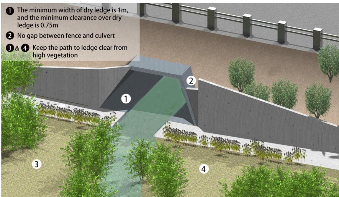
Figure 6.32: Culvert Retrofitting with Dry Ledge
