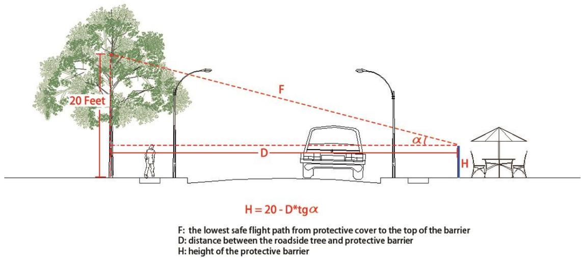
Figure 6.18: Height of Barrier for an Open-air Restaurant on a Road without a Median
