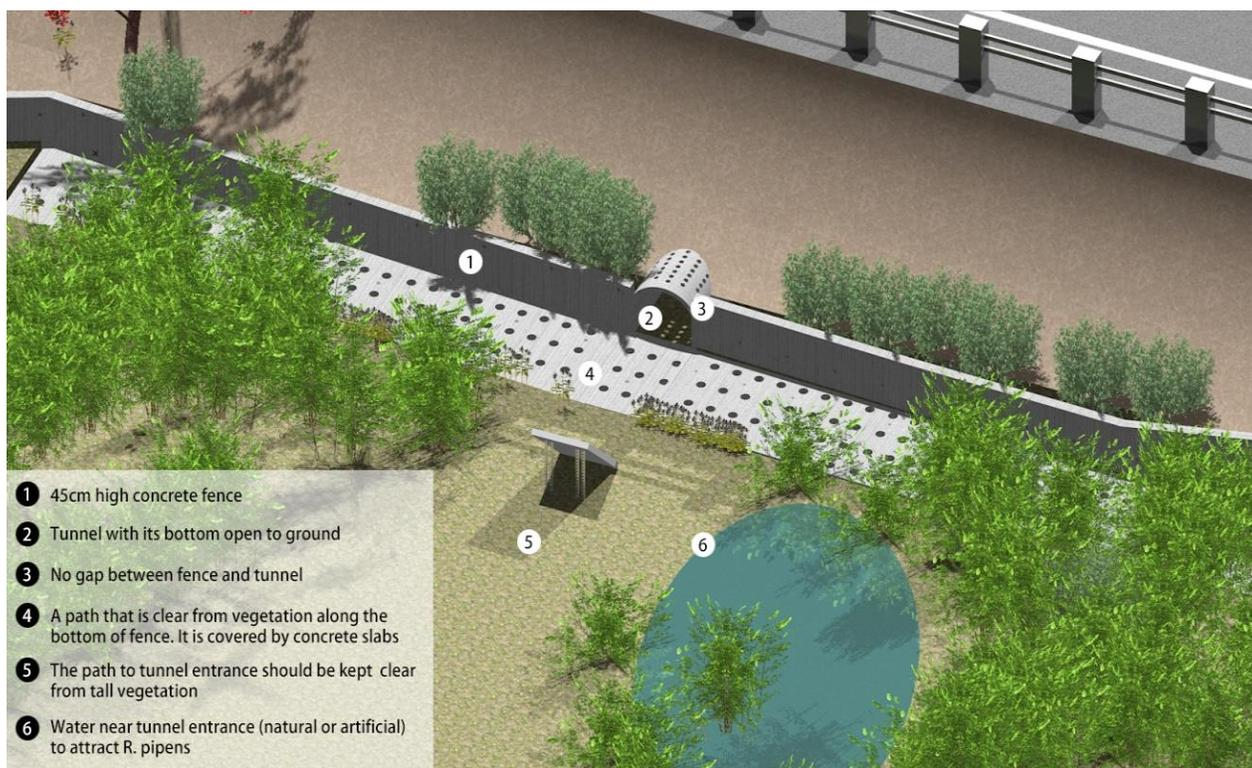
Figure 6.35: 3D view of *R. pipiens* Tunnel and Fence
