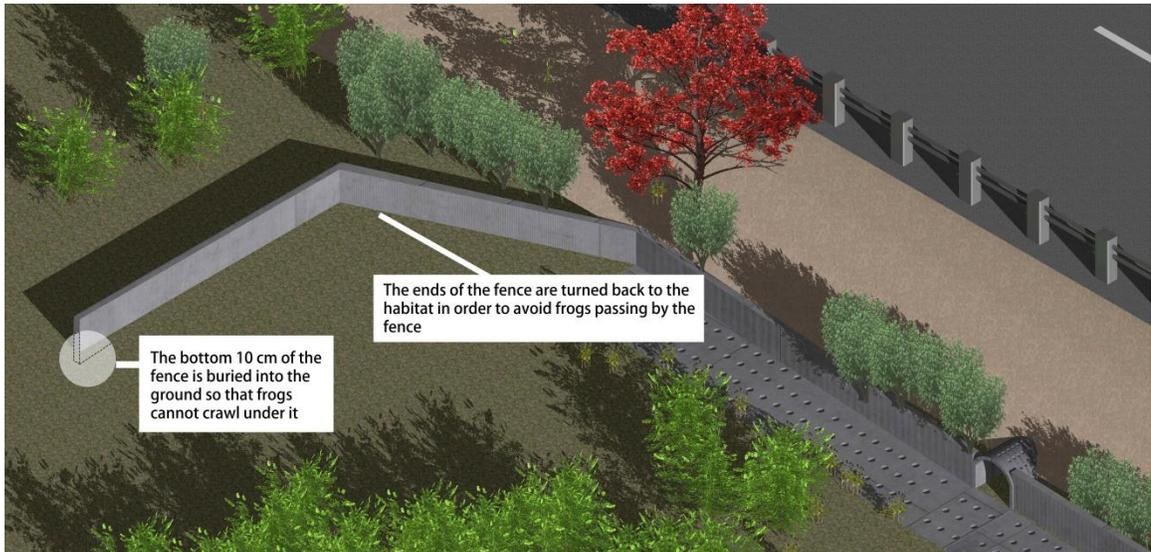
Figure 4.30: Ends of a Fence for *R. pipiens*
