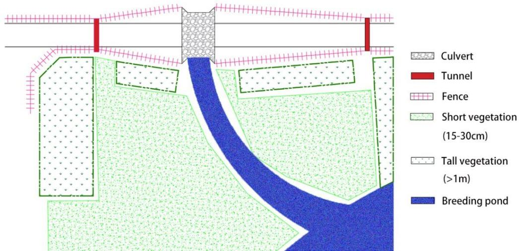
Figure 6.33: Path Network to Funnel *R. pipiens*'s Movement
