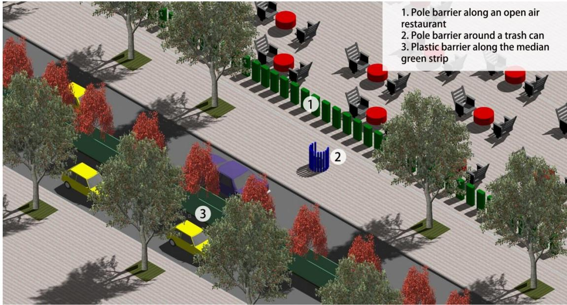
Figure 3.20: 3D View of Barriers for a Road with Open-air Restaurant, Trash Bins, and a Median Strip
