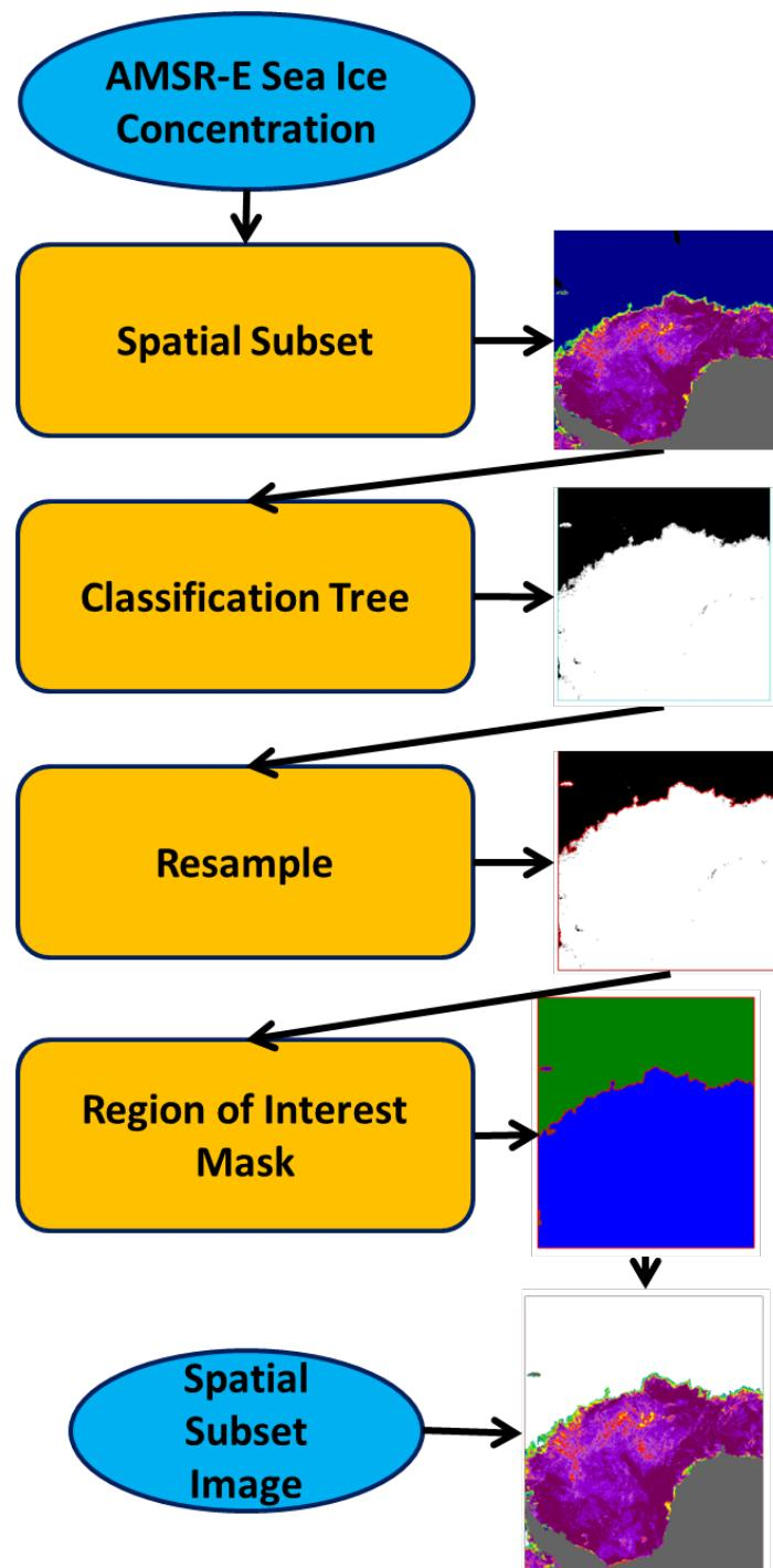
Figure 4.2 The steps to separate the ice-free area beyond the ice pack from the open water pixels within the ice pack.
