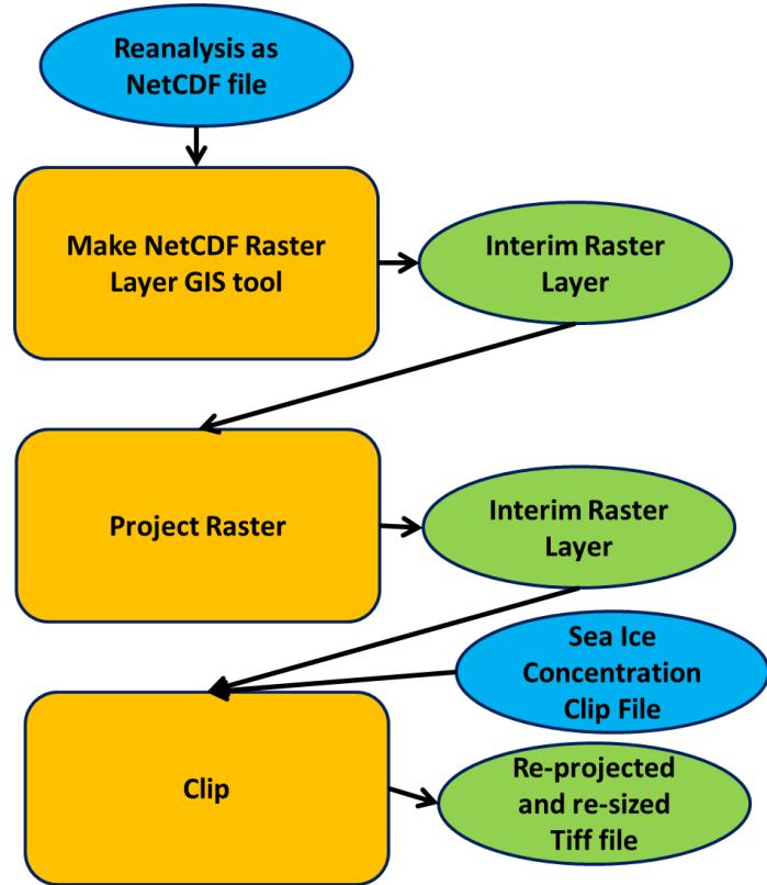
Figure 4.3 Schematic flowchart to transform NetCDF reanalysis fields to raster images in tiff file format using Python scripting and ArcGIS geoprocessing tools.
