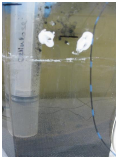
Figure 2.5: Method of supplemental nutrient solution application.
