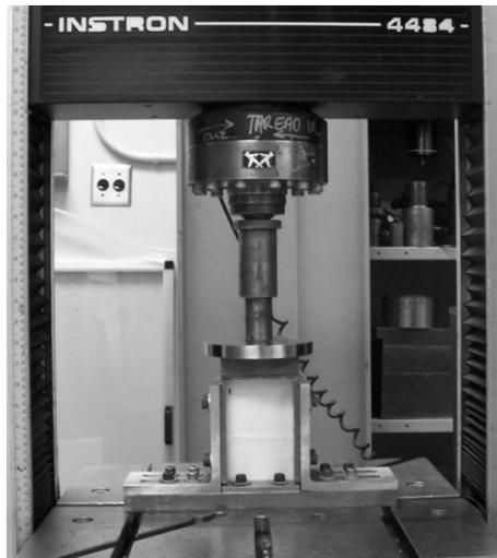
**Figure 2.13** Experimental setup for CAI testing in an Instron 4484 universal testing machine.
