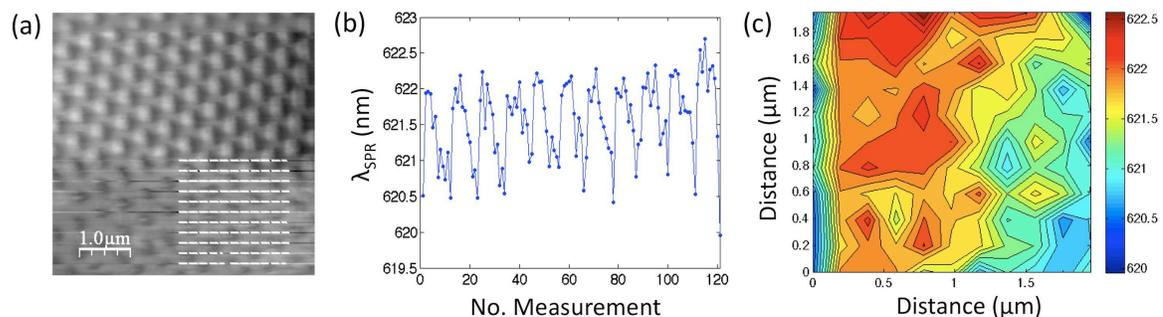
Figure 6.4: (a) AFM image acquired simultaneously with darkfield spectral acquisition where SPR measurement points within the scan are indicated by white dash marks. (b) corresponding  $\lambda_{\text{SPR}}$  at each measurement point (line added as guide) (c) SPR image of nanohole array  $\lambda_{\text{SPR}}$ (nm) (pixel spacing=195 nm).
