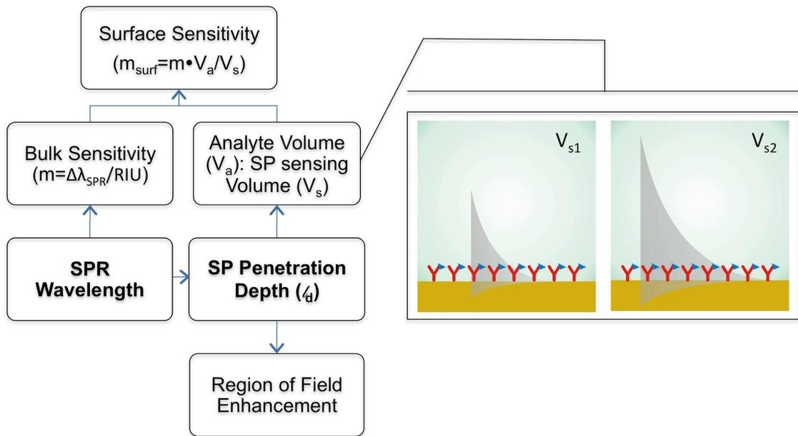
Figure 1.9: Factors affecting SPR spectroscopy surface sensitivity ( $m_{\text{surf}}$ ). The SP field diagrams depict different  $l_d$ , and thereby  $V_s$ , with the same  $V_a$ ;  $V_a/V_{s1} > V_a/V_{s2} \rightarrow m_{\text{surf}1} > m_{\text{surf}2}$
