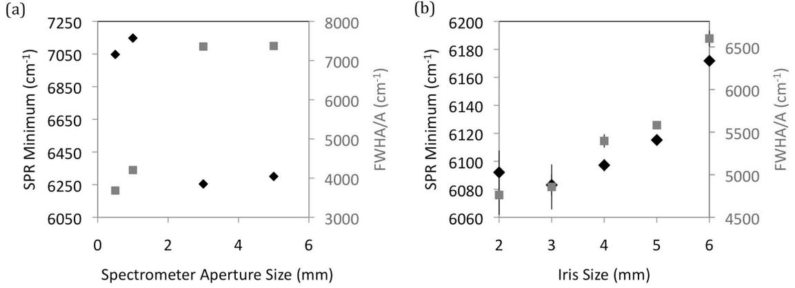
Figure 3.5: SPR minimum ( $\lambda_{\text{SPR}}$ ) ( $\blacklozenge$ ) and peak FWHM/A ( $\blacksquare$ ) for various aperture and iris size. The analysis of the aperture size is specific to the Bruker Optics Vertex 70 FTIR spectrometer.
