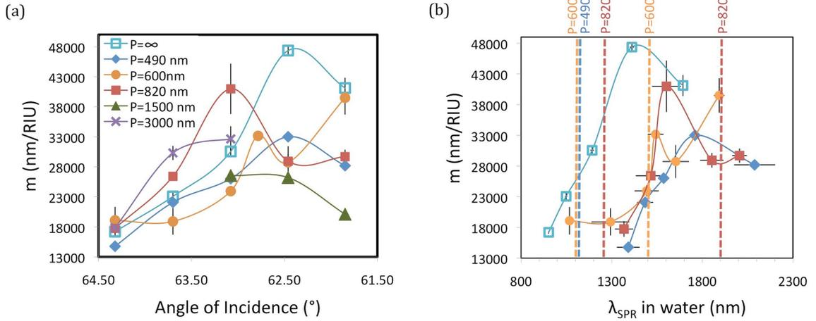
Figure 5.9: Bulk sensitivity of various periodicity ( $D/P= 0.36 \pm 0.02$ ) nanohole arrays as a function of (a) incident angle and (b)  $\lambda_{\text{SPR}}$ .  $P=\infty$  represents continuous gold. The  $\lambda_{\text{SPR}}$  of sample sensitive Bragg SPs are represented by dashed lines in (b).
