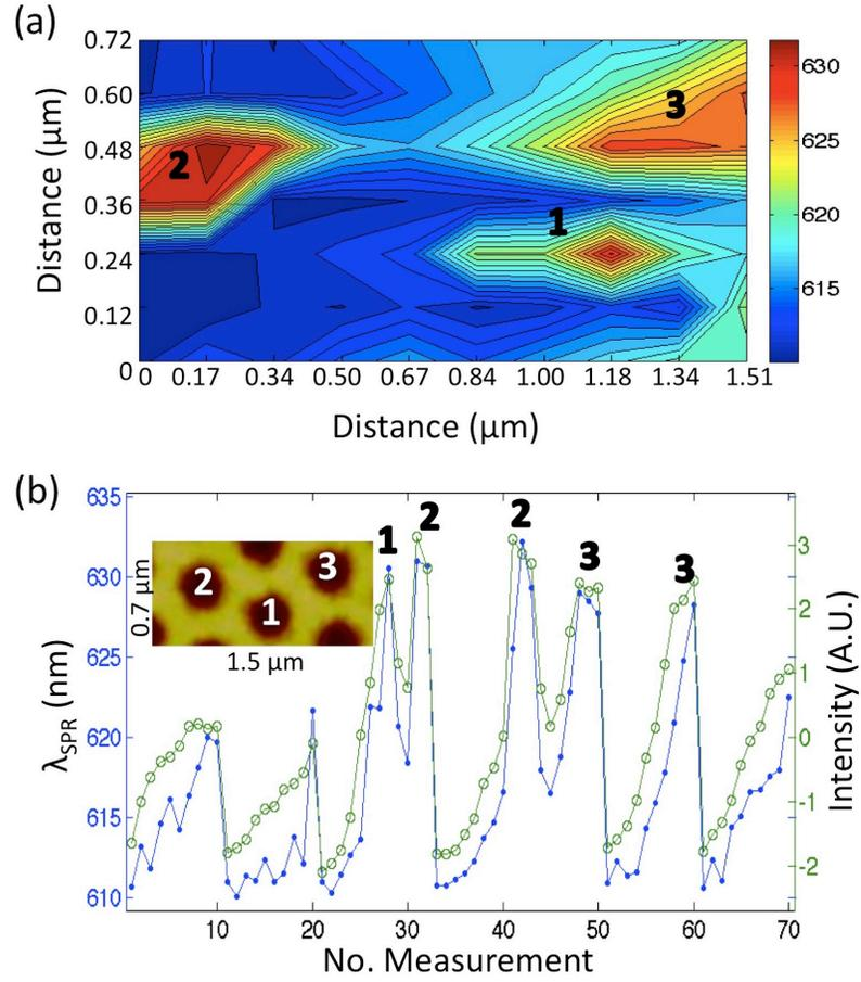
Figure 6.6:  $\lambda_{\text{SPR}}$  of stationary nanohole array with SNP positioned at various spots represented as (a) spatial image and (b) corresponding  $\lambda_{\text{SPR}}$  (blue dots) and mean centered scatter intensity (green open circles) at each measurement point (line added as guide) and inset AFM image of nanohole array outlining proposed scanned area and corresponding nanoholes with distance adjusted for hysteresis.
