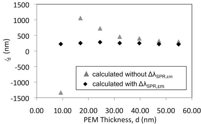
Figure 4.10: Nanohole array surface plasmon penetration depth calculated with and without  $\Delta\lambda_{\text{SPR},em}$
