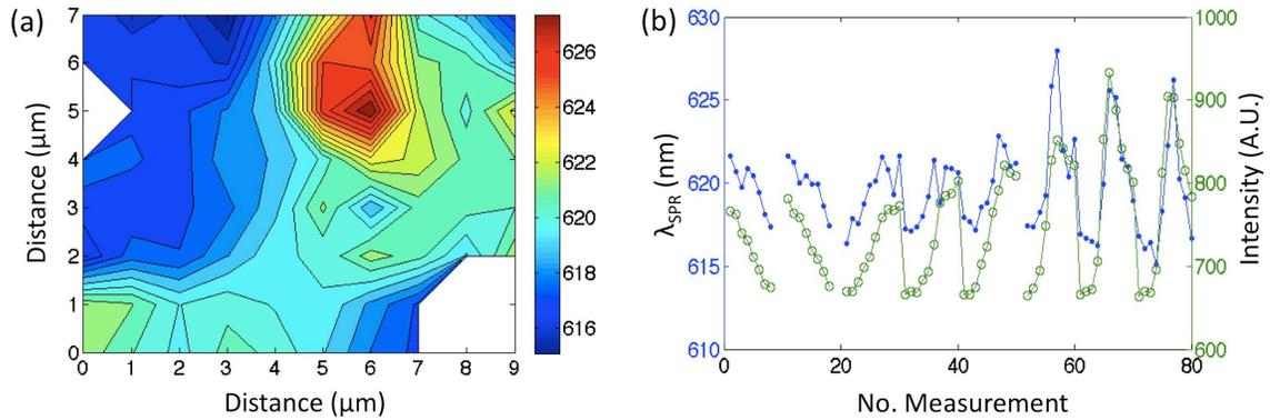
Figure 6.5:  $\lambda_{\text{SPR}}$  of stationary nanohole array with SNP probe positioned at various spots (spacing=  $1 \mu\text{m}$ ) represented as (a) spatial image where white space represents five missing data points and (b) corresponding  $\lambda_{\text{SPR}}$  (blue dots) and scatter intensity (green open circles) at each measurement point (line added as guide).
