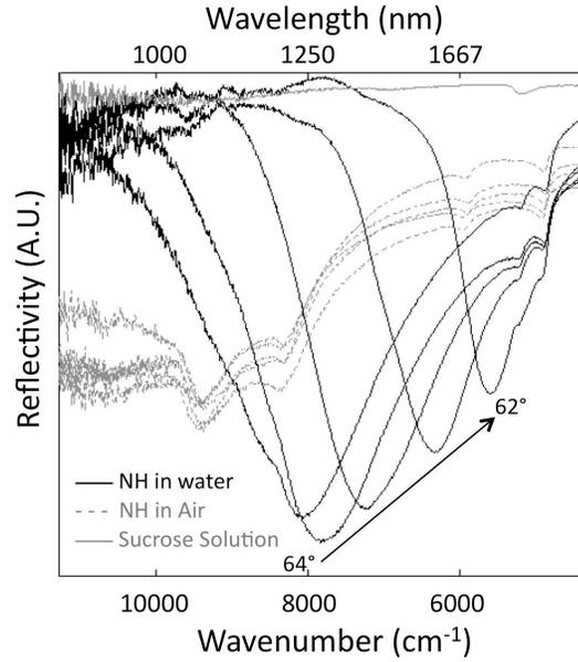
Figure 5.3: Representative nanohole array SPR spectra ( $\theta_{\text{inc}} = 64 - 62^\circ$ ) demonstrating Bragg SPs (in air) and propagating SPs (in water). A spectrum of sucrose is included to visualize potentially convoluting absorptions from the analyte.
