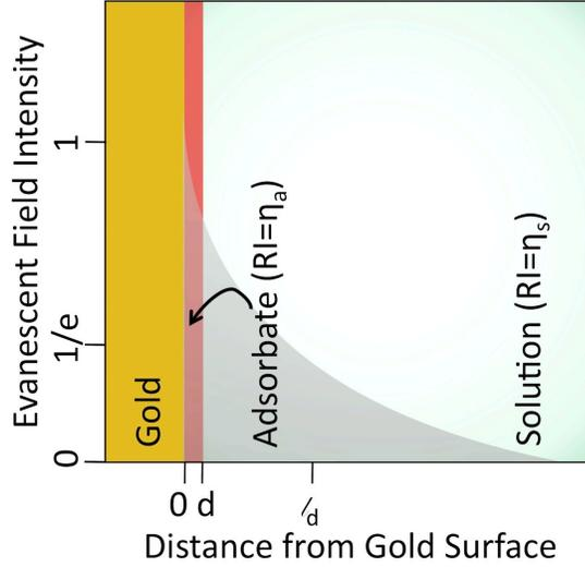
Figure 4.1: Evanescent surface plasmon with intensity decaying exponentially through bilayer of adsorbate with thickness= $d$  and bulk solution. The penetration depth,  $l_d$ , is the distance at which the relative field intensity decays to  $1/e$ .
