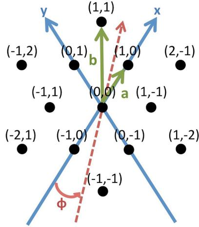
Figure 2.11: Azimuthal angle ( $\phi$ ) and different Bragg resonance orders ( $x,y$ ) displayed with respect to nanohole array reciprocal lattice. a and b represent the two different vector lengths from (0,0) included in the diagram.
