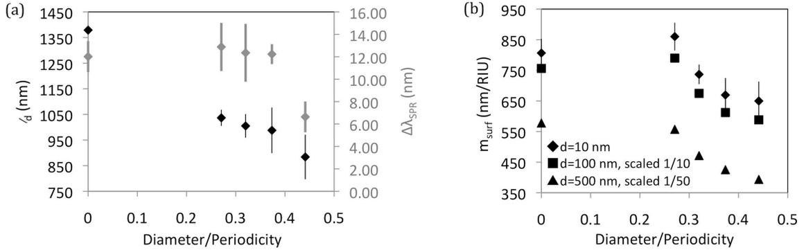
Figure 5.10: SP (a)  $l_d$ ,  $\Delta\lambda_{\text{SPR}}$  for two PEM bilayers ( $d=10$  nm), and (b) surface sensitivity of various  $D/P$  nanohole array substrates ( $P=820$  nm,  $\lambda_{\text{SPR}} = 1440$  nm).  $D/P=0$  represents continuous gold. Error bars on  $l_d$  represent standard deviation of  $l_d$  calculated from different thicknesses (1-5 bilayers). Error bars on  $\Delta\lambda_{\text{SPR}}$  and surface sensitivity represent standard deviation of triplicate measurements.
