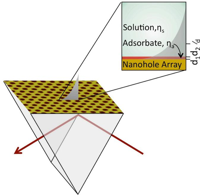
Figure 5.1: Diagram of nanohole array in Kretschmann configuration with adsorbate volume ( $d_1$  to  $d_2$ ) and sensing volume (gold interface to  $l_d$ ) illustrated. The refractive index (RI) sensed by the plasmonic field is an effective RI composed of the adsorbate RI ( $\eta_a$ ) and bulk RI ( $\eta_s$ ).
