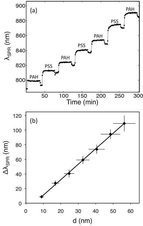
Figure 4.6: (a) Sensorgram for PEM buildup with NaCl rinse after each PEM layer. The straight line is provided as a visual aide. (b)  $\Delta\lambda_{\text{SPR}}$  with PEM thickness buildup. Vertical error bars correspond to the standard deviation in shift for  $N = 3$ . Horizontal error bars represent  $\pm s_d$ . Linear fit;  $m = 2.12 \pm 0.04$ ,  $b = \Delta\lambda_{\text{SPR},em} = -10.2 \pm 1.4$ ,  $R^2 = 0.998$ .
