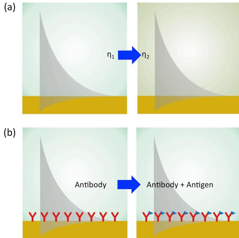
Figure 1.6: Diagram of (a) change in bulk solution refractive index ( $\eta$ ) throughout the entire SP penetration depth and (b) analyte adsorption near the surface which occupies a fraction of the SP penetration depth. The  $\Delta\lambda_{SPR}$  for given RI changes represent (a) bulk sensitivity and (b) surface sensitivity.
