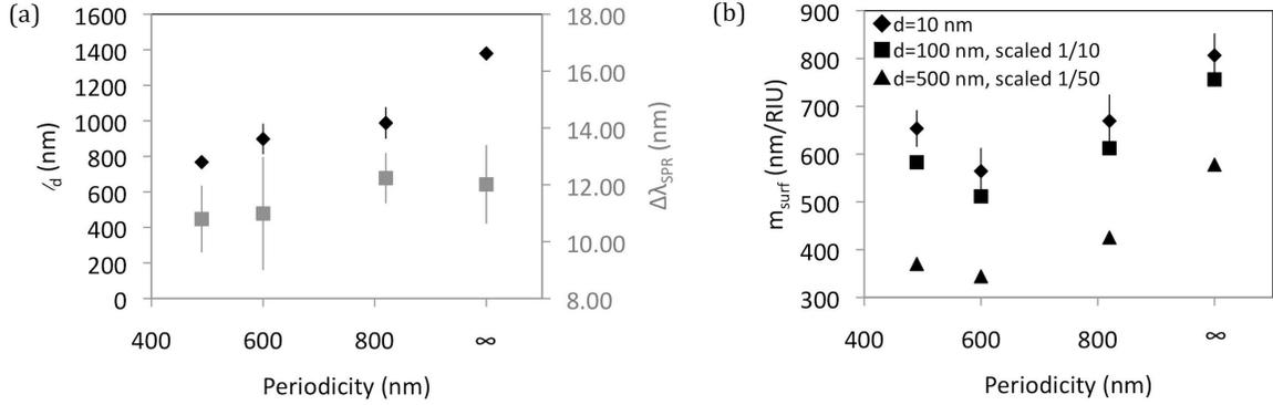
Figure 5.11: SP (a)  $l_d$ ,  $\Delta\lambda_{\text{SPR}}$  for two PEM bilayers ( $d= 10$  nm), and (b) surface sensitivity of various periodicity nanohole array substrates ( $D/P=0.36 \pm 0.2$  nm).  $P=\infty$  represents continuous gold. Error bars on  $l_d$  represent standard deviation of  $l_d$  calculated from different thicknesses (1-5 bilayers). Error bars on  $\Delta\lambda_{\text{SPR}}$  and surface sensitivity represent standard deviation of triplicate measurements
