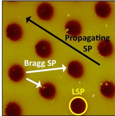
Figure 2.2: Diagram of nanohole array SP modes.
