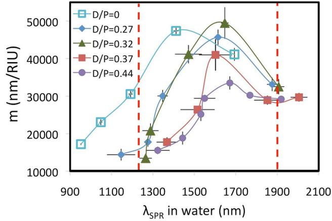
Figure 5.8: Bulk sensitivity of various diameter nanohole arrays ( $P=820$  nm) as a function of  $\lambda_{\text{SPR}}$ .  $D/P=0$  nm represents continuous gold. The  $\lambda_{\text{SPR}}$  of the sample sensitive Bragg SPs are represented by red dashed lines.
