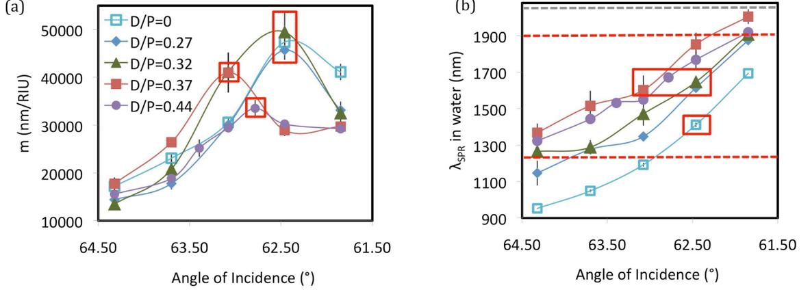
Figure 5.7: (a) Bulk sensitivity and (b)  $\lambda_{\text{SPR}}$  of various diameter nanohole arrays ( $P=820$  nm) as a function of incident angle.  $D/P=0$  nm represents continuous gold. The points of maximum bulk sensitivity for each sample are outlined and the  $\lambda_{\text{SPR}}$  of the Bragg SPs are represented by dashed lines.
