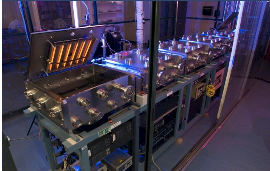
**Figure 3-2 Six Chamber in-line PECVD system at IEC**
