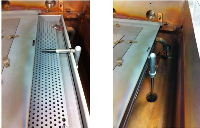
**Figure 2-11 Hiden Analytical Langmuir Probe installed in PECVD chamber at IEC**
