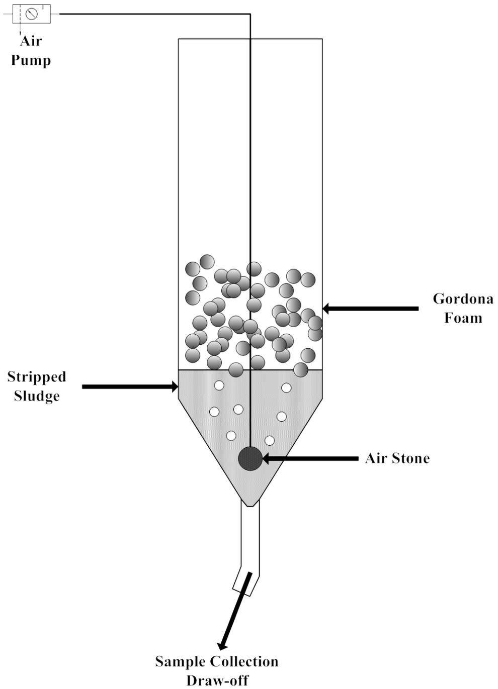
**Figure 3.1** Diagram of air stripping procedure
