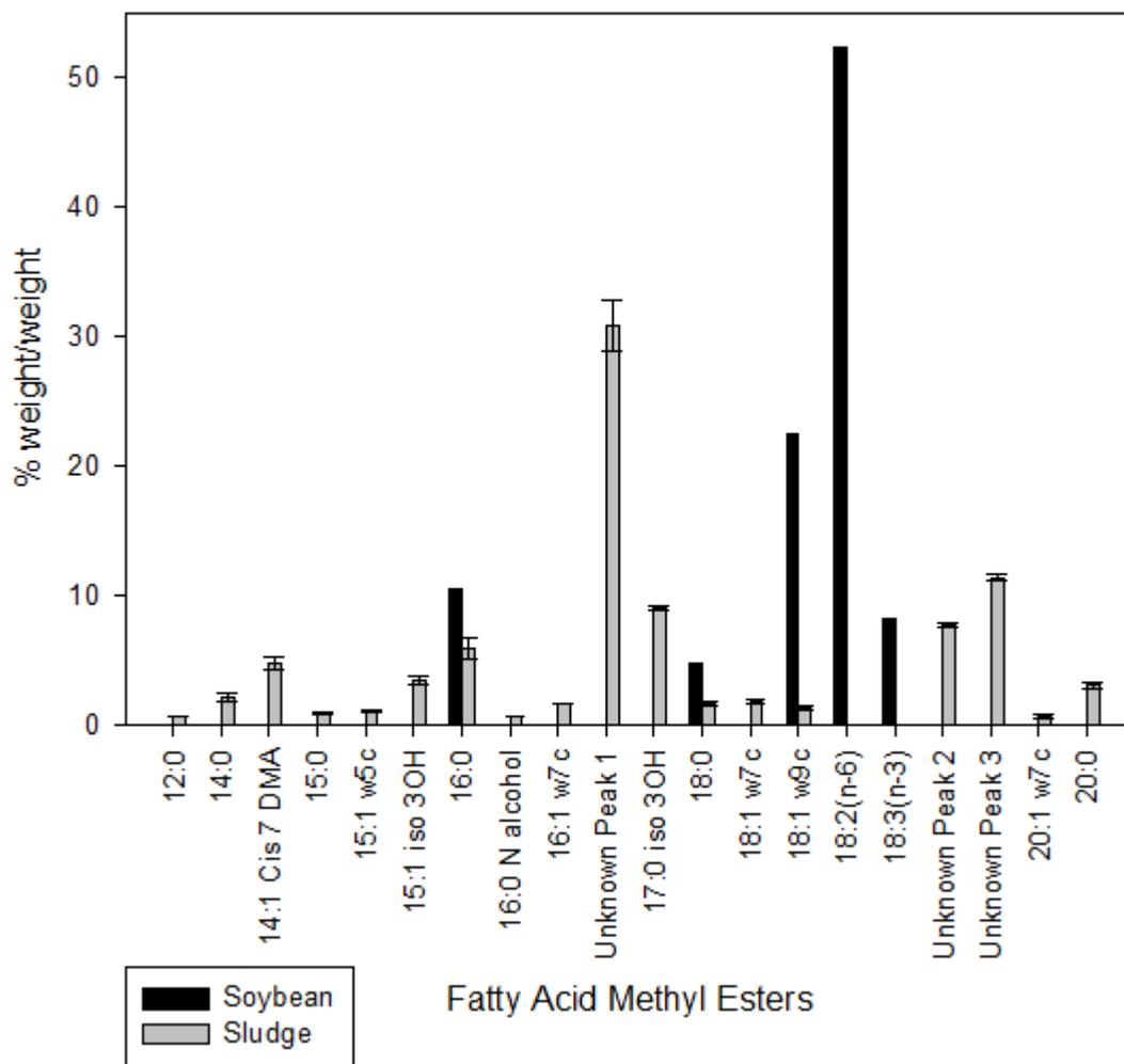
**Figure 4.6** FAME profiles for sludge biodiesel samples as compared to soybean biodiesel samples (Canakci and Van Gerpen, 2003; Lotero et al., 2005).
