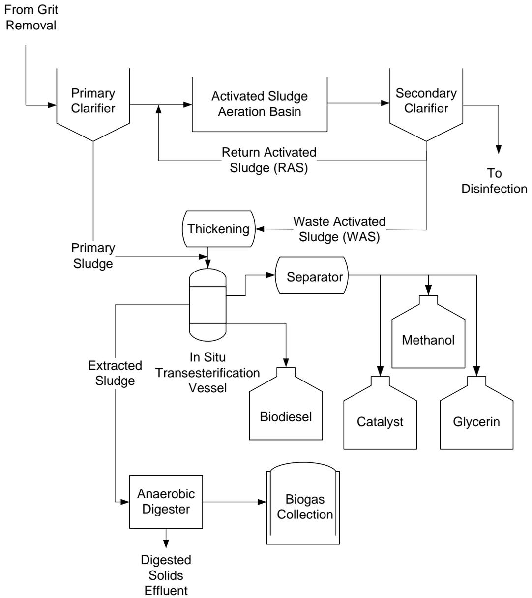
**Figure 5.1 Integrated biodiesel and wastewater treatment process**
