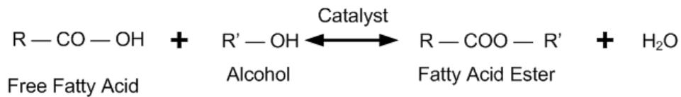
**Figure 2.1** The transesterification reaction. Triglycerides (top) and free fatty acids (bottom) are being converted to fatty acid esters. Adapted from Carrapiso and Garcia (2000) and Marchetti et al. (2006).
