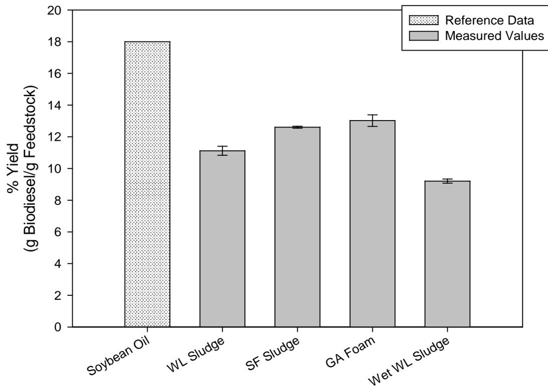
**Figure 4.2** Biodiesel yields for different sludges as compared to yields for soybean oil (Freedman et al., 1984; USDA, 2008). The bar data signify the average of duplicate samples and the error bars correspond to the standard deviation.
