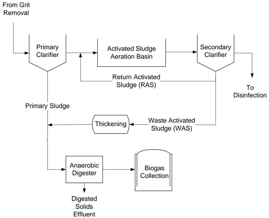
**Figure 2.3 Primary and secondary treatment in a municipal wastewater treatment plant. Adapted from Tchobanoglous and Schroeder (1985) and Metcalf & Eddy (1991).**
