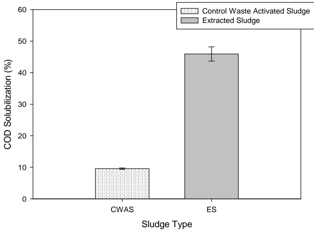
**Figure 4.8** Percent COD solubilization in different sludges. The bar data signify the average of duplicate samples and the error bars correspond to the standard deviation.
