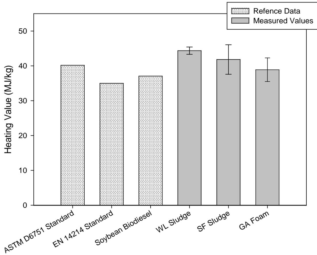
**Figure 4.3 Biodiesel heating values for different sludge biodiesel samples as compared to soybean diesel and biodiesel standard values (Knothe et al., 2005; EN, 2008; NREL, 2009; ASTM, 2010). The bar data signify the average of duplicate samples and the error bars correspond to the standard deviation.**
