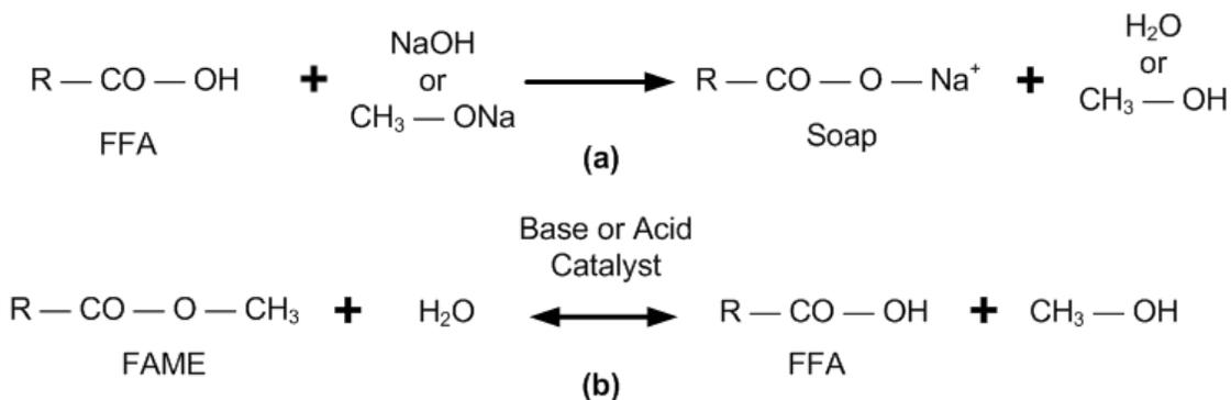
**Figure 2.2** Formation of soap due to the interaction of FFA and sodium hydroxide (a) and hydrolysis of FAMES by water (b). Adapted from Lotero et al. (2005).
