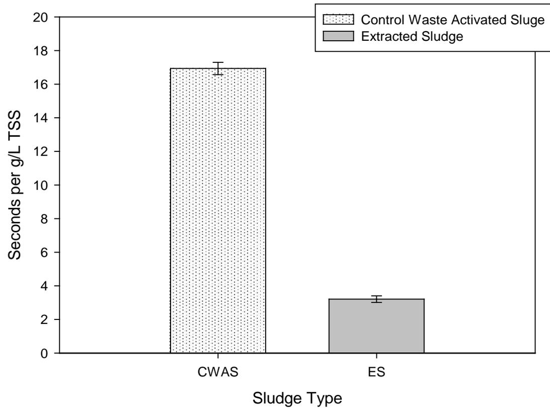
**Figure 4.7** Dewaterability of sludges with and without pretreatment. The bar data signify the average of duplicate samples and the error bars correspond to the standard deviation
