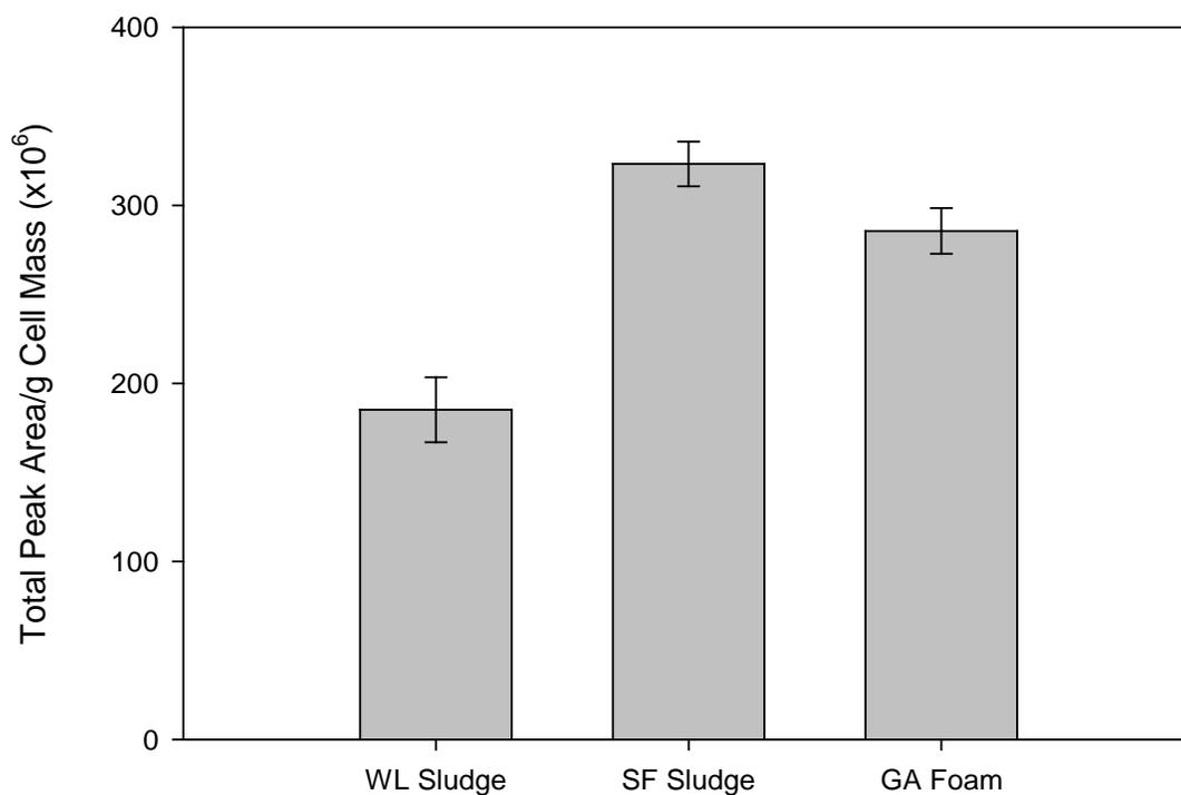
**Figure 4.1** Relative amounts of fatty acids for different sludge samples normalized by the cell mass. The bar data signify the average of duplicate samples and the error bars correspond to the standard deviation.
