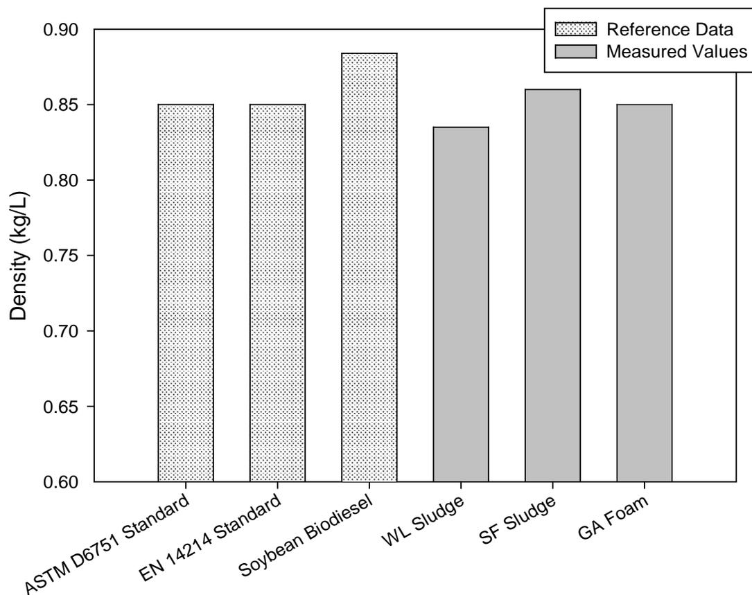
**Figure 4.4** Biodiesel density values for different sludge biodiesel samples as compared to soybean diesel and biodiesel standard values (Knothe et al., 2005; EN, 2008; NREL, 2009; ASTM, 2010).
