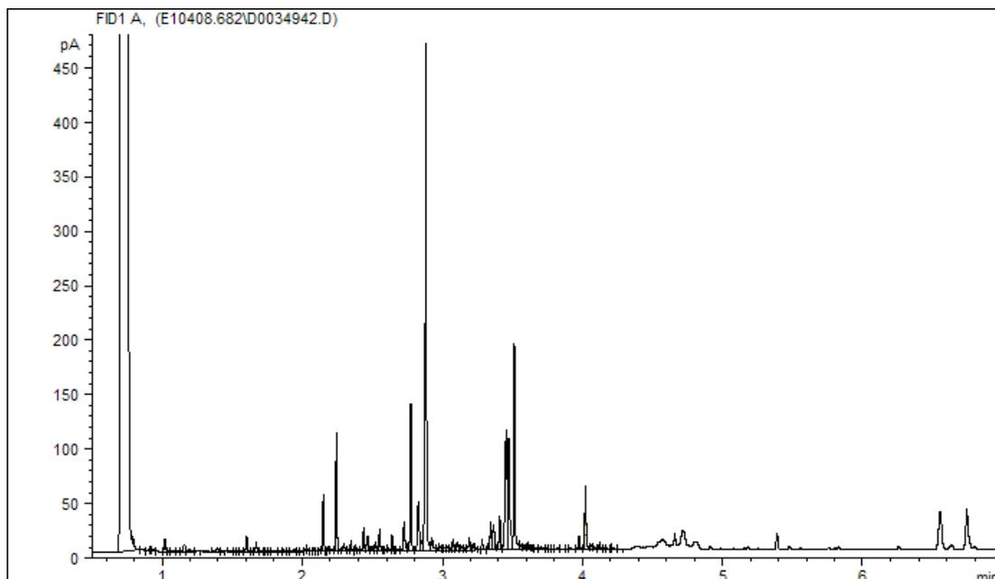
**Figure 4.5** Gas chromatograph of a sludge biodiesel sample.
