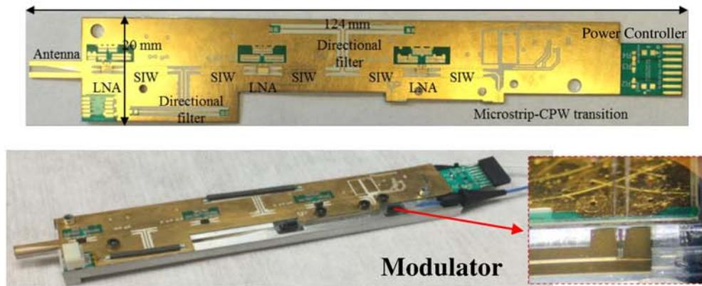
Figure 7-4: Detailed LCP module (top) and a packaged RF front-end module with integrated modulator (bottom)
