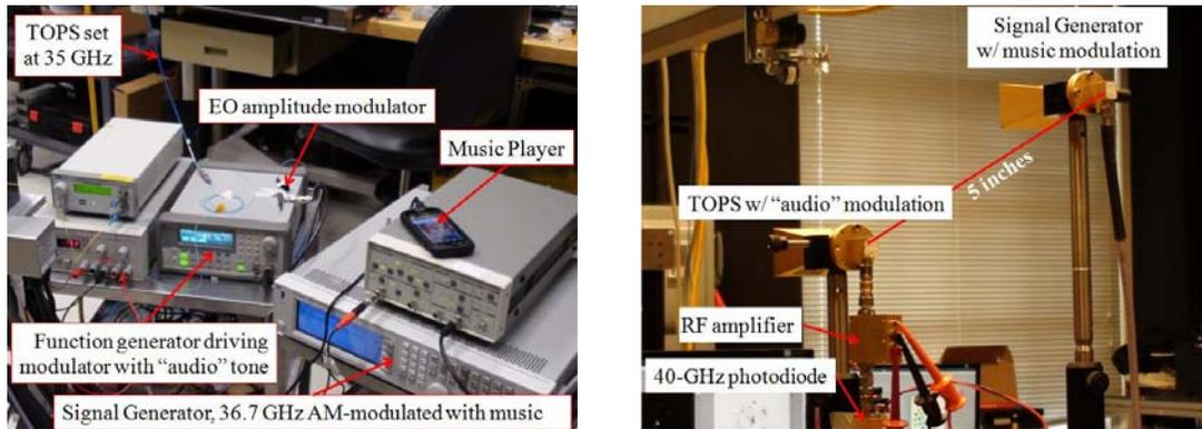
Figure 6-2: Equipment setup to generate two RF tones with AM transmitted data (left) and antenna setup for both sources with labeled spatial separation (right)
