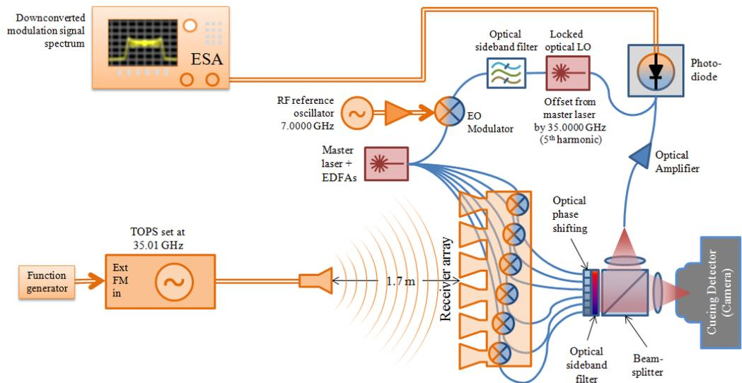
Figure 6-4: Photonic downconversion demonstration setup with an FM audio tone transmitting at 35.01 GHz RF carrier and mixed on a photodiode with the optical LO to an IF of 10 MHz
