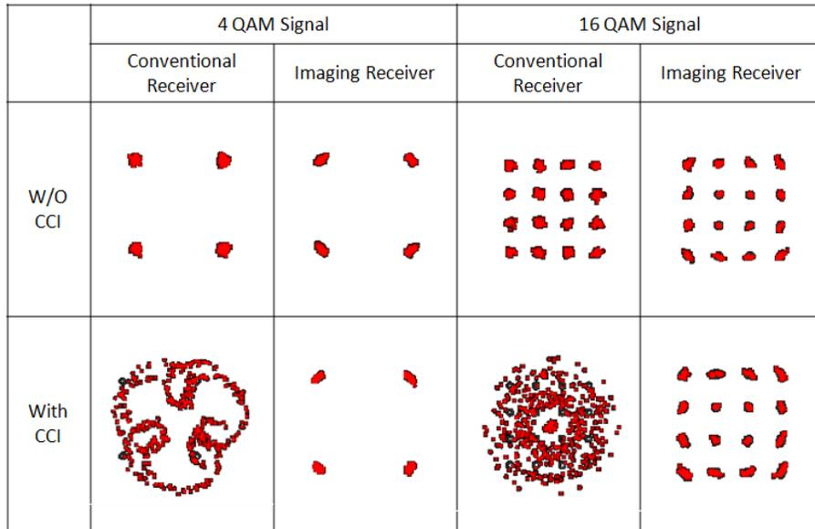
Figure 6-11: 4 QAM and 16 QAM at 50 Msps symbol rate with and without the presence of a second CCI transmitter
