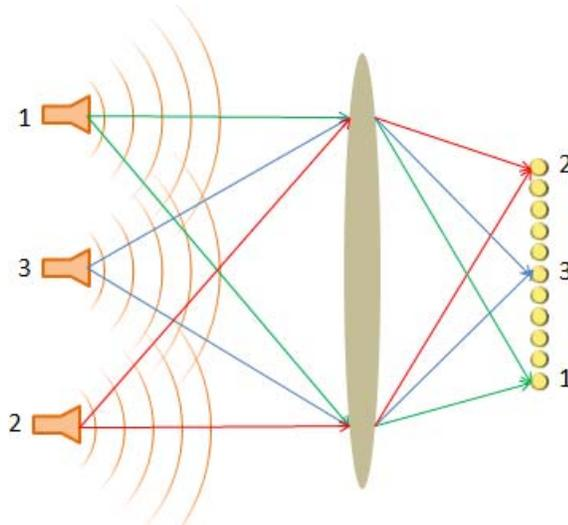
Figure 1-2: Spatial mapping of signals after arriving at a receiver from different angles onto separate locations of the receiver plane detector
