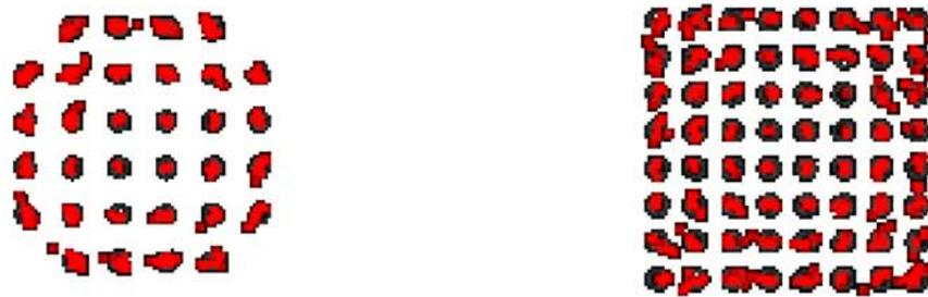
Figure 6-9: Demodulated 32 QAM (left) and 64 QAM (right) recovered through the imaging receiver at 50 Msps symbol rate
