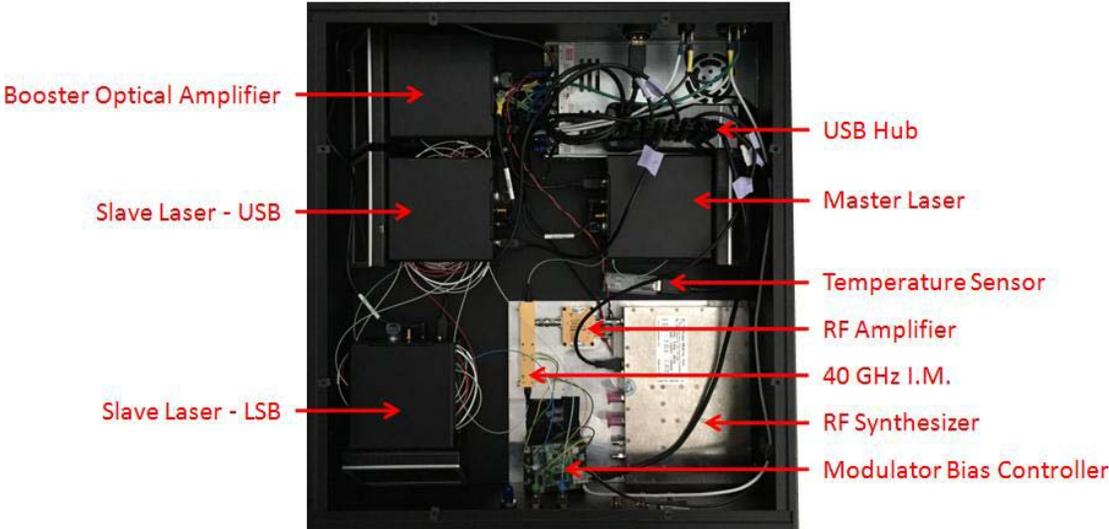
Figure 3-7: TOPS design with labeled components
