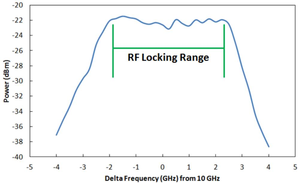
Figure 3-3: RF locking range of the TOPS offset from 10 GHz
