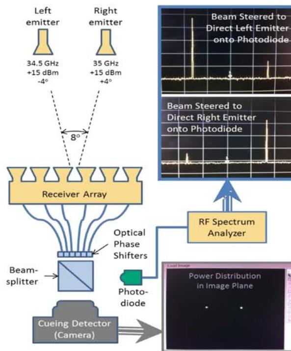
Figure 4-3: Illustration of preliminary demonstration of spatial multiplexing discrimination by the proposed receiver configuration
