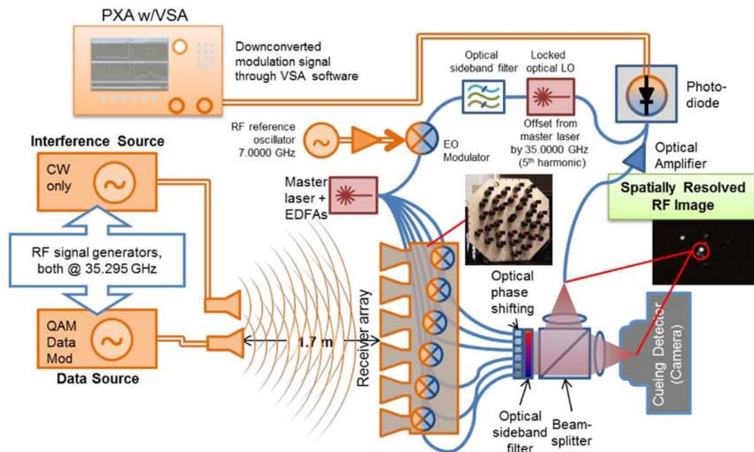
Figure 6-6: Photonic downconversion demonstration of communications signal recovery in the presence of co-channel interference
