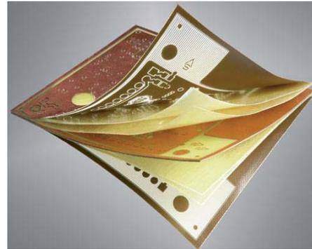
Figure 7-3: Conductive layers all interconnected to each other through coupling structures (left) [43] and the LCP material (right) [44]
