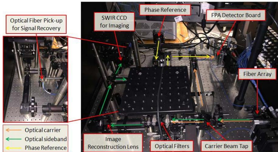
Figure 2-8: Optical processor of receiver including fiber pickup for signal recovery
