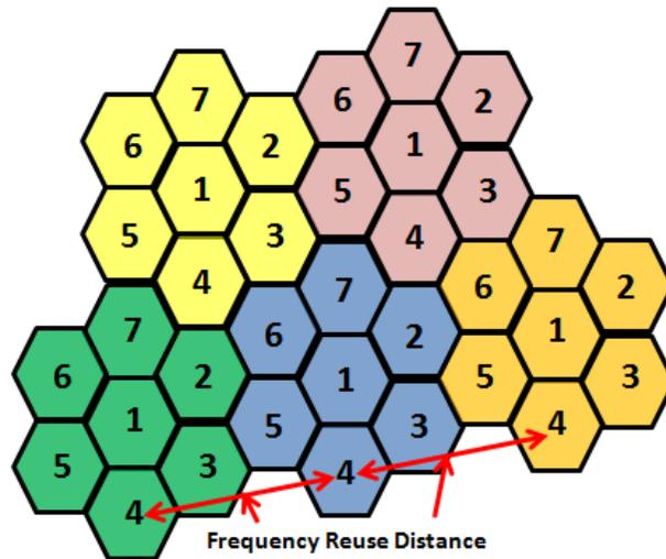
Figure 1-3: Frequency Reuse through cell staggering [10]
