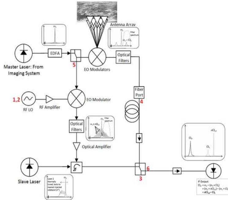
Figure 5-1: Schematic of optical LO used within receiver architecture
