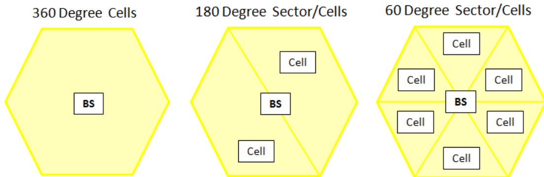
Figure 1-5: Cell Sectorization Method using multiple directional antennas [14]
