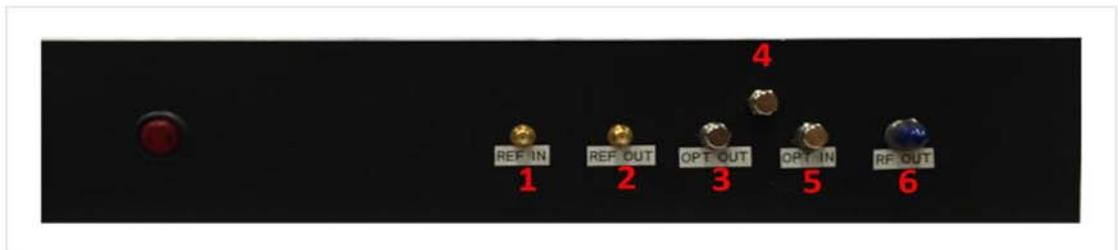
Figure 5-2: Front panel display of RF and optical adapters for connectivity to imaging receiver
