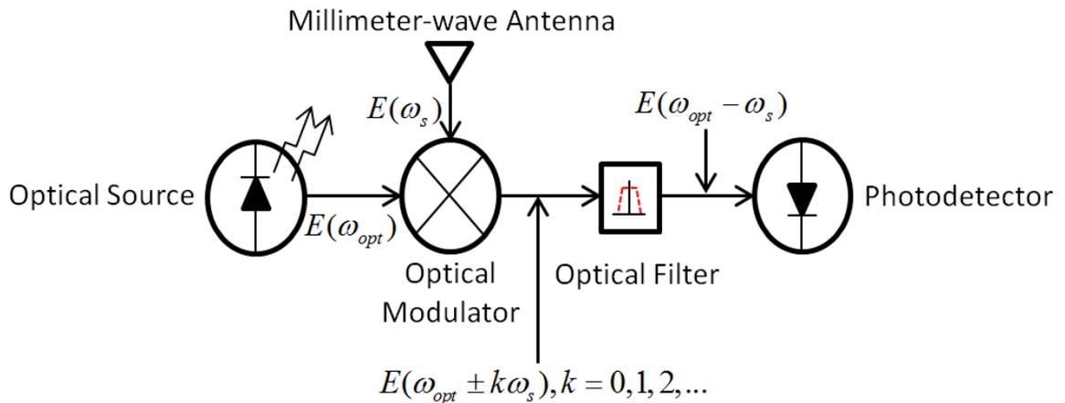
Figure 2-1: Conceptual RF Photonic Link of Communication Receiver
