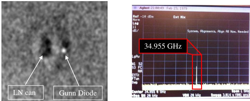
Figure 4-1: Image from 35 GHz passive millimeter-wave imaging system showing both passive and active field of views from three meters away (left) and the mechanically tuned Gunn diode detected on an RF spectrum analyzer (right) [20]
