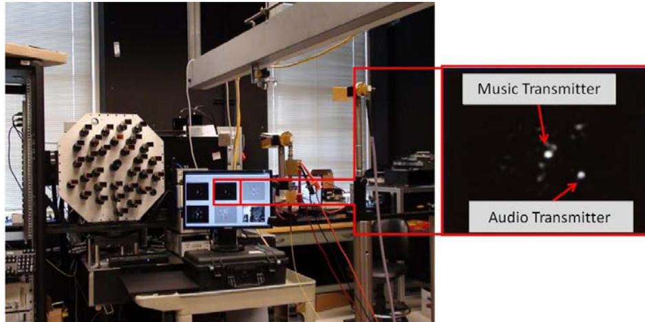
Figure 6-3: Two tone receiver setup with the imaging receiver beam steered toward the music transmitter (left) and the cueing detector image of the two sources with the music transmitter centered on the image (right)
