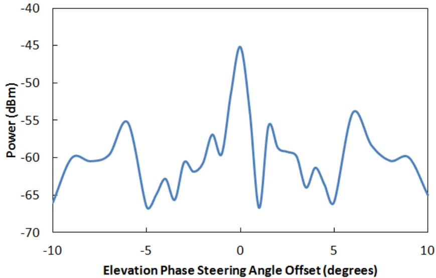
Figure 4-5: Power detection through phase steering in Elevation direction
