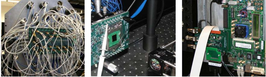
Figure 2-4: LNA power and phase control board attached to antenna array (left), FPA receiver board for phase control (middle), and FPGA for system control (right) [17]
