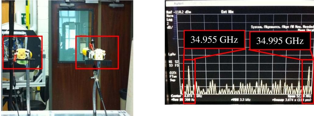
Figure 4-2: Image of two sources (left) and the received RF Spectrum (right) [20]
