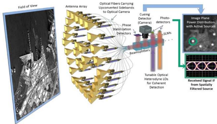
Figure 2-7: Illustration of the ability of the proposed communication receiver architecture. Spatially isolated RF sources are separately tracked and detected in the image plane and routed for IF detection
