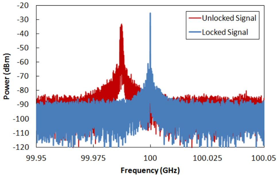
Figure 3-4: Comparison of locked and unlocked RF at 100 GHz by turning off master laser into the modulator
