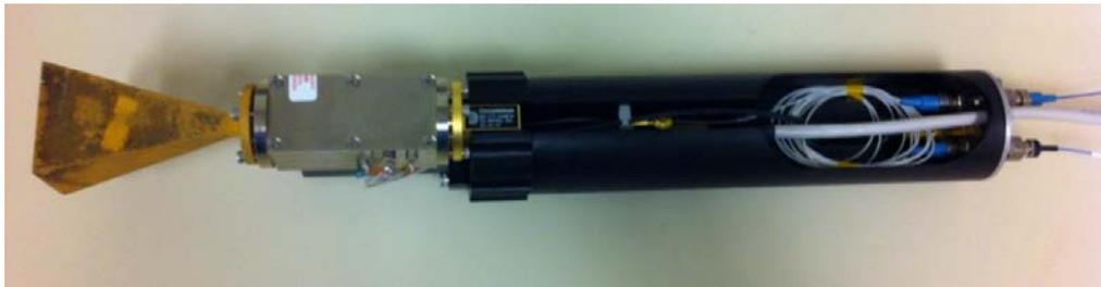
Figure 7-2: RF Front-End Module in current communication receiver
