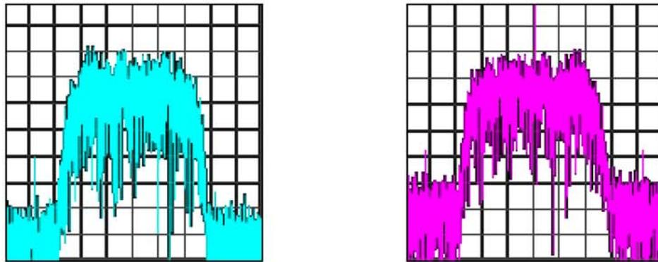
Figure 6-10: Downconverted IF spectrum with CCI suppression through communication receiver (left) and co-channel carrier spectrum interference through a conventional free space antenna (right)
