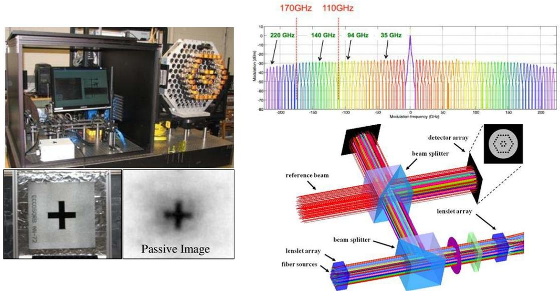
Figure 2-3: Experimentally tested and demonstrated optically addressed receiver capable of passive radiometric imagery (left), broadband optical modulators capable of E/O conversion up to 300 GHz (top right), and optical phase control system for given receiver architecture (bottom right)
