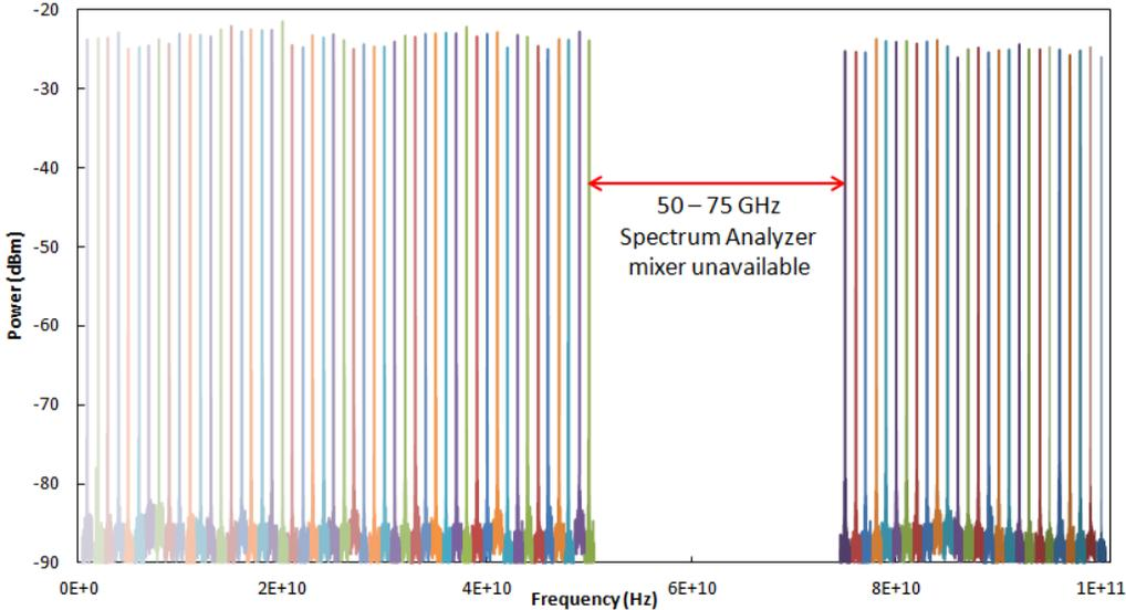
Figure 3-8: RF spectrum of generated RF from 1 to 100 GHz using TOPS
