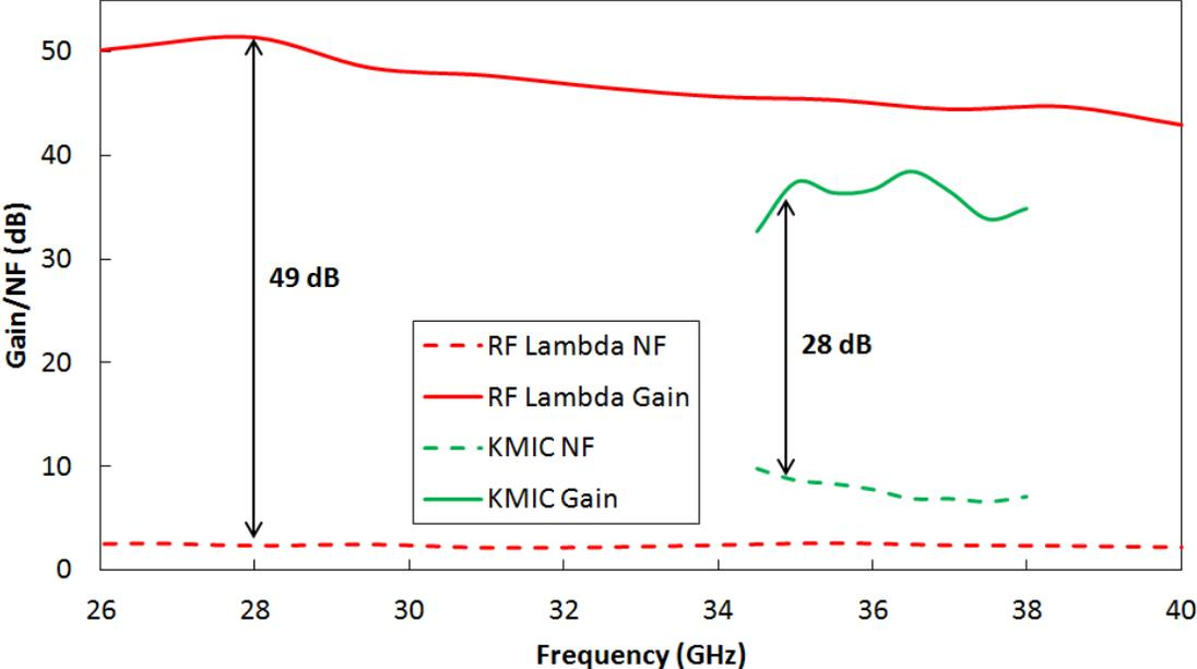
Figure 7-1: Amplifier comparison of current KMIC amplifier to improved RF Lambda amplifier for bandwidth coverage and better gain and NF characteristics
