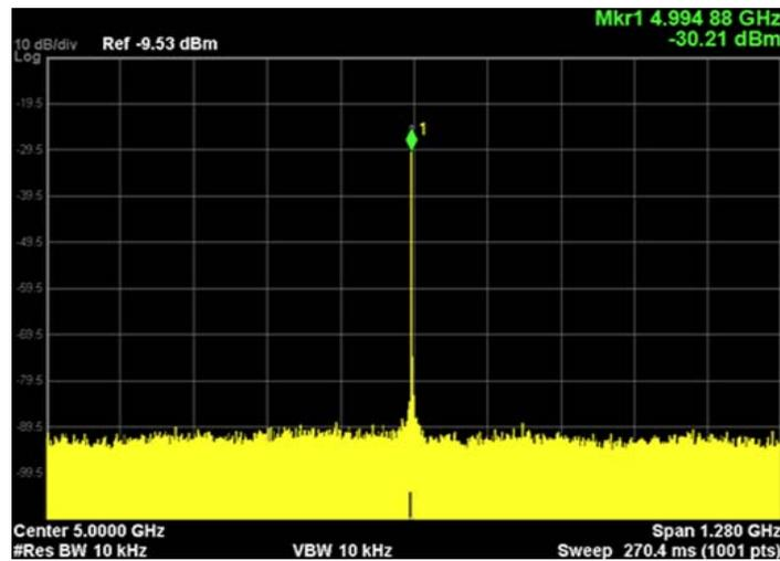
Figure 5-4: Downconverted RF from 35 GHz to 5 GHz using an optical LO
