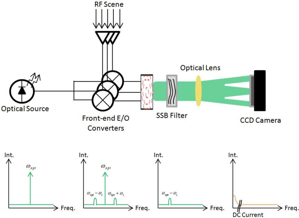
Figure 2-2: Schematic of RF to optical free space for spatial imaging (top) and optical spectrum through E/O conversion and photodetection
