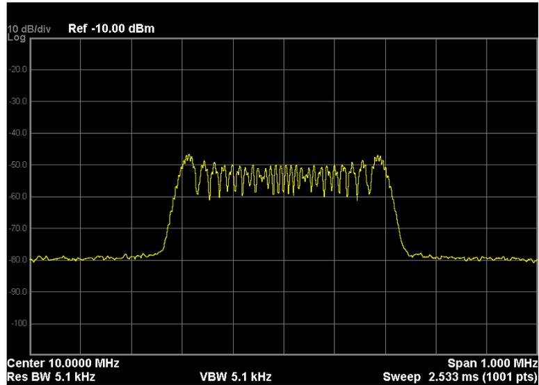
Figure 6-5: Recovered signal at a 10 MHz IF on an RF spectrum analyzer illustrating the signals IBW
