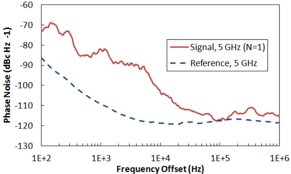
Figure 3-5: Phase noise comparison of RF synthesizer and TOPS output
