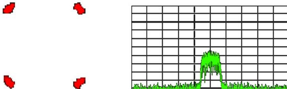
Figure 6-7: Preliminary 4 QAM demodulated signal with 1 Msps symbol rate (left) and corresponding RF spectrum illustrating the signal bandwidth (right)
