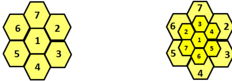
Figure 1-4: Typical cell cluster (left) and cell splitting process (right) [12]
