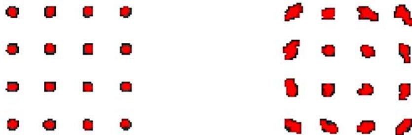
Figure 6-8: Illustration of path matched RF with no associated phase noise (left) and inherent phase noise contribution from communication receiver due to optical fiber path mismatch (right)
