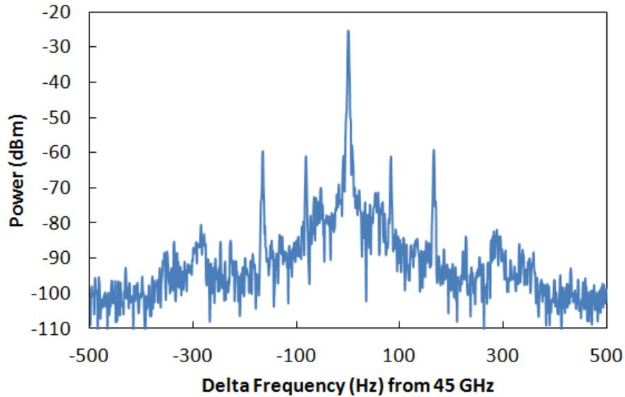
Figure 3-6: Linewidth of RF signal at 45 GHz
