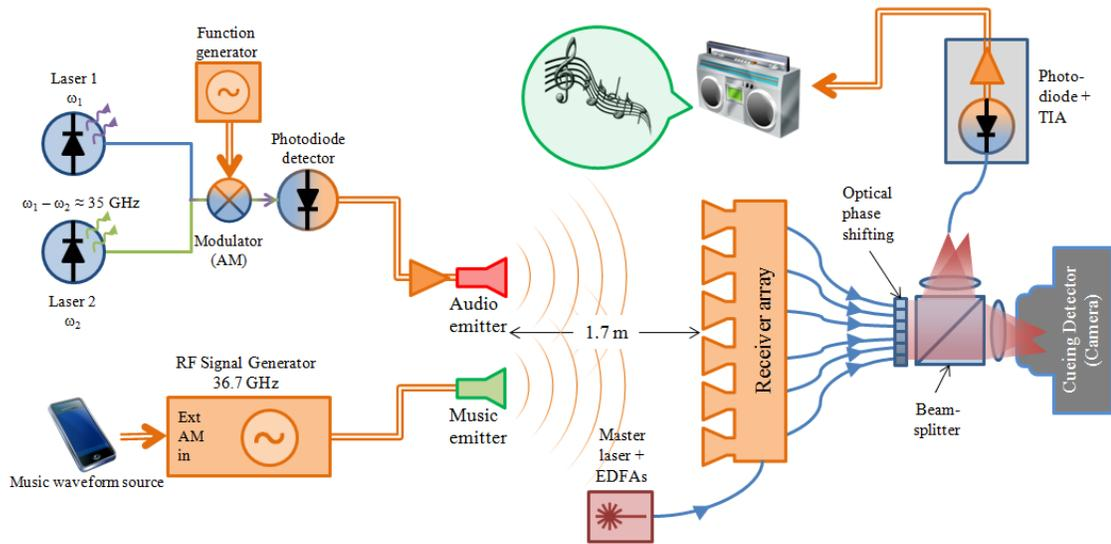
Figure 6-1: Photonic demonstration setup for spatially isolated AM recovery and detection using TOPS as an audio transmitter
