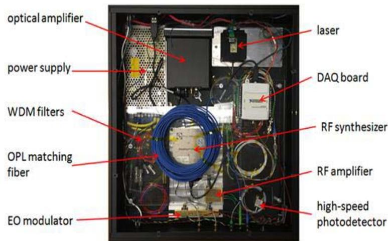
Figure 5-3: Top view of optical LO with labeled components
