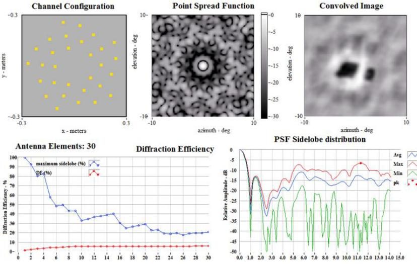
Figure 2-5: Channel configuration of the antenna array (top left), corresponding PSF of the array (top middle), and passive image of cars set at 50 meters from the receiver (top right). The sidelobe levels at radial offsets from the center of the PSF (bottom right) and diffraction efficiency as a function of the number of elements in the array (bottom left)
