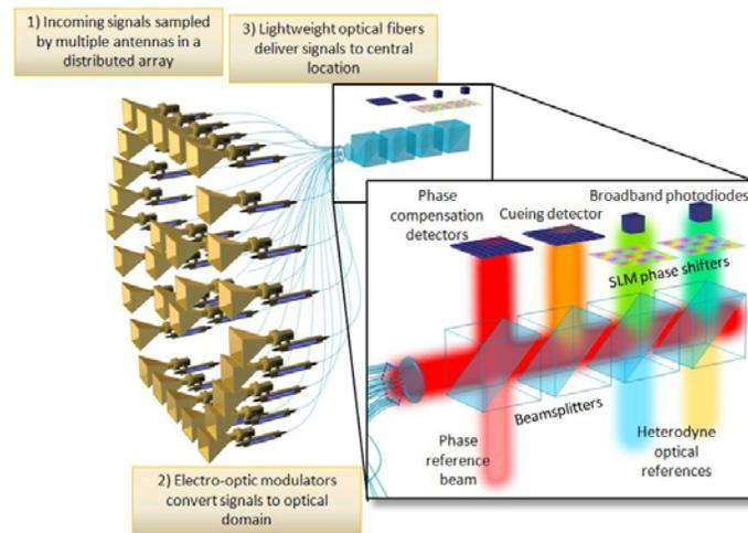
Figure 2-6: RF receiver concept to receive RF, upconvert RF onto an optical carrier, and route and process the signals via a back-end optical processor for temporal and spectral analysis.
