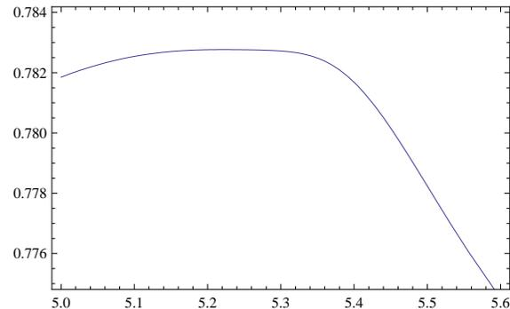
(b) The terminal cost, expressed by the value of the navigation function, temporarily increases along the probable near optimal trajectory, consistently with the requirements of Proposition 1. This brief increase may be a result of a sample input that yielded significantly better performance compared to other candidate solutions in the sample set.
