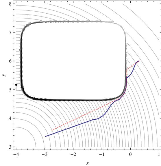
(a) The solid curve represents the path produced by the randomized receding horizon scheme, while the dashed curve shows the path corresponding to steepest descent. Note how the receding horizon path curves to the bottom-left to reduce the communication shadowing effect from the obstacle.
