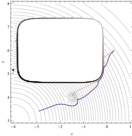
(a) Oops! pitfall. In this simulation run of four steps, there is a local minimum at which the steepest descent solution shown with the dashed curve gets trapped. The randomized receding horizon solution circumvents the minimum and continues toward the goal, bending to the right trying to simultaneously decrease the shadowing effect of the obstacle.
