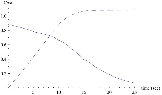
(b) Terminal and incremental cost evolution along the randomized receding horizon path of Fig. 7(a). At the beginning of the fourth simulation step, the algorithm decides to increase the terminal cost temporarily, so that the local minimum is circumvented.
