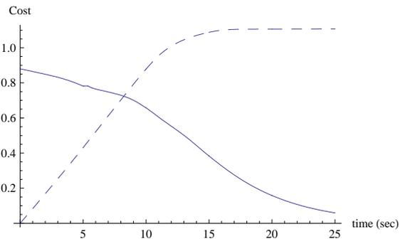
(a) Evolution of terminal cost (shown in solid curve) and incremental cost (shown in dashed curve) along a solution of the receding horizon scheme over time. The simulation period covers five steps, each with a control horizon of five seconds. Note the brief increase on the terminal cost close to the fifth simulation second, shown in detail in Fig. 6(b)
