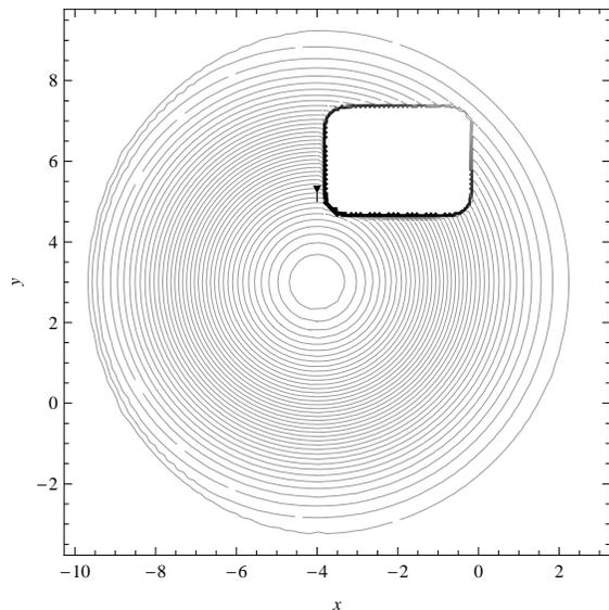
(a) Contour plot of the navigation function on a spherical workspace with a rectangular obstacle. The destination configuration is slightly off-center. The position of the radio base station is marked close to the bottom left hand corner of the obstacle.
