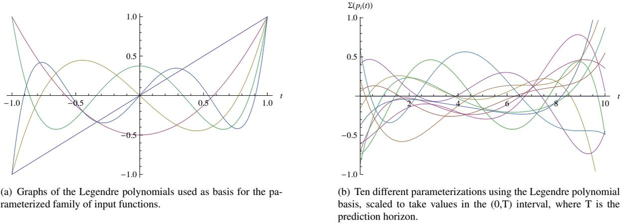
Figure 3: A Legendre polynomial basis is chosen to parameterize the control inputs. Each input candidate is a perturbation over the (nominal) direction of the potential field as indicated in (15).
