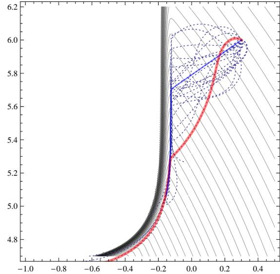
(b) An example of candidate paths resulting from different input samples. Different paths are shown in dashed curves. The steepest descent path is shown with the solid curve and for the prediction horizon selected, terminates close to  $(-0.175, 5.1)$ . The probable near optimal one is highlighted with the thick solid line, and continues beyond the selected frame.
