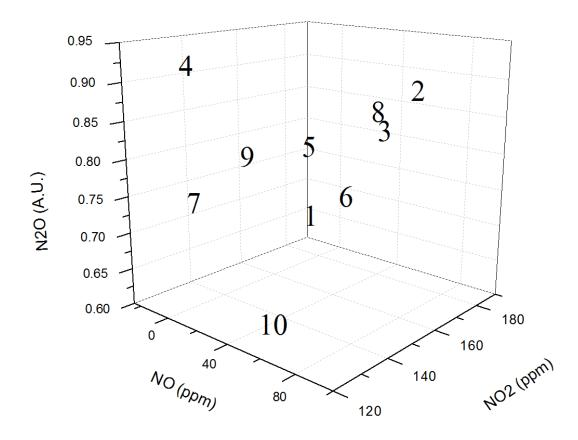
Figure 28 A 3-dimensional plot of the RuCoBa catalysts displaying the NO, NO $_2$ , and N $_2$ O concentrations at 300 $^\circ$ C with the addition of a 5Co15Ba catalyst represented as #10
