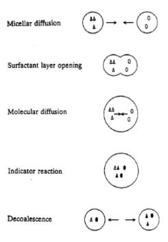
Figure 4 A schematic of the five elementary steps associated with reverse micellar coalescence, solubilizate exchange, reaction and decoalescence.
