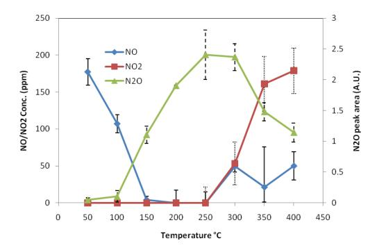
Figure 12 High-Throughput SCR data for Pt-B catalyst
