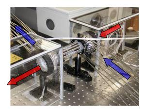
Figure 6 Photograph of the GPA. The red arrows indicate the direction of the IR beam while the blue arrows indicated the flow of effluent gases from the catalyst beds (reproduced from [17]).
