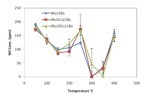
Figure 22 High-throughput data of NO concentration for the 4Ru15Ba, 4Ru5Co15Ba, and 4Ru10Co15Ba catalysts
