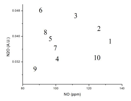
Figure 29 A 2-dimensional plot of the RuCoBa catalysts displaying the NO and  $N_2O$  concentrations at  $150^{\circ}C$  with the addition of a 5Co15Ba catalyst represented as #10.
