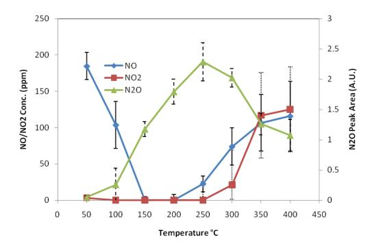
Figure 10 High-Throughput SCR data for Pt-X catalyst
