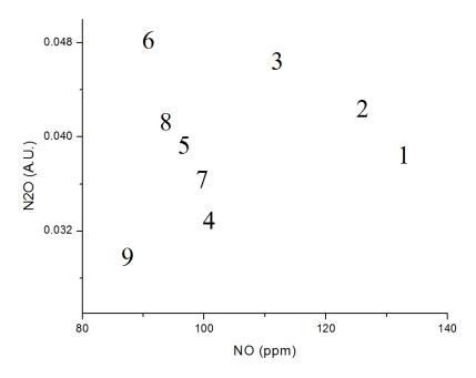
Figure 26 A 2-dimensional plot of the RuCoBa catalysts displaying the NO and  $N_2O$  concentrations at  $150^{\circ}C$
