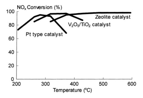
Figure 2 General NO<sub>x</sub> conversion trend of different SCR catalytic technologies (reproduced from [12]).
