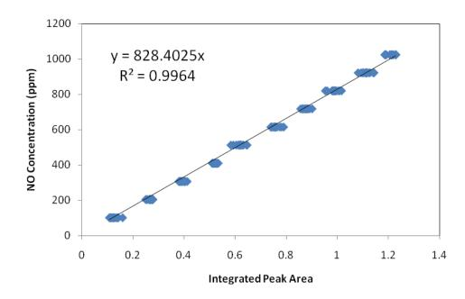
Figure 7 NO Calibration. The peak area of NO was integrated from 1975 to 1800 cm<sup>-1</sup>
