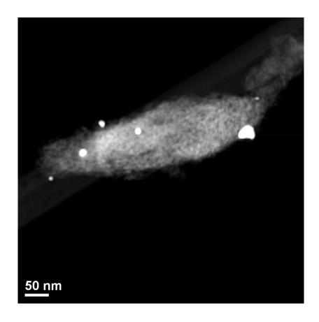
Figure 14 TEM image of Pt-B catalyst at a scale of 50nm
