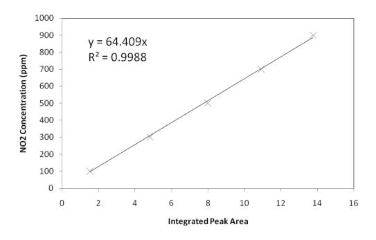
Figure 8 NO<sub>2</sub> Calibration. The peak area of NO<sub>2</sub> was integrated from 1660 to 1540 cm<sup>-1</sup>
