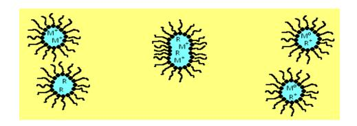
Figure 3 The surfactant stabilized the water (white) which contains the metal and reductant in the oil phase (yellow) (reproduced from [4]).
