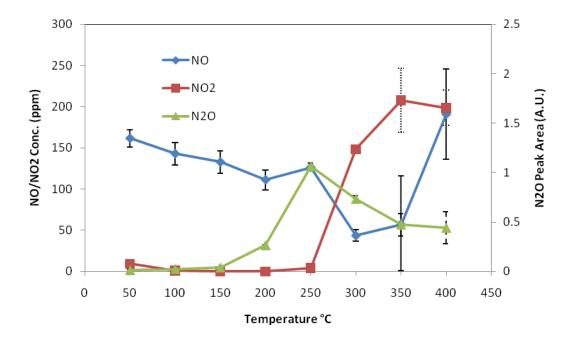
Figure 17 High-Throughput SCR data for 1Ru5Co15Ba catalyst
