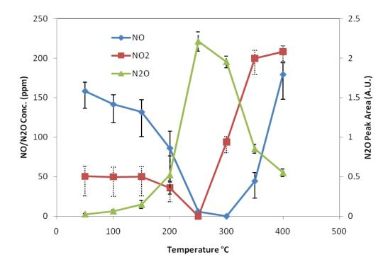
Figure 16 High-Throughput SCR data for 1Pt5Co15Ba catalyst
