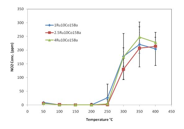
Figure 20 High-throughput data of NO<sub>2</sub> concentration for the 1Ru10Co15Ba, 2.5Ru10Co15Ba, and 4Ru10Co15Ba catalysts
