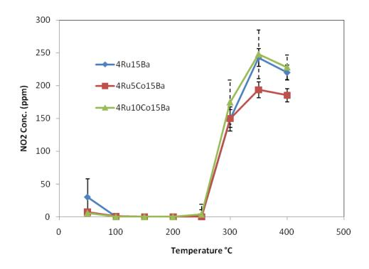
Figure 23 High-throughput data of NO₂ concentration for the 4Ru15Ba, 4Ru5Co15Ba, and 4Ru10Co15Ba catalysts
