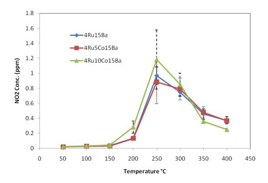
Figure 24 High-throughput data of N₂O concentration for the 4Ru15Ba, 4Ru5Co15Ba, and 4Ru10Co15Ba catalysts
