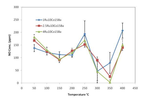
Figure 19 High-throughput data of NO concentration for the 1Ru10Co15Ba, 2.5Ru10Co15Ba, and 4Ru10Co15Ba catalysts
