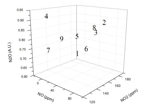
Figure 25 A 3-dimensional plot of the RuCoBa catalysts displaying the NO, NO $_2$ , and N $_2$ O concentrations at 300 $^{\circ}$ C
