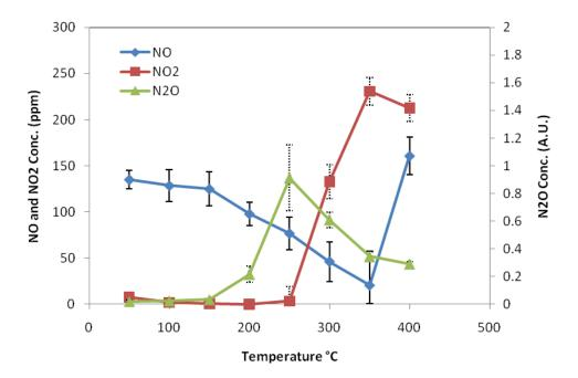
Figure 27 High-Throughput SCR data for 5Co15Ba catalyst
