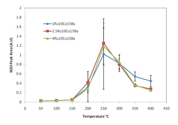
Figure 21 High-throughput data of N₂O concentration for the 1Ru10Co15Ba, 2.5Ru10Co15Ba, and 4Ru10Co15Ba catalysts
