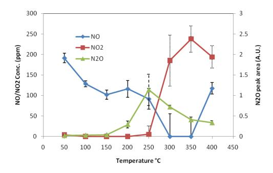
Figure 11 High-Throughput SCR data for Ru-B catalyst
