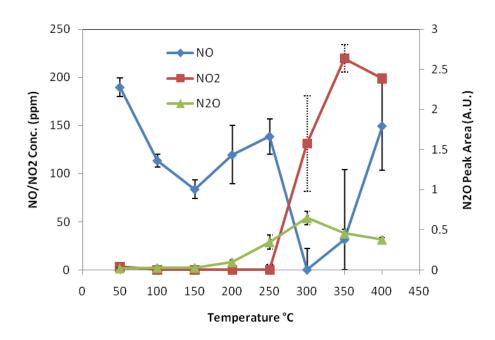
Figure 9 High-Throughput SCR data for Ru-X catalyst
