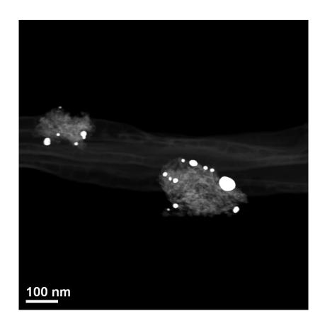
Figure 13 TEM image of Pt-B catalyst at a scale of 100nm
