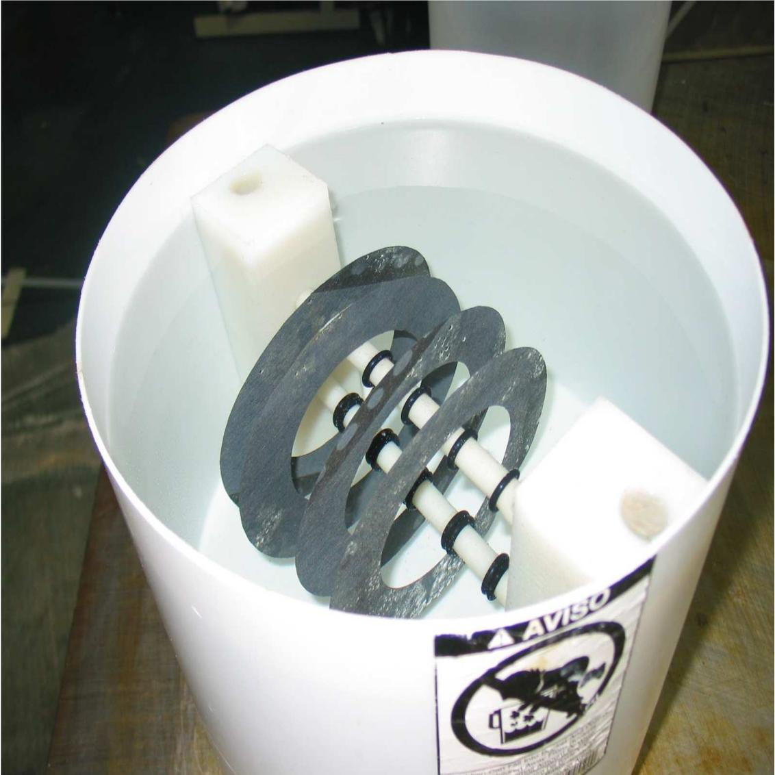
**Figure 6: Submerged GDLs in Pure Water**
