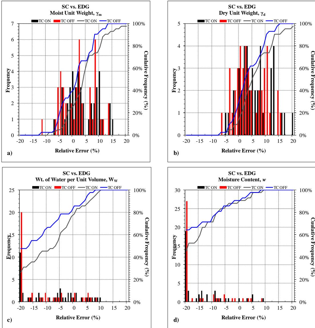
**Figure 6.22** Relative Error Histograms and CDF Plots – SC vs. EDG (Mold Soil Model)
