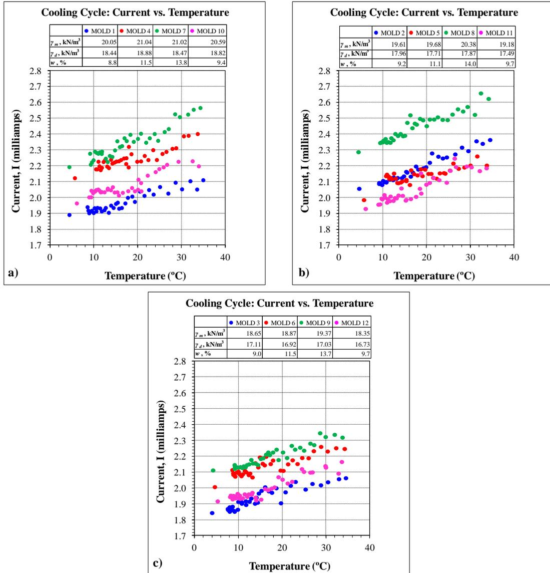
**Figure C.2 Cooling Cycle: Current vs. Temperature**
