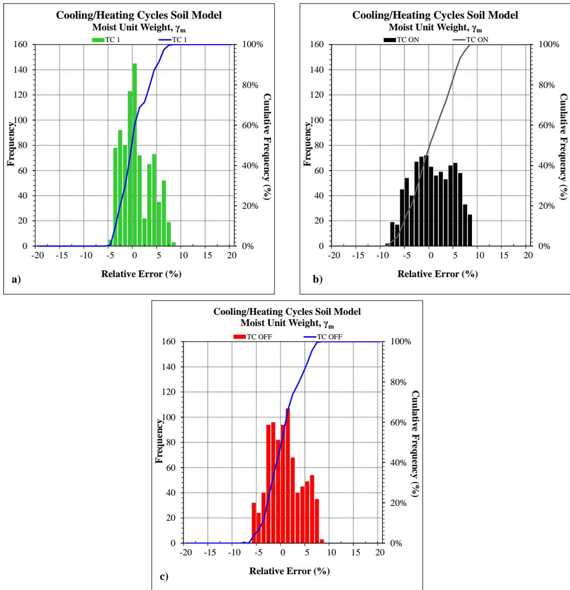
**Figure 8.17** Relative Error Histograms and CDF Plots – Cooling/Heating Cycles Soil Model
