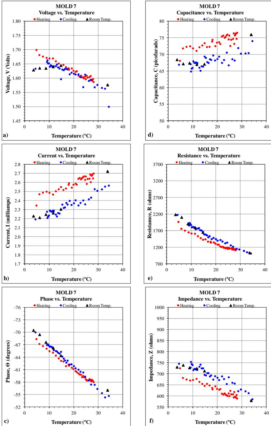
**Figure A.7 Electrical Properties Recorded Using the EDG vs. Temperature (MOLD 7)**
