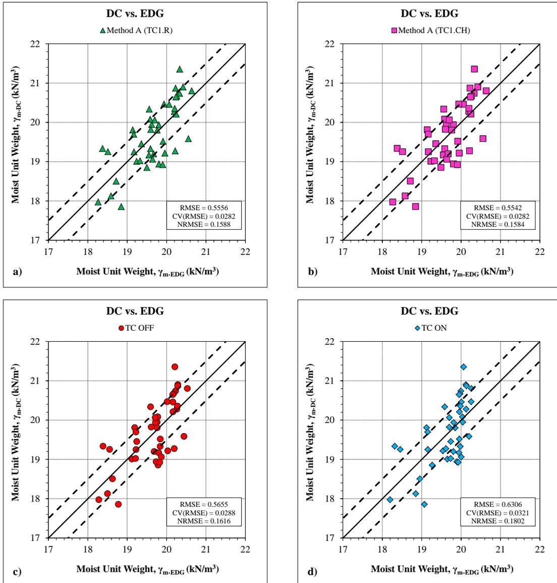
**Figure 9.7 1:1 Plots – Large Box Soil Model (Method A)**
