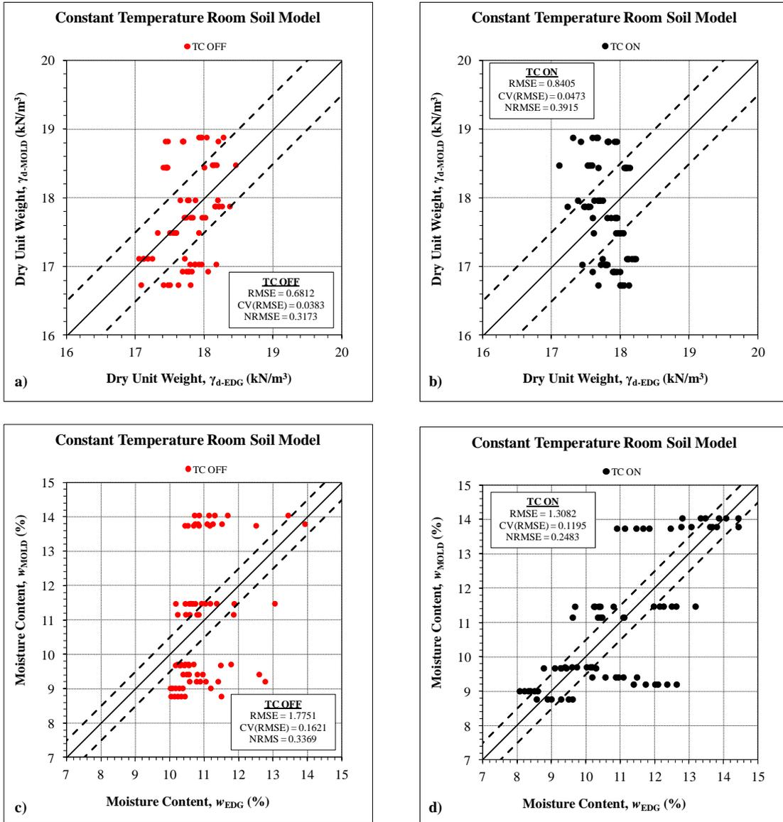
**Figure 7.6 1:1 Plots – Constant temperature Room Soil Model (TC OFF & TC ON)**
