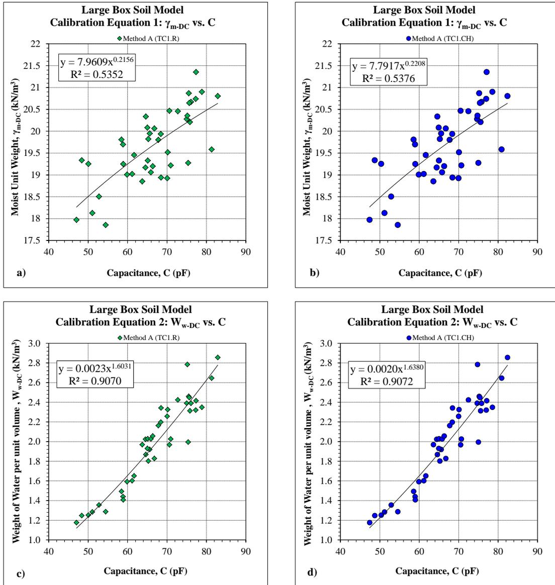
**Figure 9.3 Calibration Equations – Large Box Soil Model (Method A)**
