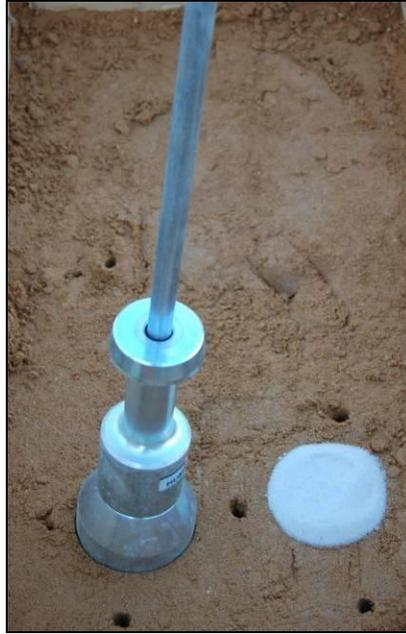
**Figure 6.10 Drive Cylinder test performed in Large Box**
