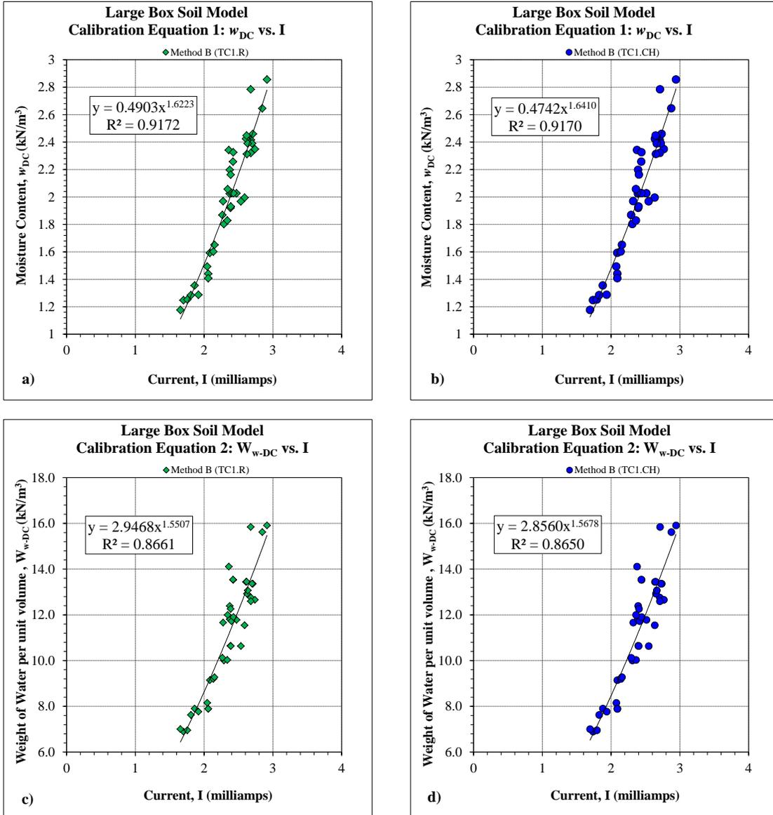
**Figure 9.4 Calibration Equations – Large Box Soil Model (Method B)**
