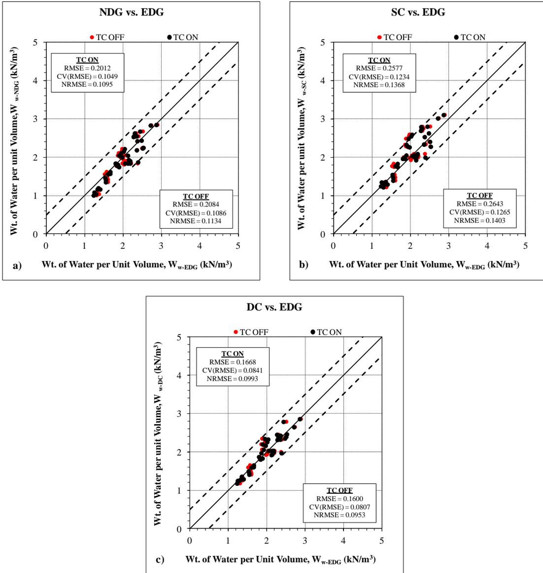
**Figure 6.26 Large Box Soil Model Results – Weight of Water per Unit Volume**
