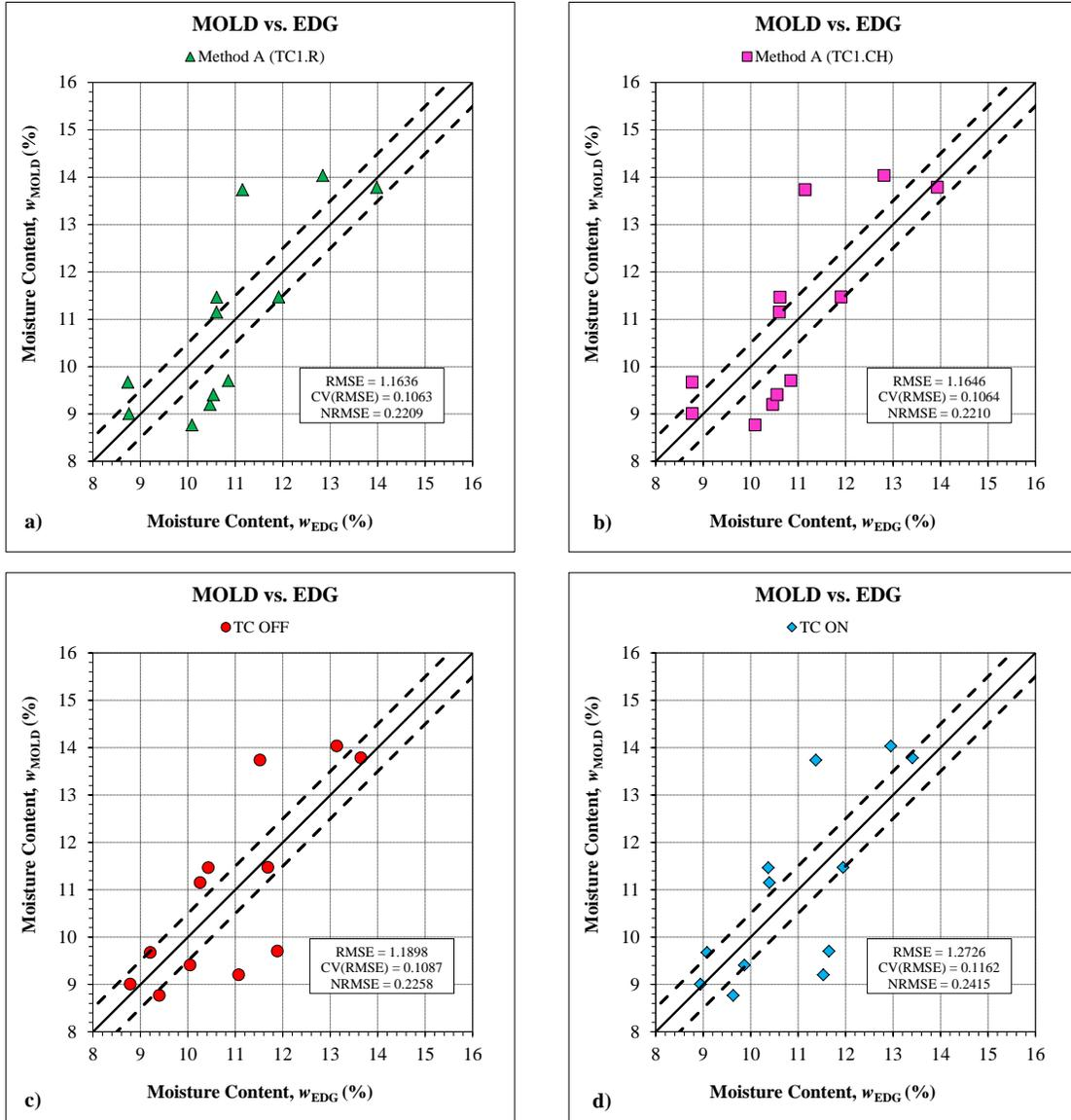
**Figure 9.17 1:1 Plots – Mold Soil Model (Method A)**
