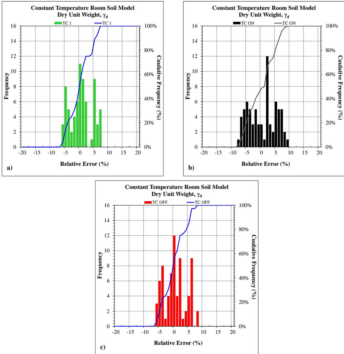
**Figure 8.15 Relative Error Histograms and CDF Plots – Constant Temperature Room Soil Model**
