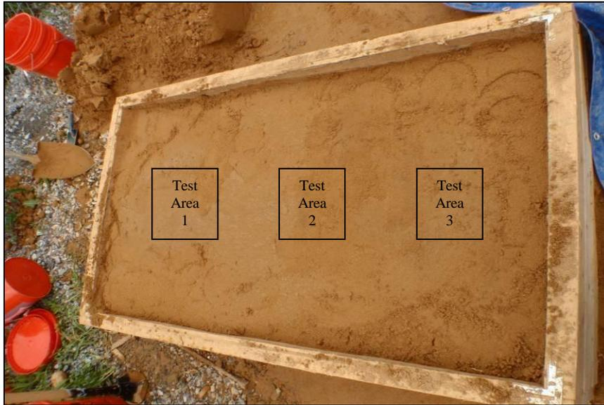
**Figure 6.6** Large box before performing in-situ density tests
