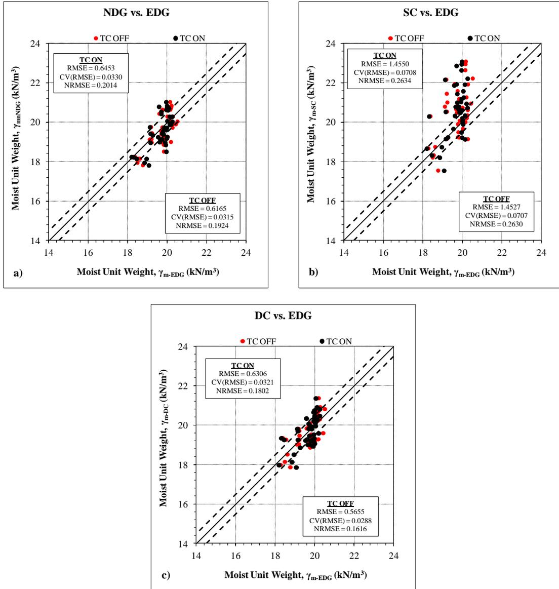
**Figure 6.25 Large Box Soil Model Results – Moist Unit Weight**
