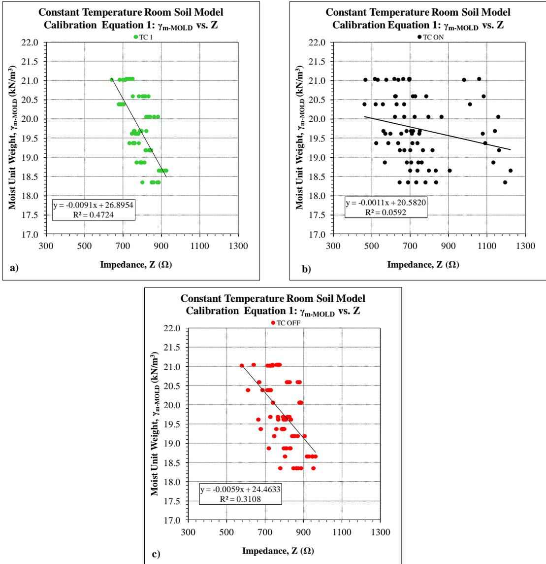
**Figure 8.1 Calibration Equations – Constant Temperature Room Soil Model**
