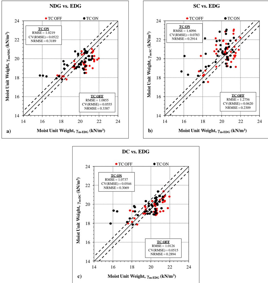
**Figure 6.17 Large Box Test Results: Mold Soil Model – Moist Unit Weight**
