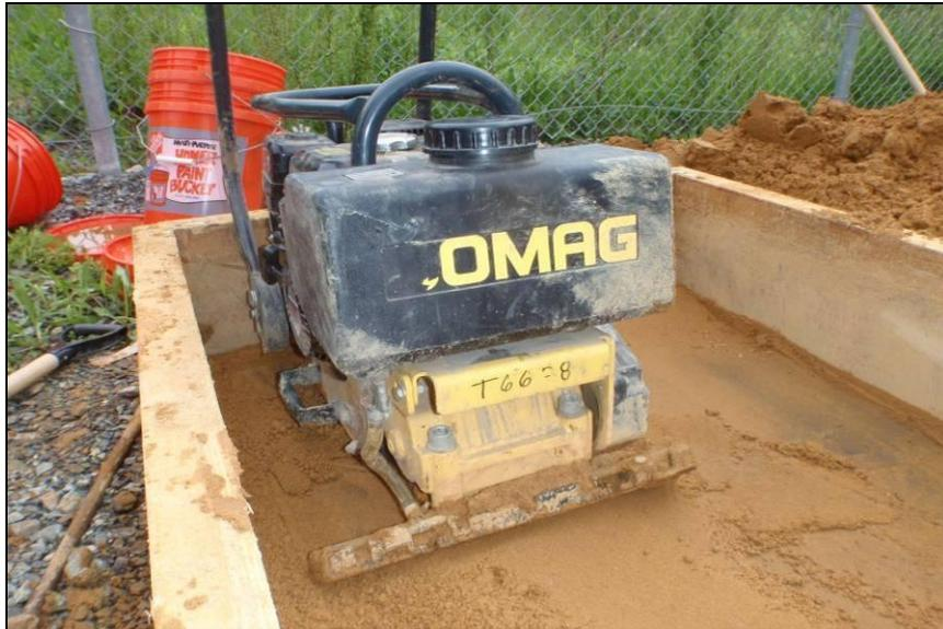
**Figure 6.5** Soil Compacted with walk-behind vibratory plate compactor
