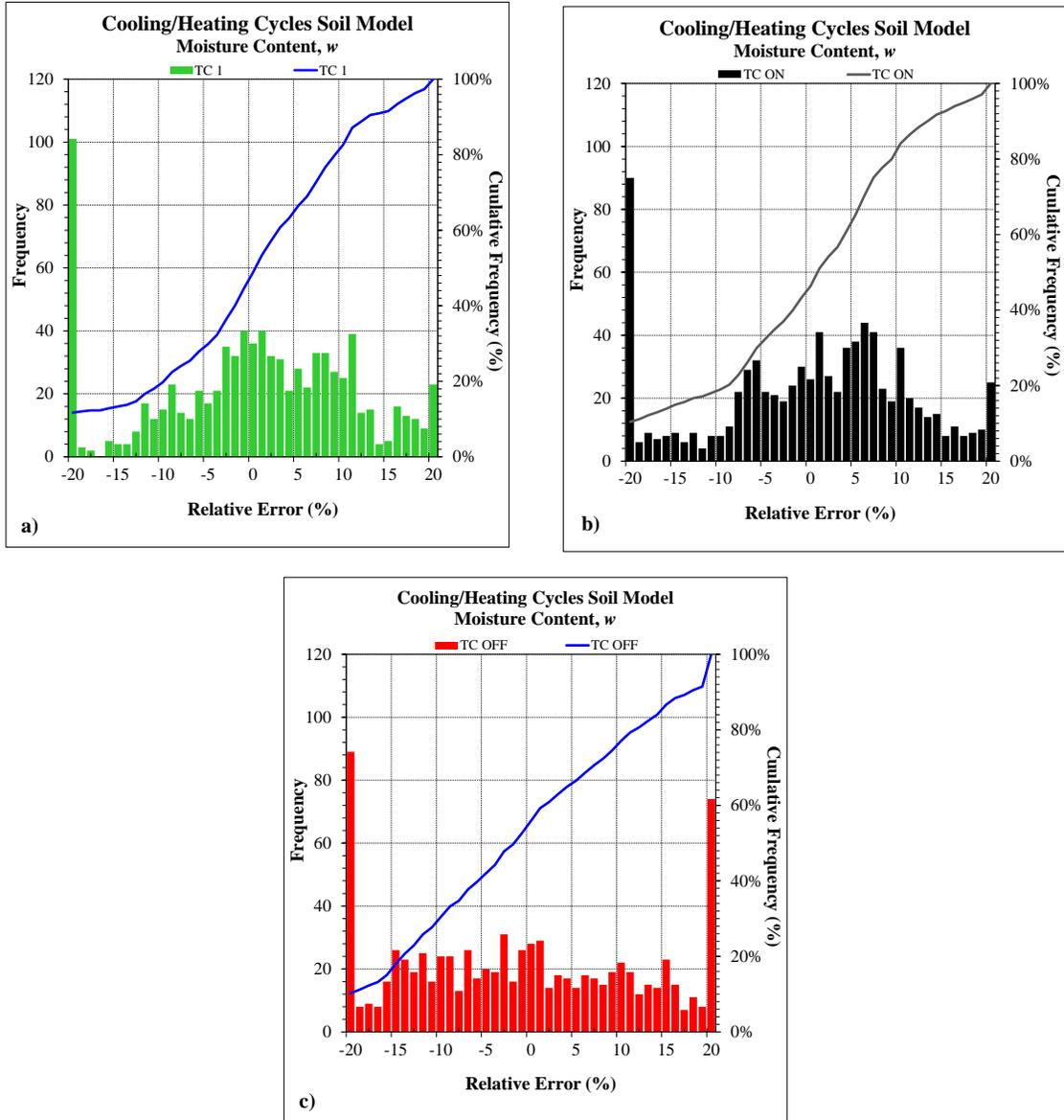
**Figure 8.20 Relative Error Histograms and CDF Plots – Cooling/Heating Cycles Soil Model**
