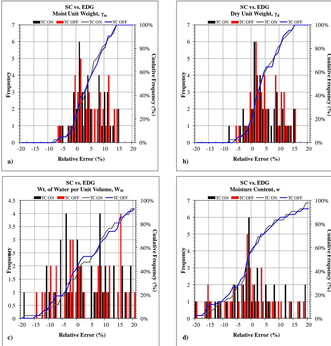
**Figure 6.30 Relative Error Histograms and CDF Plots – SC vs. EDG**
