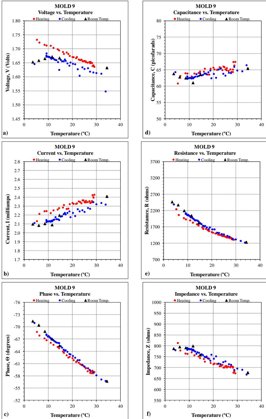
**Figure A.9 Electrical Properties Recorded Using the EDG vs. Temperature (MOLD 9)**
