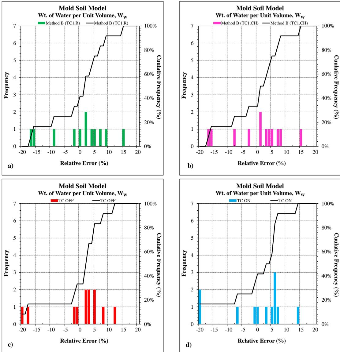
**Figure 9.26 Relative Error Histograms and CDF Plots – Mold Soil Model (Method B)**
