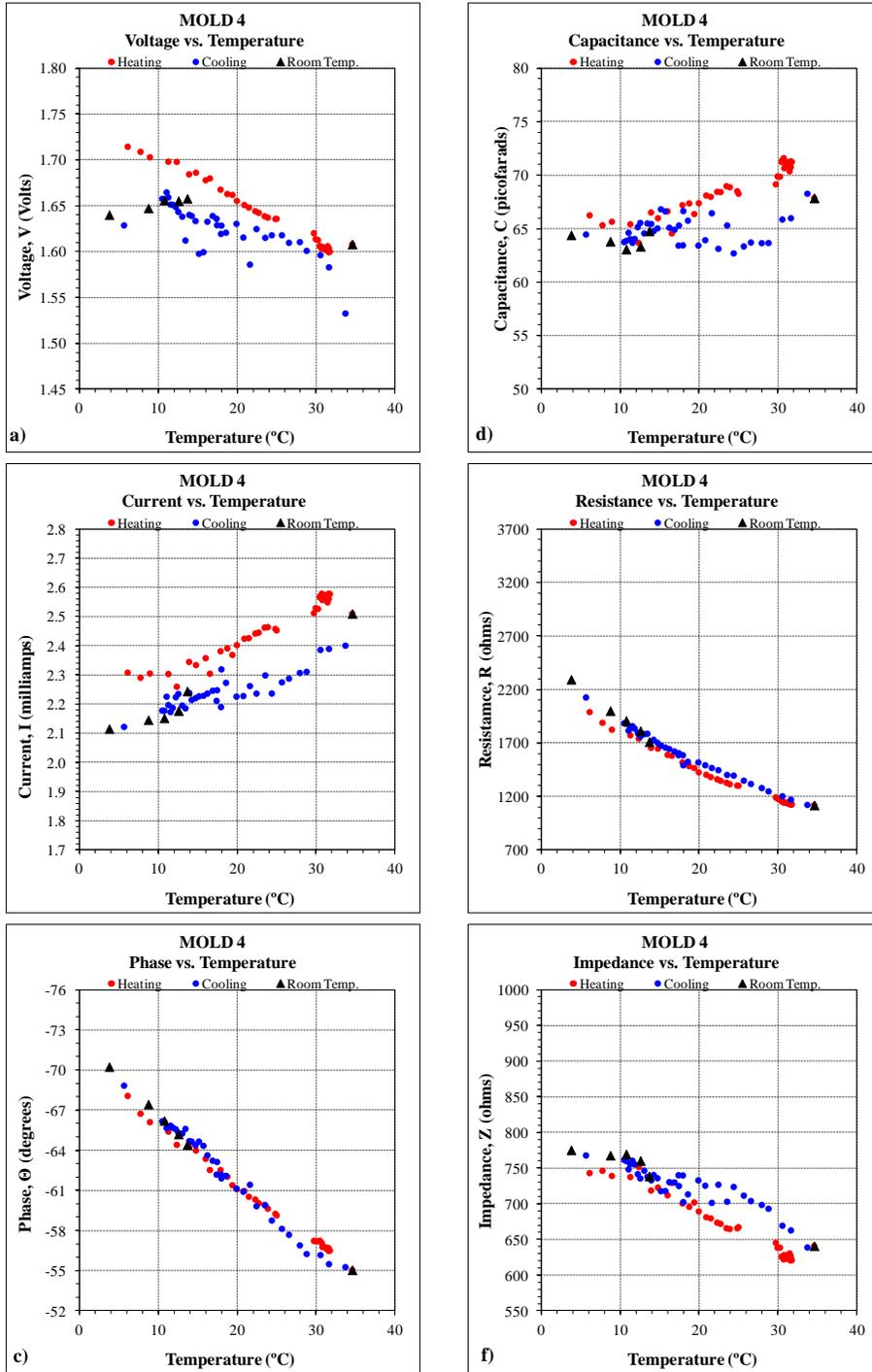
**Figure A.4 Electrical Properties Recorded Using the EDG vs. Temperature (MOLD 4)**
