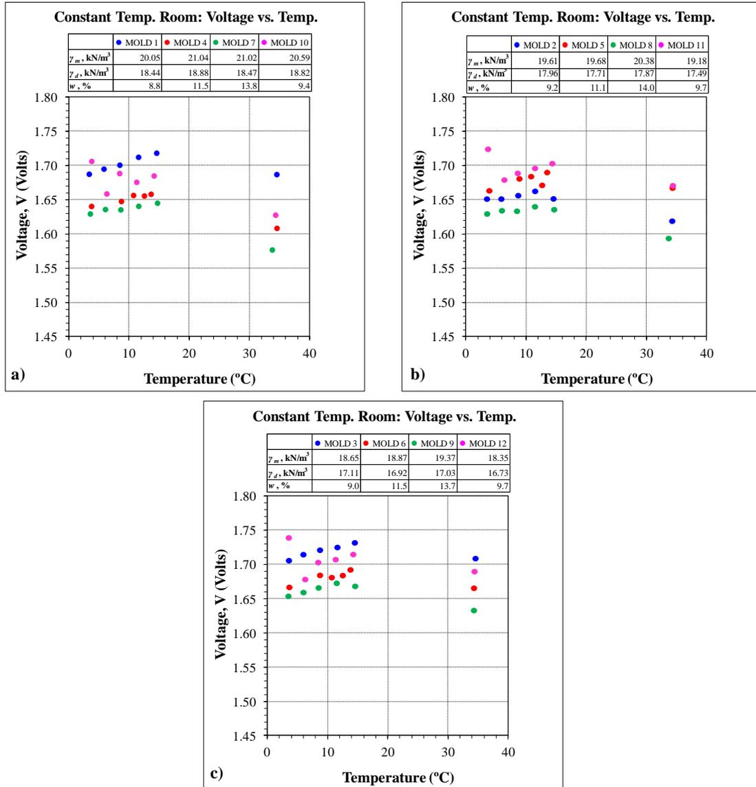
**Figure C.13 Constant Temperature Room Testing: Voltage vs. Temperature**
