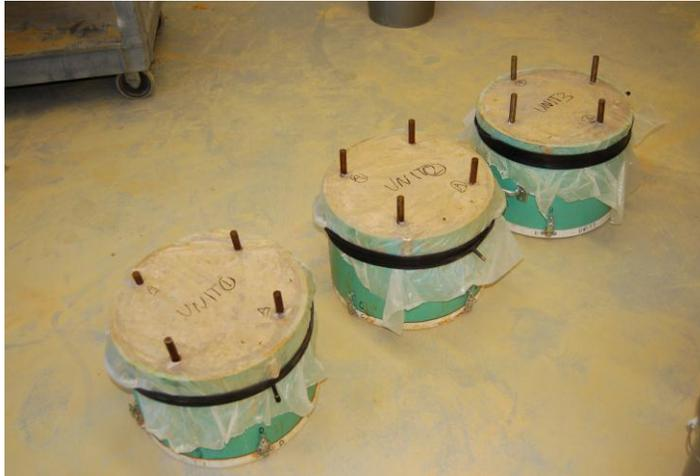
**Figure 7.2** Compacted soil molds wrapped in plastic for temperature testing experiments
