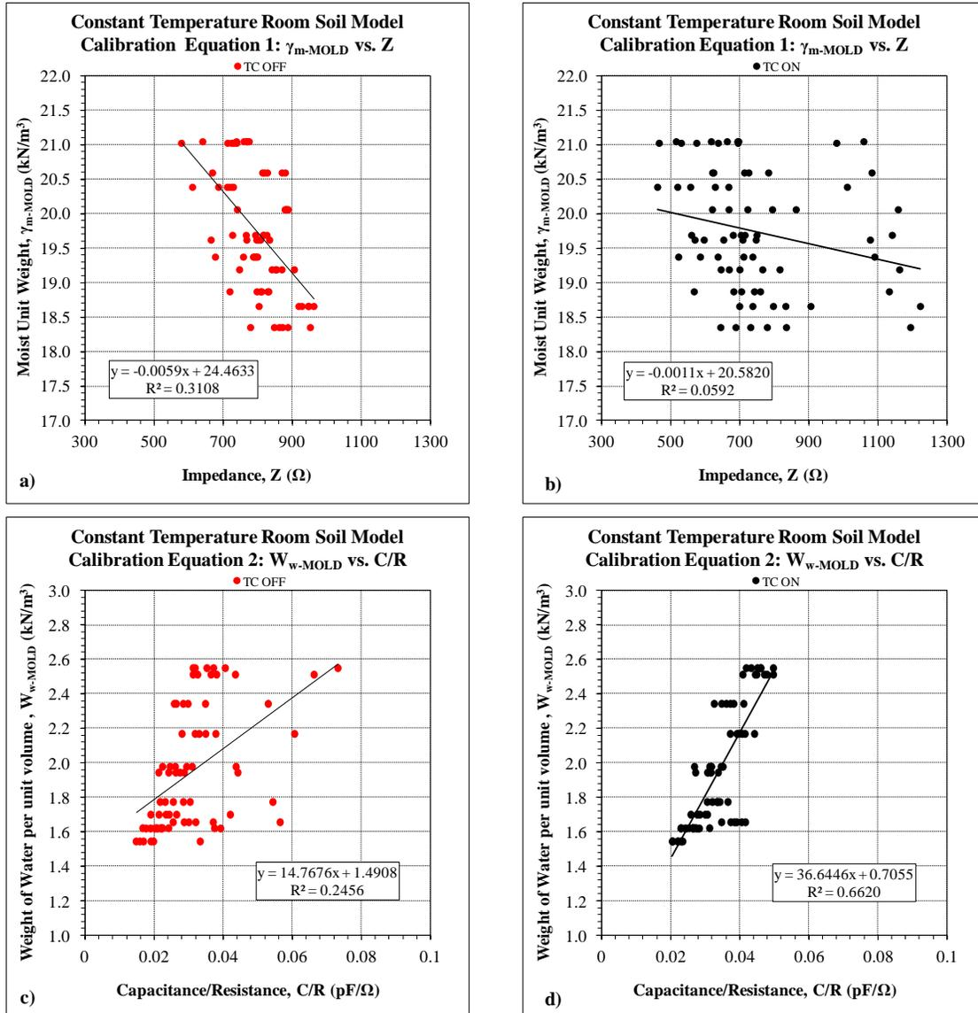
**Figure 7.3 Calibration Equations – Constant Temperature Room Soil Model**
