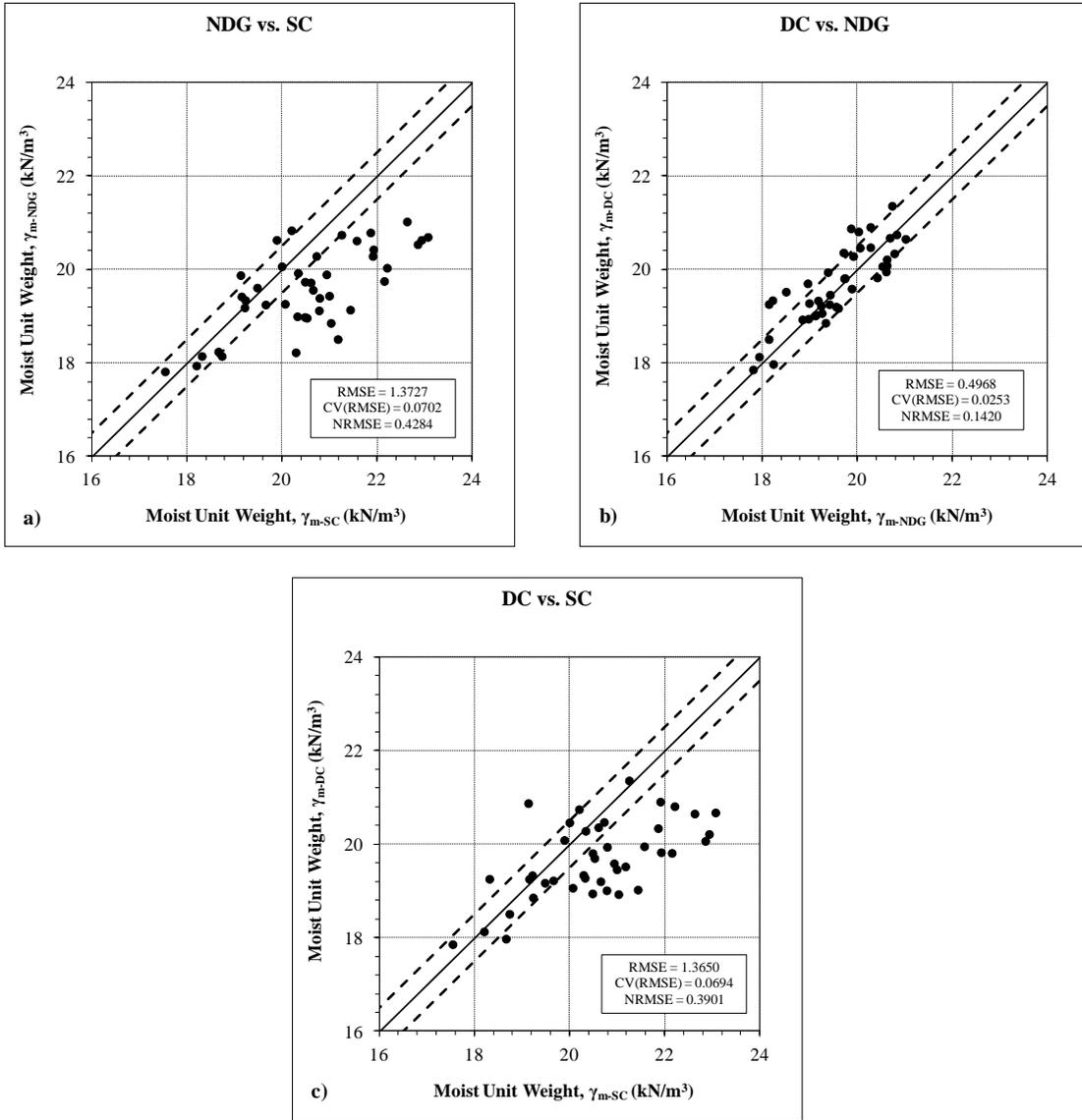
**Figure 6.12 Standard Large Box Tests – Moist Unit Weight**
