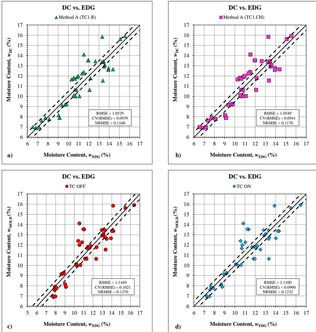
**Figure 9.19 1:1 Plots – Large Box Soil Model (Method A)**
