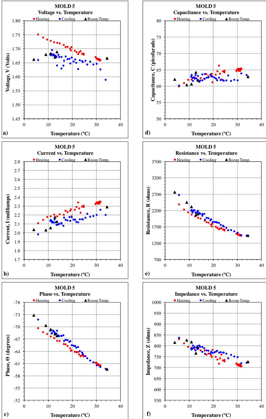
**Figure A.5 Electrical Properties Recorded Using the EDG vs. Temperature (MOLD 5)**
