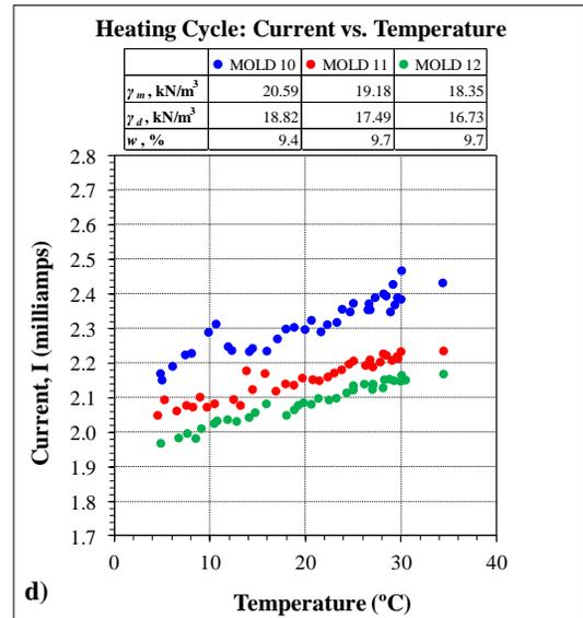
**Figure B.8 Heating Cycle: Current vs. Temperature**
