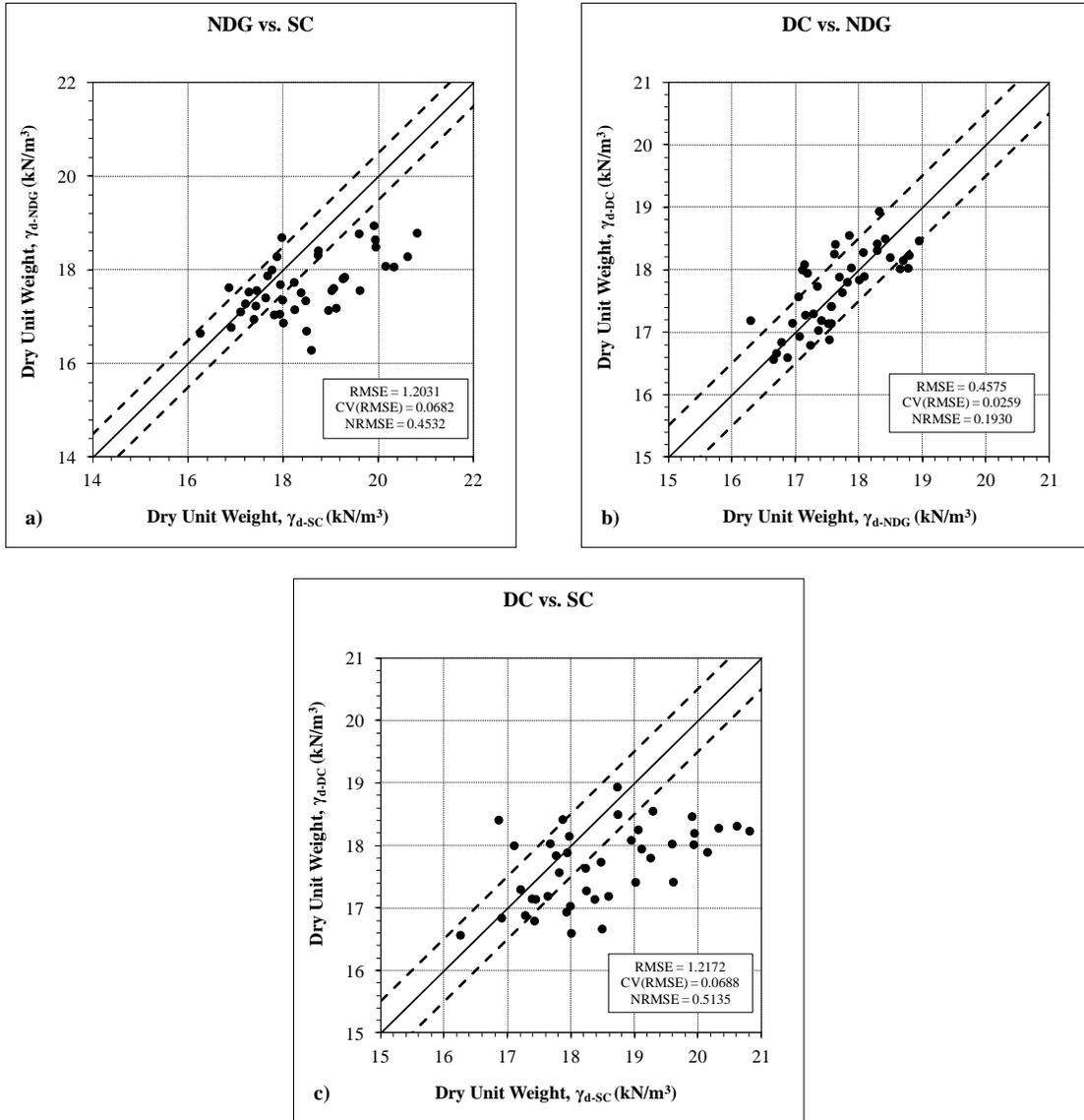
**Figure 6.14 Standard Large Box Tests – Dry Unit Weight**
