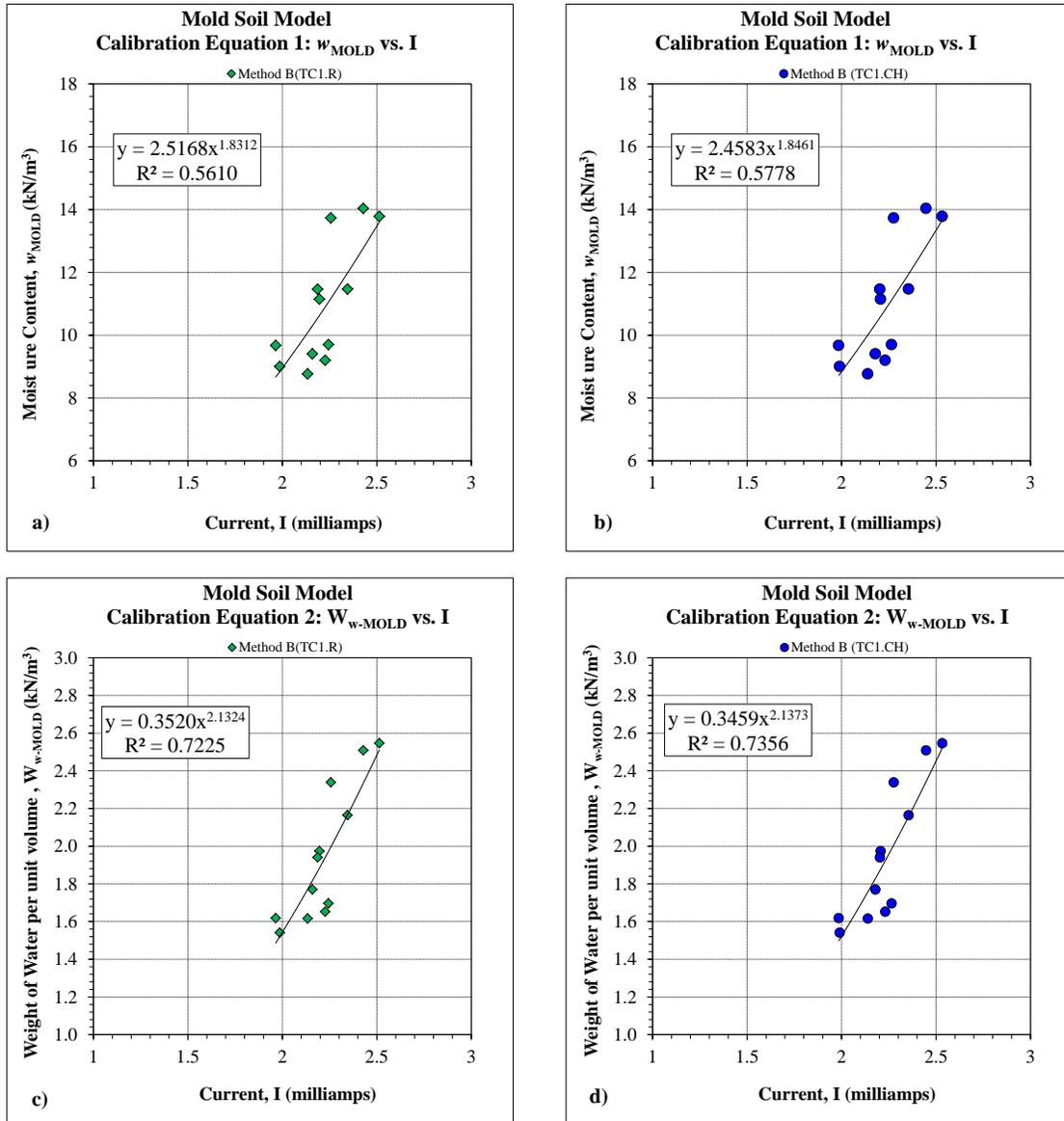
**Figure 9.2 Calibration Equations – Mold Soil Model (Method B)**
