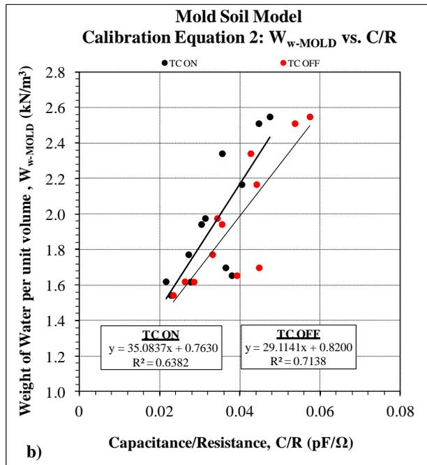
**Figure 5.5 Calibration Equations – Mold Soil Model (TC OFF & TC ON)**
