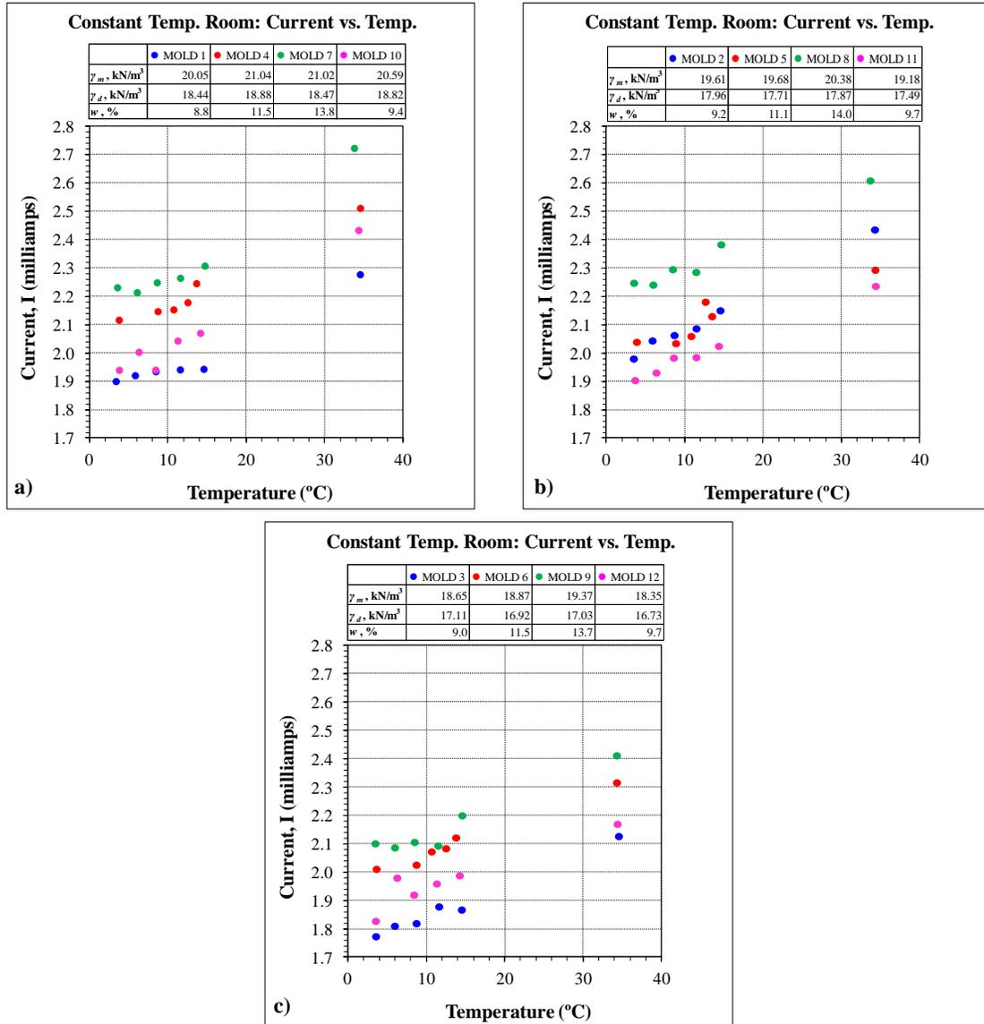
**Figure C.14 Constant Temperature Room Testing: Current vs. Temperature**
