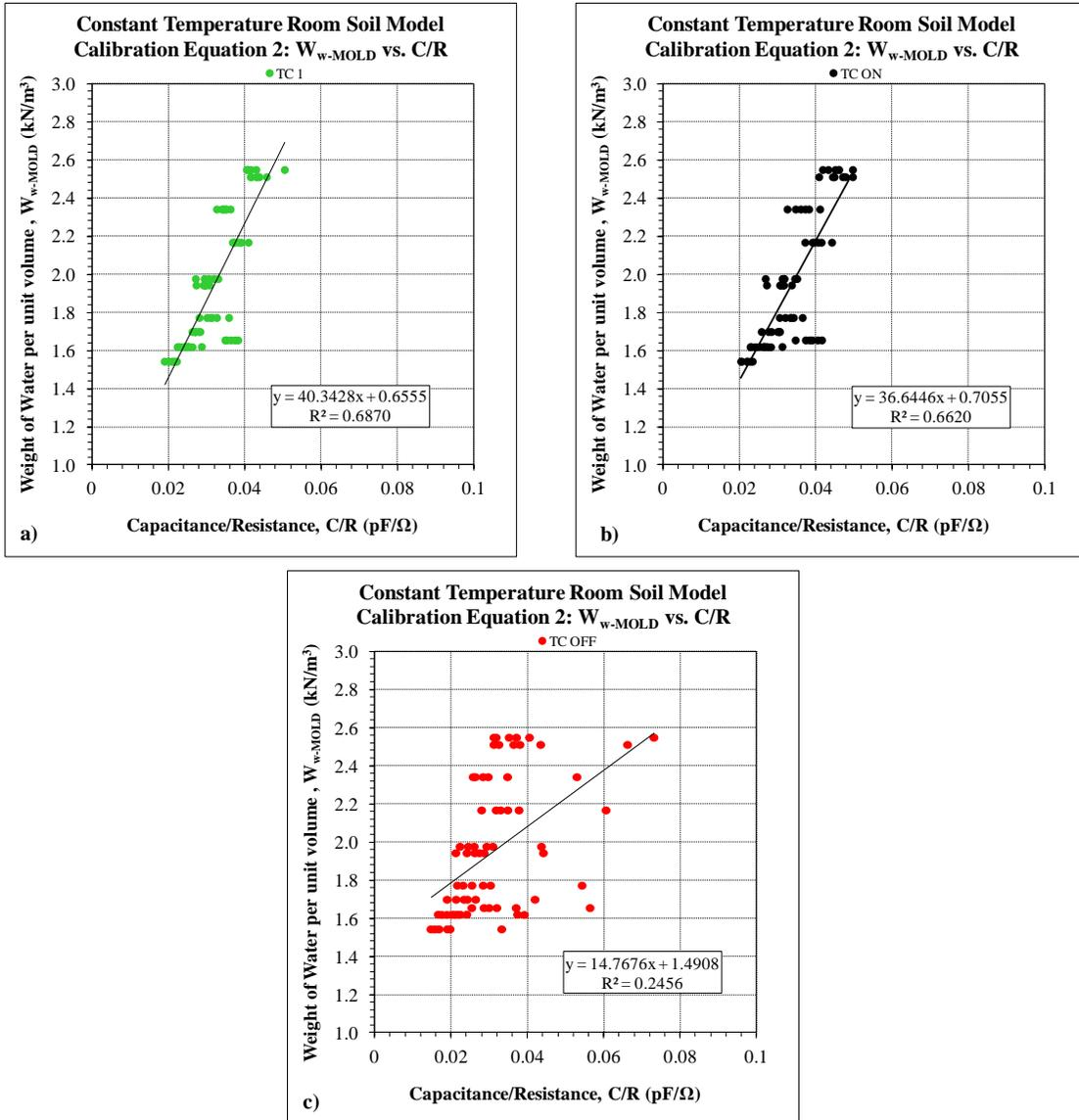
**Figure 8.2 Calibration Equations – Constant Temperature Room Soil Model**
