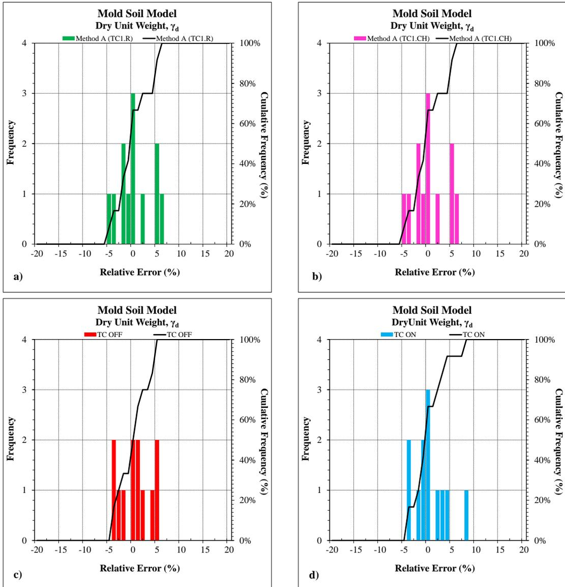
**Figure 9.29 Relative Error Histograms and CDF Plots – Mold Soil Model (Method A)**
