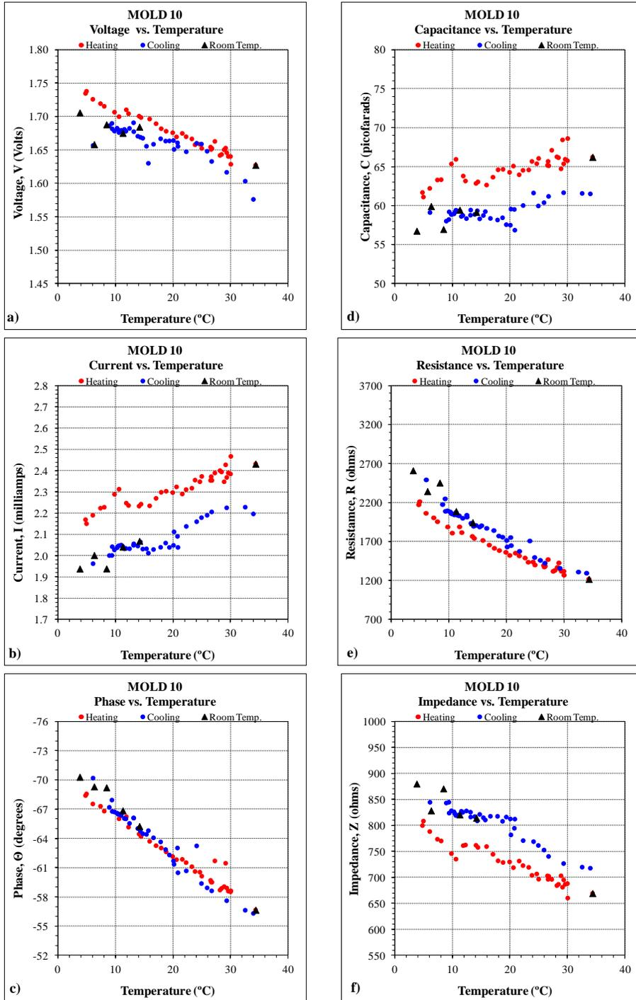
**Figure A.10 Electrical Properties Recorded Using the EDG vs. Temperature (MOLD 10)**
