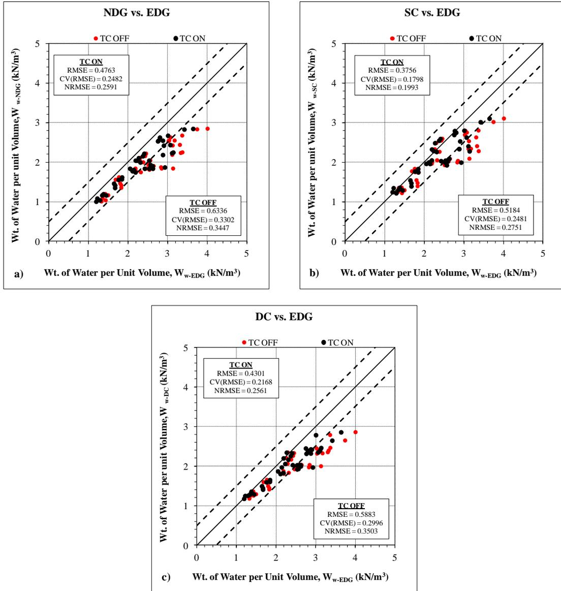
**Figure 6.18 Large Box Test Results: Mold Soil Model – Weight of Water per Unit Volume**
