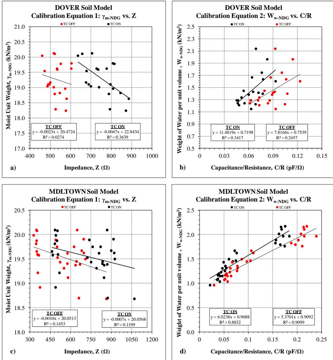
**Figure 4.7 Calibration Equations**
