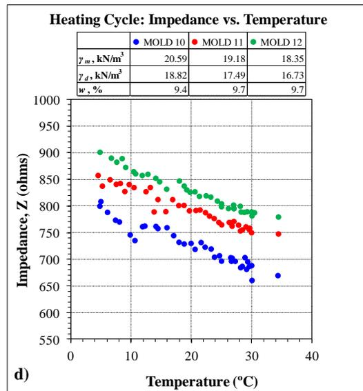
**Figure B.12 Heating Cycle: Impedance vs. Temperature**
