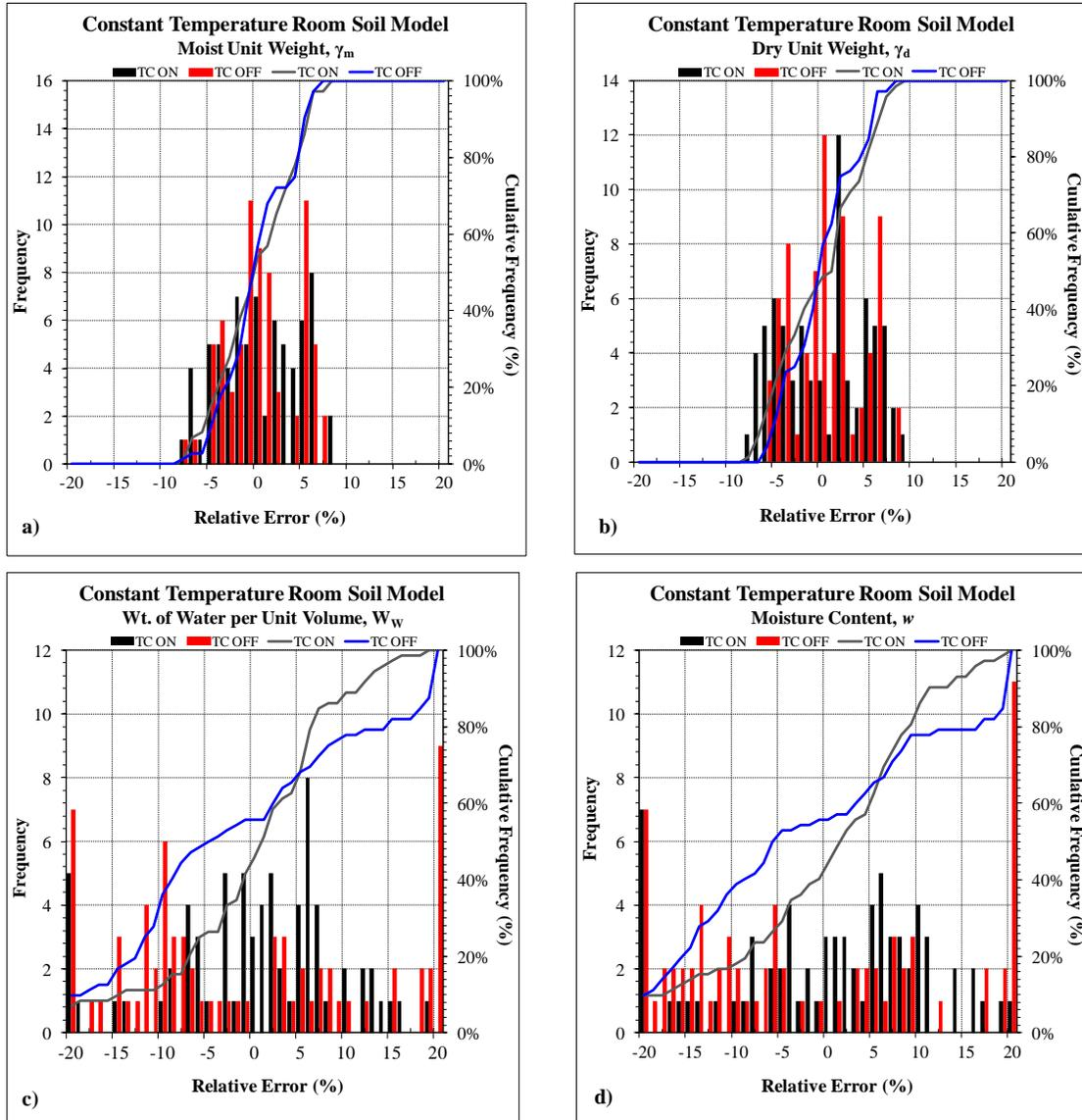
**Figure 7.9** Relative Error Histograms and CDF Plots – Constant Temperature Room Soil Model
