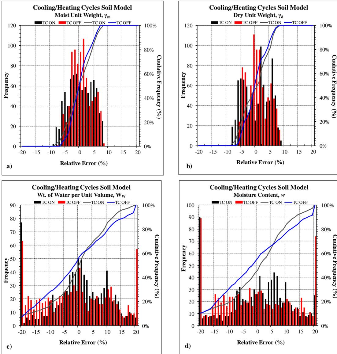
**Figure 7.10** Relative Error Histograms and CDF Plots – Cooling/Heating Cycles Soil Model
