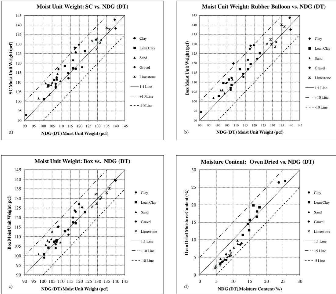
**Figure 2.10 1:1 Plots – Moist Unit Weight and Moisture Content**
