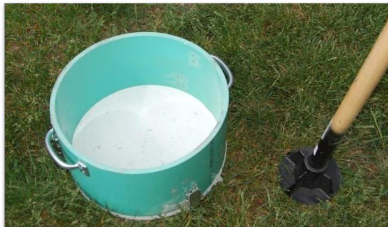
**Figure 5.1** Large “Proctor” type mold and tamper
