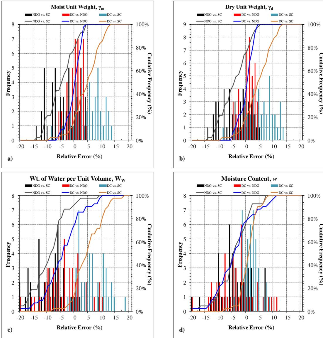
**Figure 6.16** Relative Error Histograms and CDF Plots – Standard Field Tests
