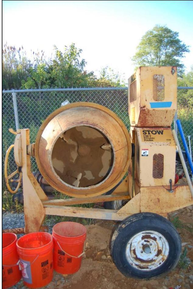
**Figure 6.3 Concrete Mixer used to mix soil to different moisture contents**
