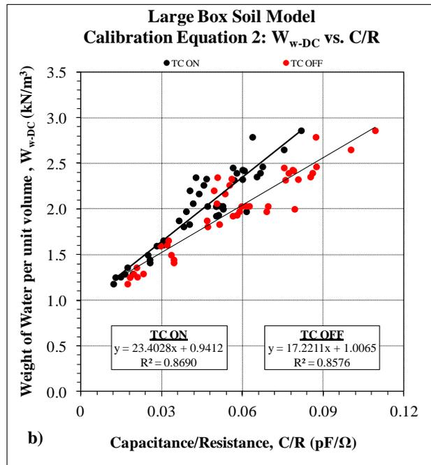
**Figure 6.24 Calibration Equations – Large Box Soil Model (TC OFF & TC ON)**
