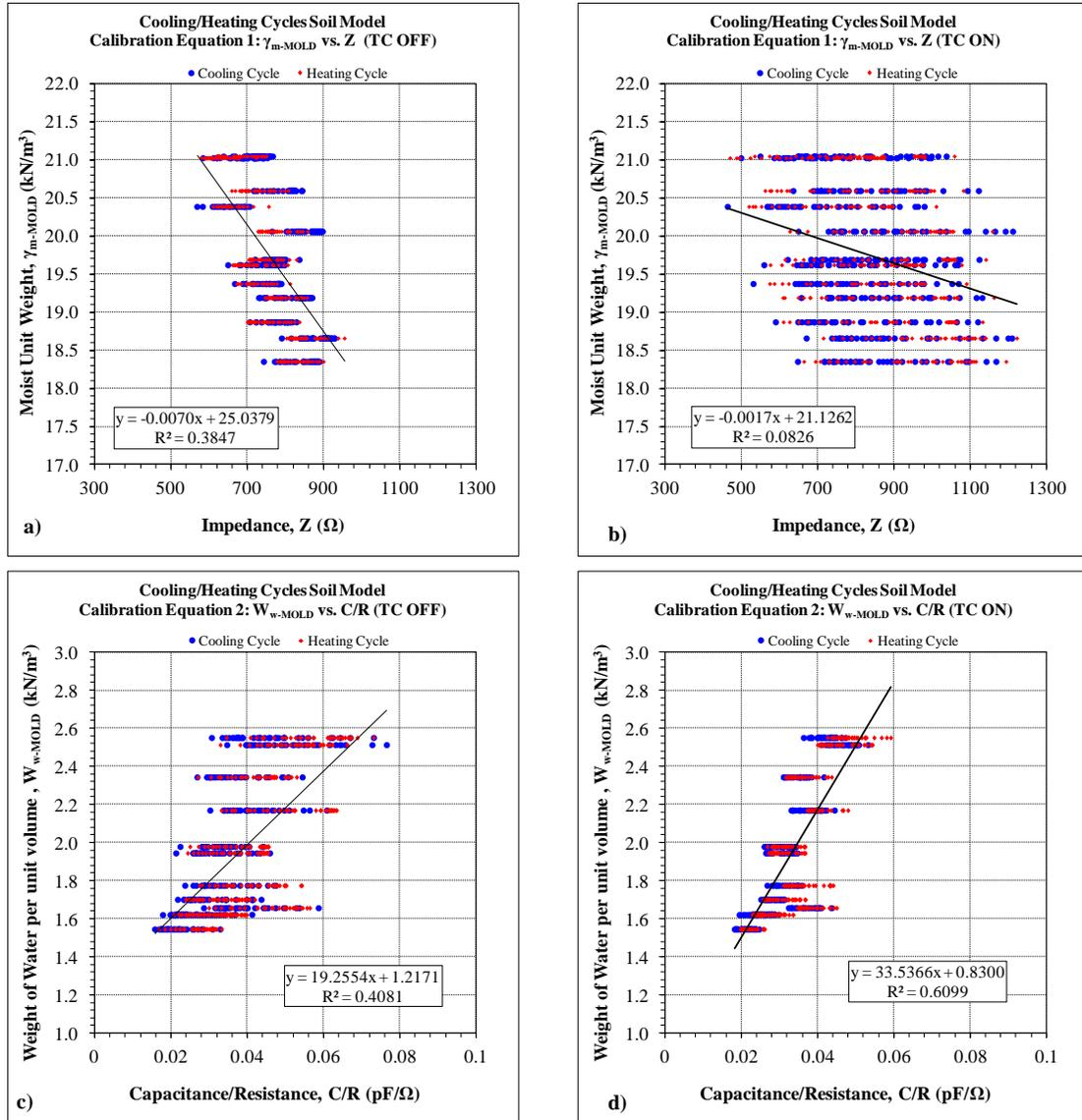
**Figure 7.4 Calibration Equations – Cooling/Heating Cycles Soil Model**
