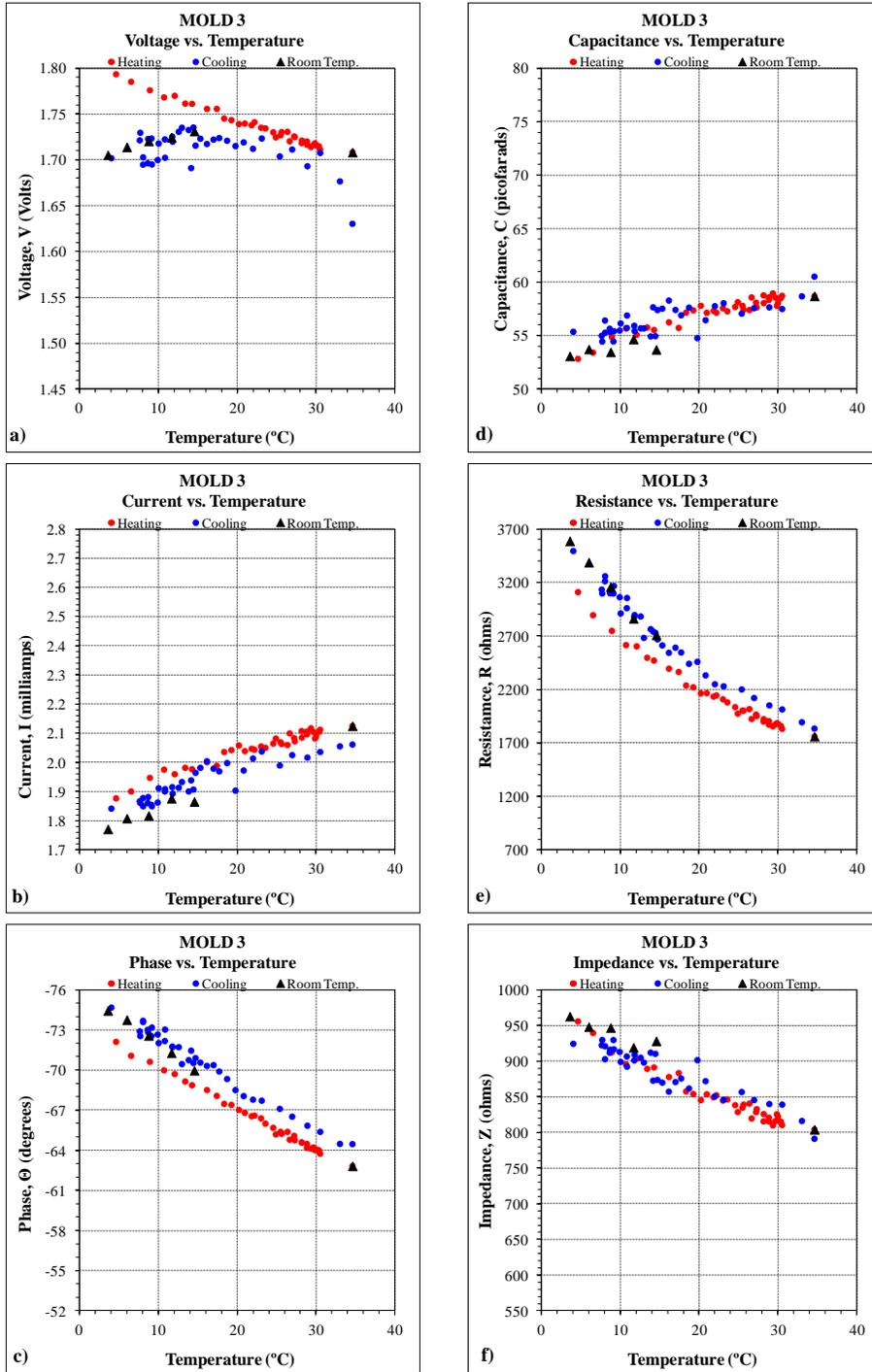
**Figure A.3 Electrical Properties Recorded Using the EDG vs. Temperature (MOLD 3)**
