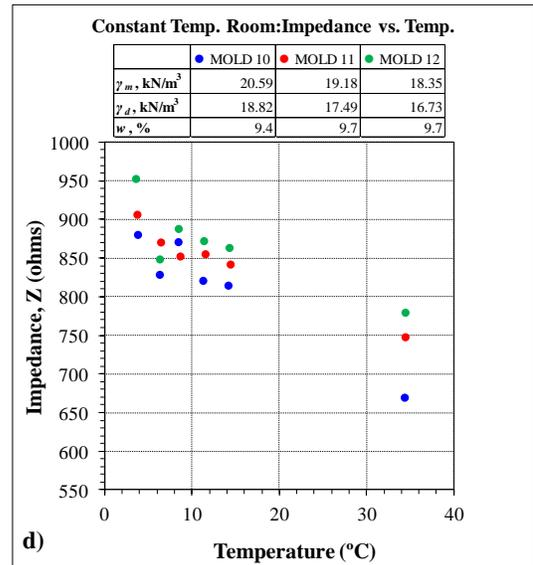
**Figure B.18 Constant Temperature Room Testing: Impedance vs. Temperature**
