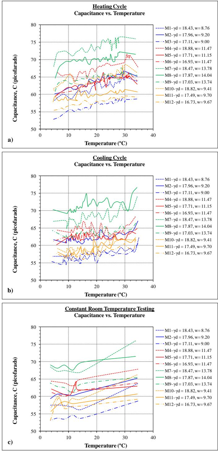
**Figure D.4 Capacitance vs. Temperature**
