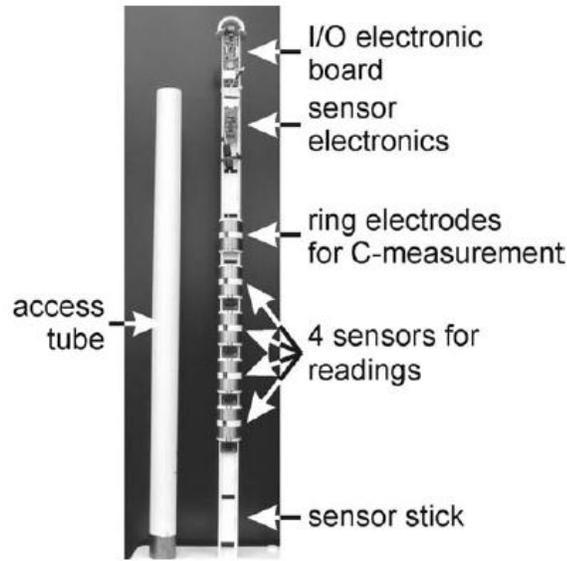
**Figure 2.6 Capacitance Sensor (modified from Schwank et al. 2006)**
