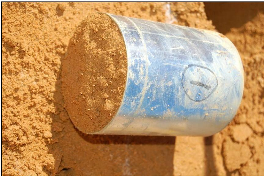
**Figure 6.11 Drive Cylinder after excavation from hole**
