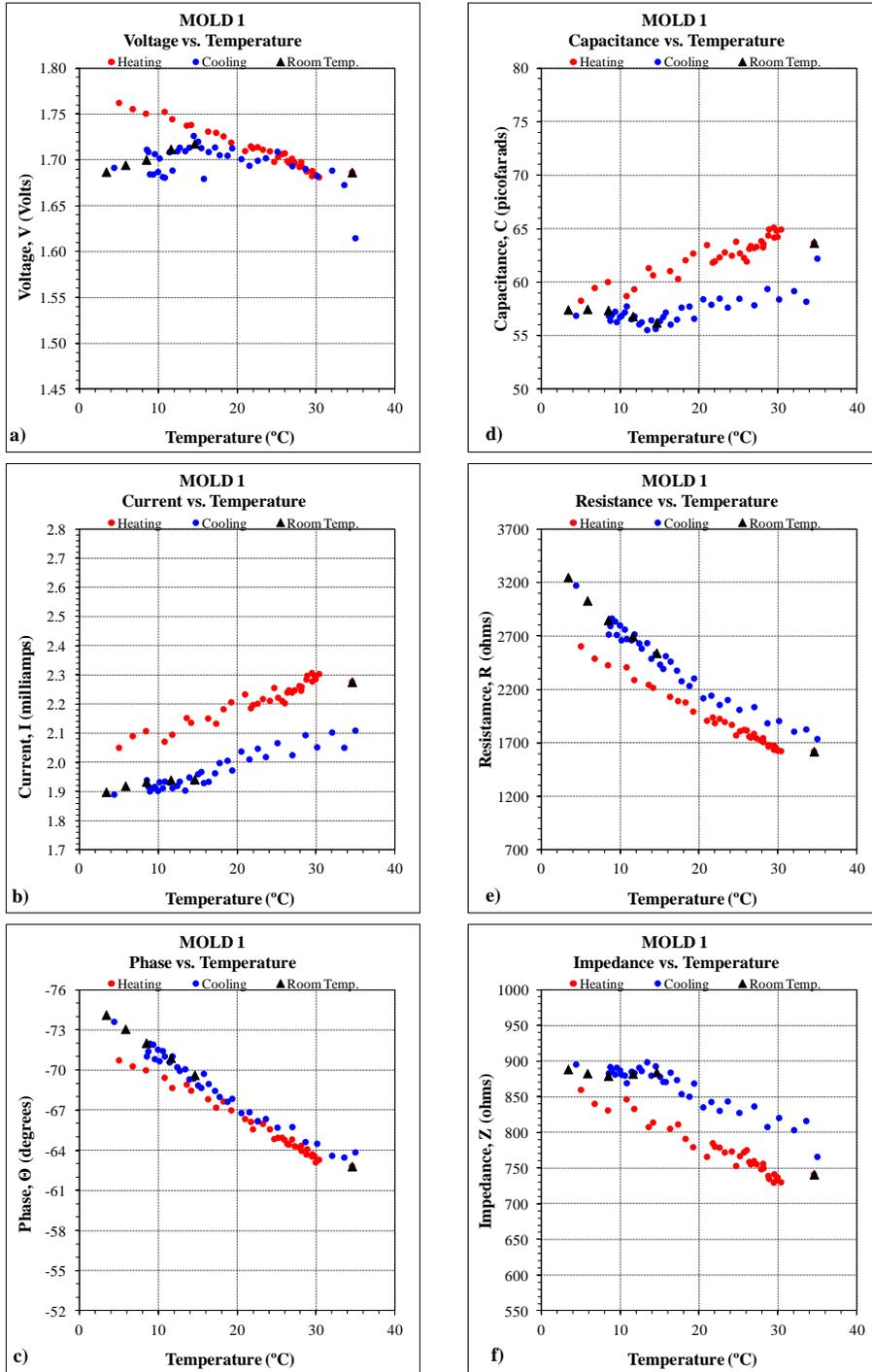
**Figure A.1 Electrical Properties Recorded Using the EDG vs. Temperature (MOLD 1)**
