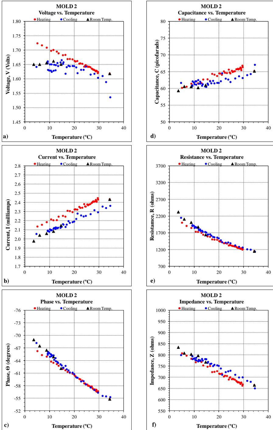
**Figure A.2 Electrical Properties Recorded Using the EDG vs. Temperature (MOLD 2)**
