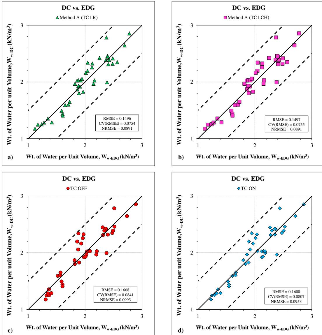
**Figure 9.11 1:1 Plots Large Box Soil Model (Method A)**
