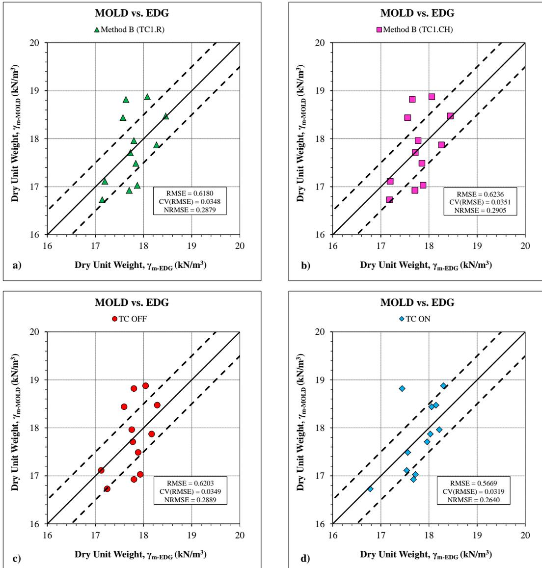
**Figure 9.14 1:1 Plots – Mold Soil Model (Method B)**
