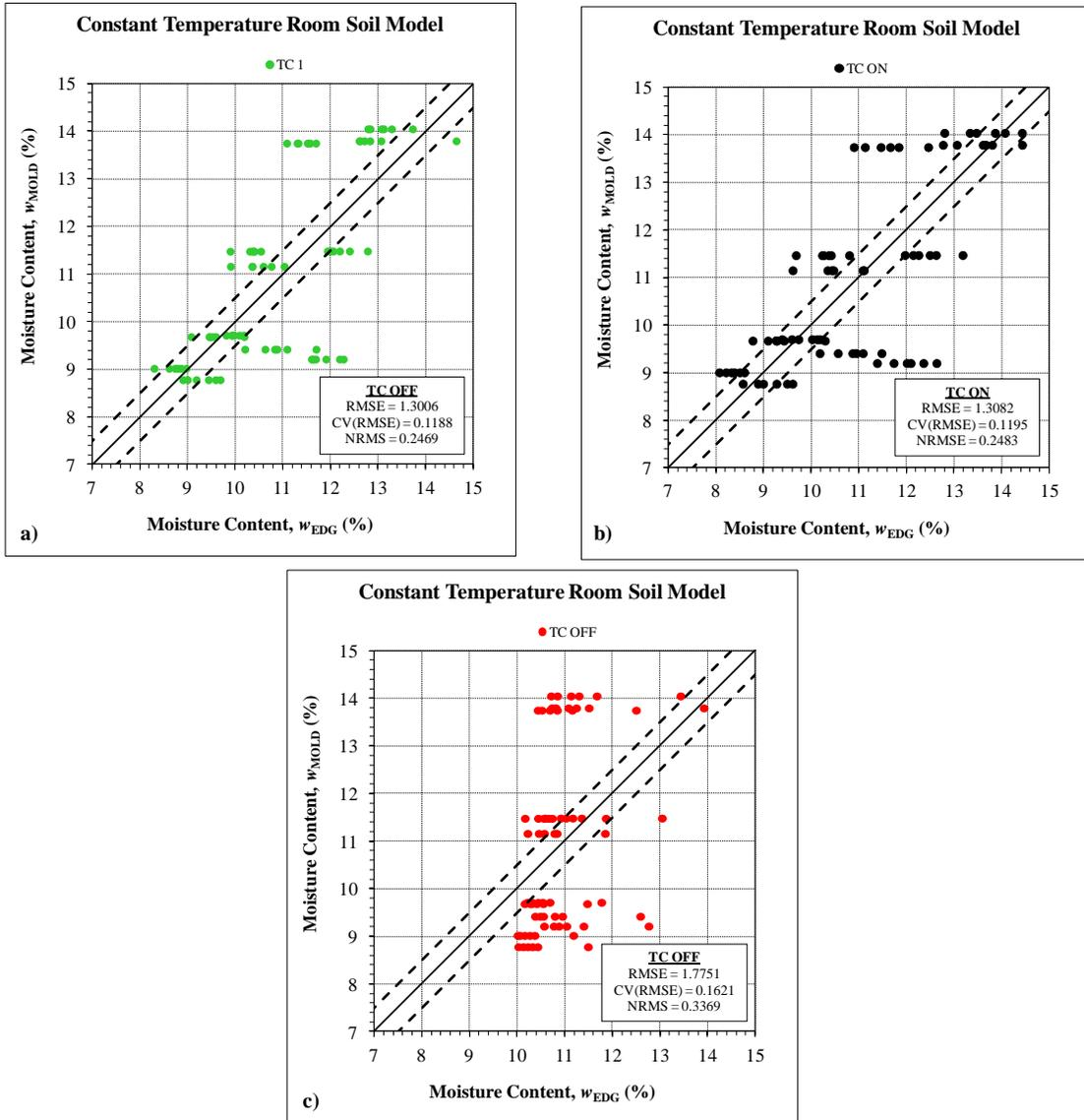
**Figure 8.8 1:1 Plots – Constant Temperature Room Soil Model**
