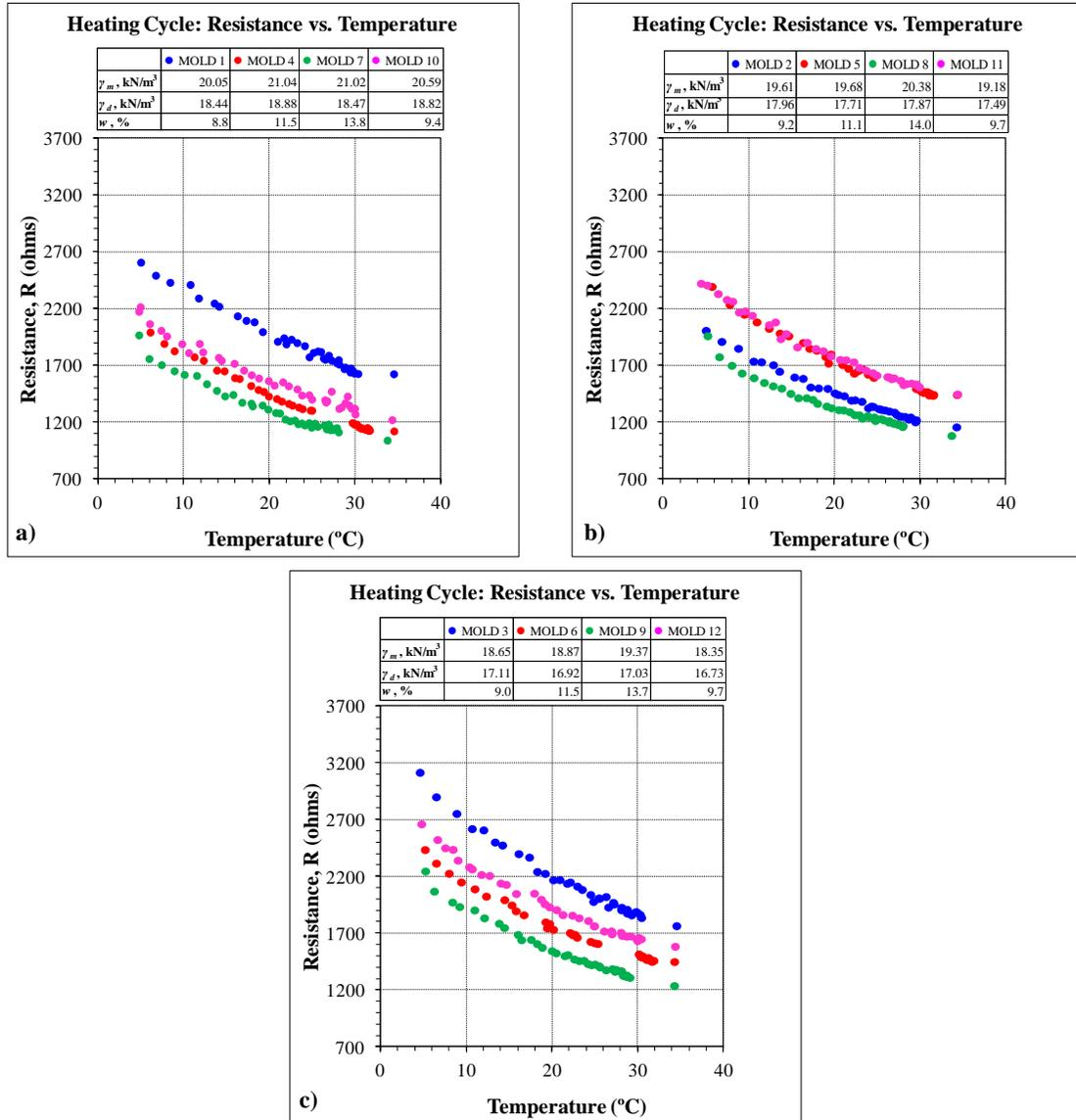
**Figure C.11 Heating Cycle: Resistance vs. Temperature**
