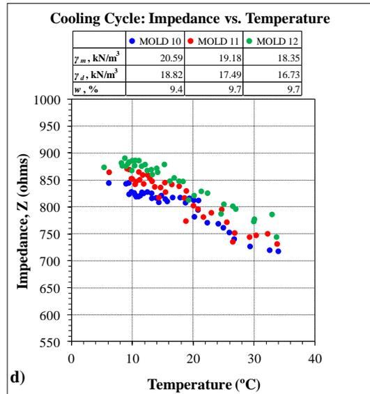
**Figure B.6 Cooling Cycle: Impedance vs. Temperature**
