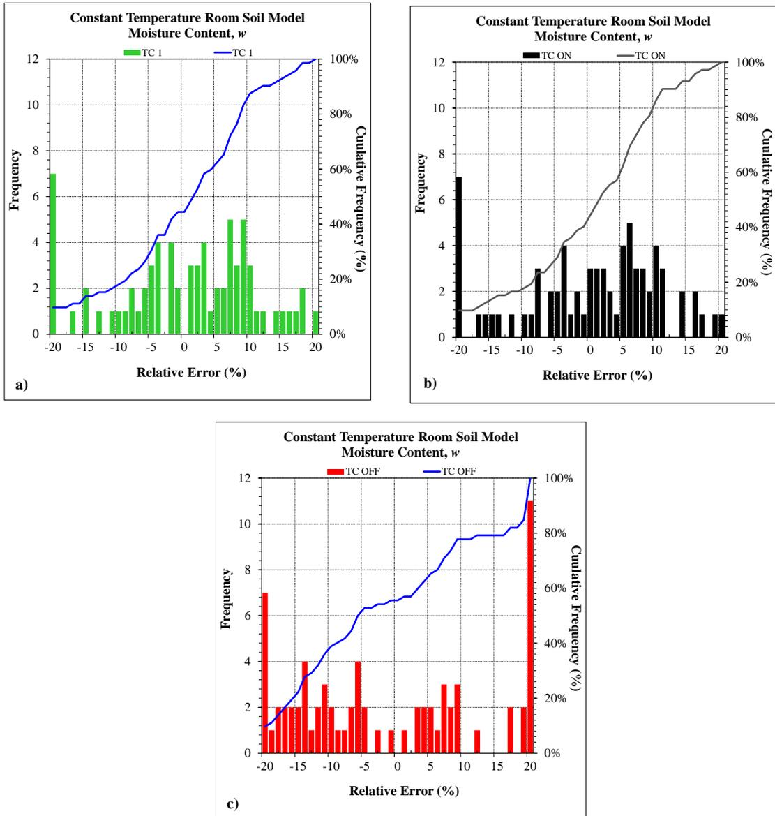
**Figure 8.16 Relative Error Histograms and CDF Plots – Constant Temperature Room Soil Model**
