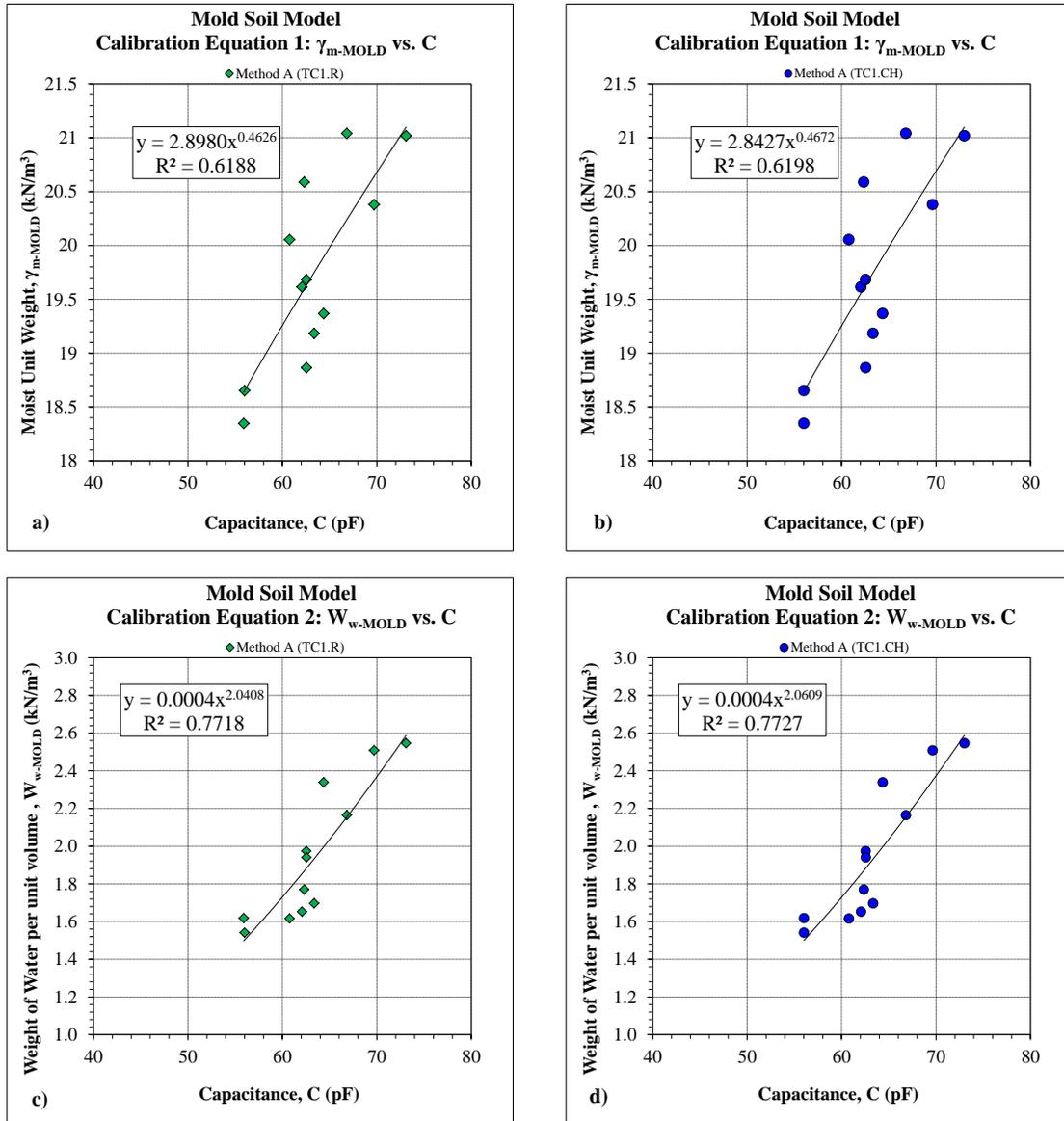
**Figure 9.1 Calibration Equations – Mold Soil Model (Method A)**
