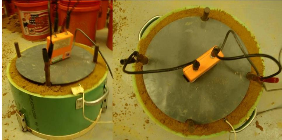
**Figure 5.4 Typical EDG setup in Mold**
