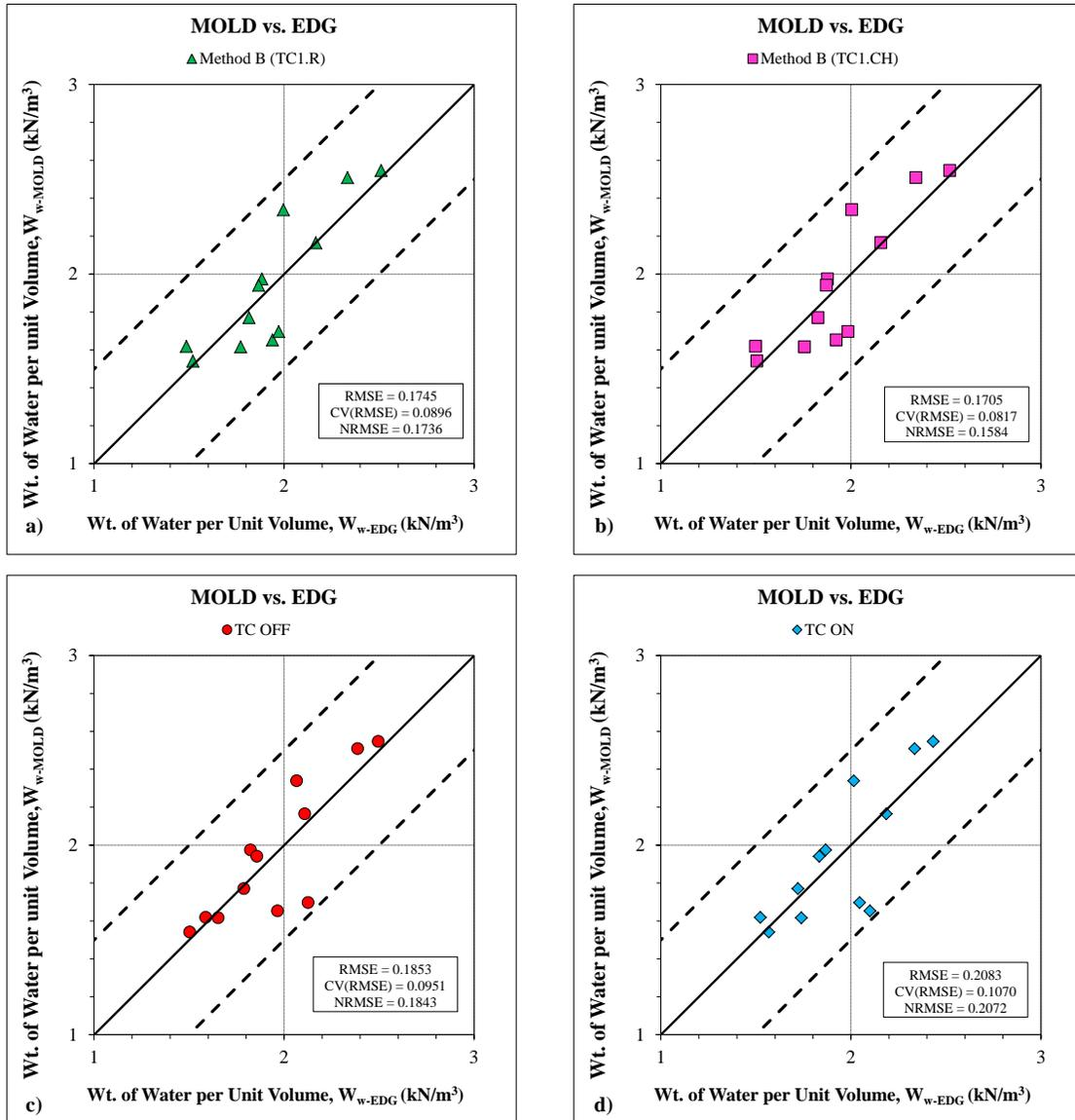
**Figure 9.10 1:1 Plots Mold Soil Model (Method B)**
