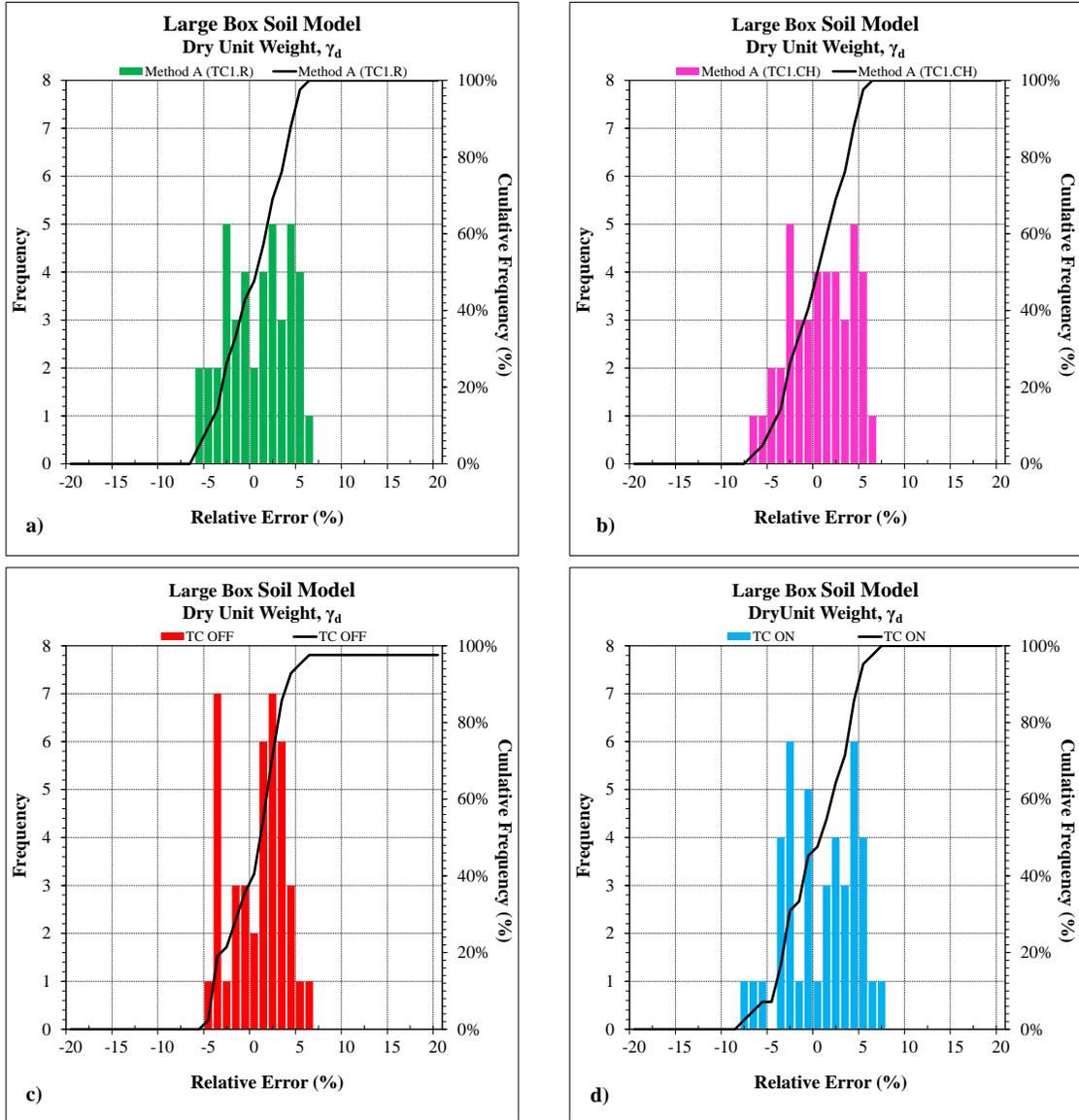
**Figure 9.31 Relative Error Histograms and CDF Plots – Large Box Soil Model (Method A)**
