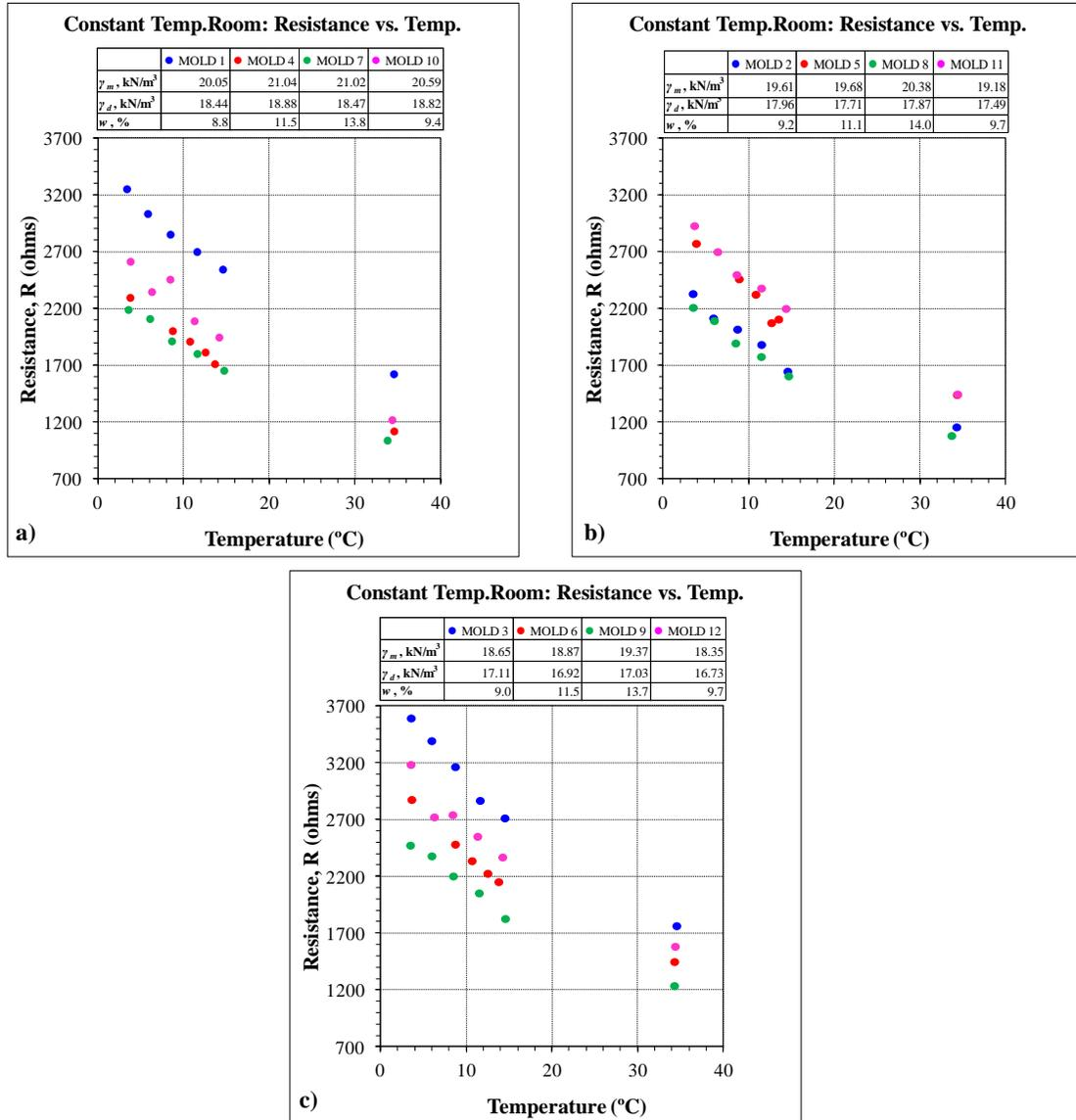
**Figure C.17 Constant Temperature Room Testing: Resistance vs. Temperature**
