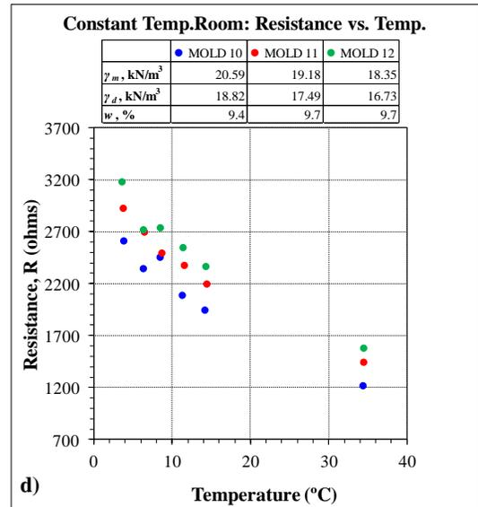
**Figure B.17 Constant Temperature Room Testing: Resistance vs. Temperature**
