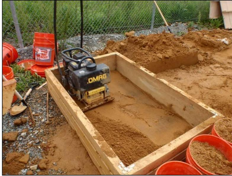
**Figure 6.1 Large Box used for simulated field conditions**
