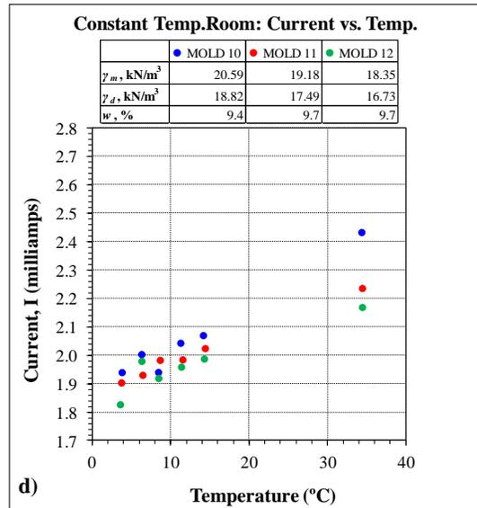
**Figure B.14 Constant Temperature Room Testing: Current vs. Temperature**
