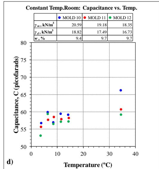
**Figure B.16 Constant Temperature Room Testing: Capacitance vs. Temperature**
