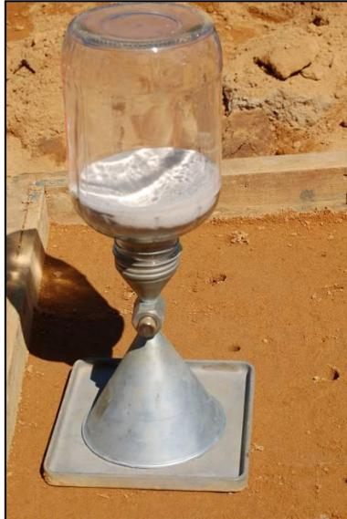
**Figure 6.9** Sand Cone test performed in Large Box
