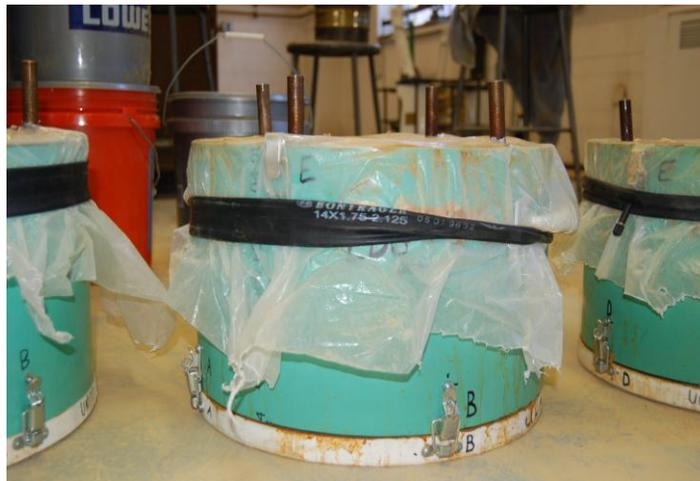
**Figure 7.1** A plastic sealing layer tightly secured to the compacted soil molds using rubber bicycle tire tubes
