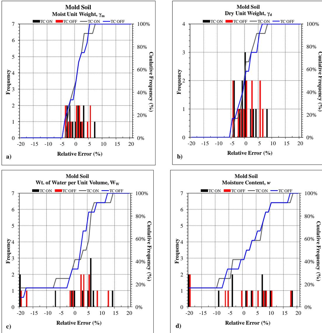
**Figure 5.7** Relative Error Histograms and CDF Plots – Mold Soil
