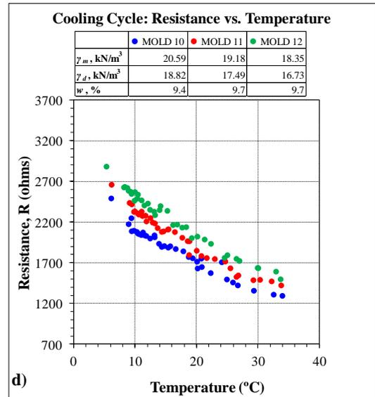
**Figure B.5 Cooling Cycle: Resistance vs. Temperature**
