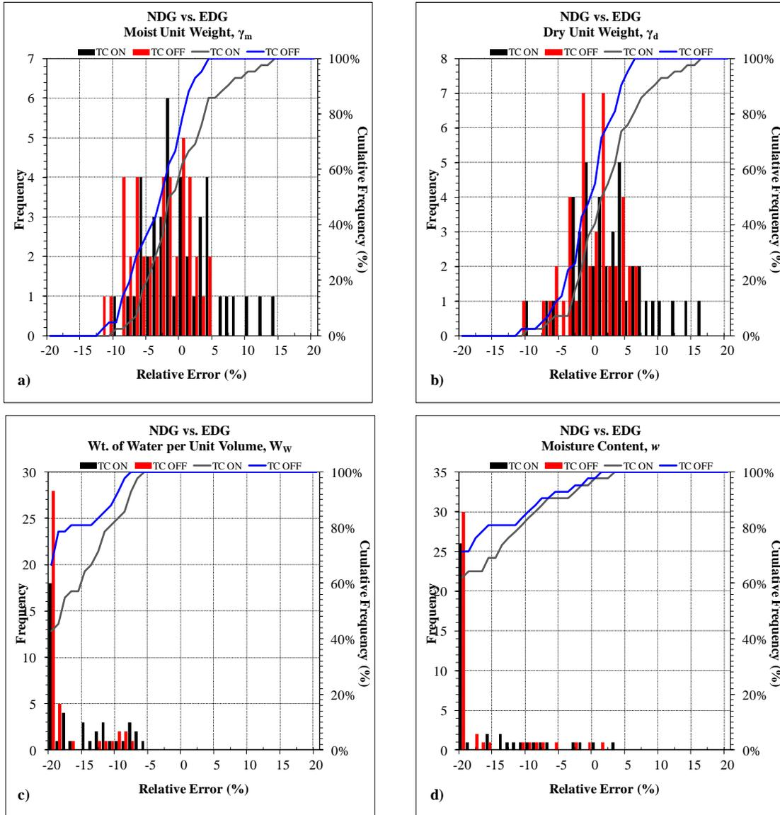
**Figure 6.21 Relative Error Histograms and CDF Plots – NDG vs. EDG (Mold Soil Model)**
