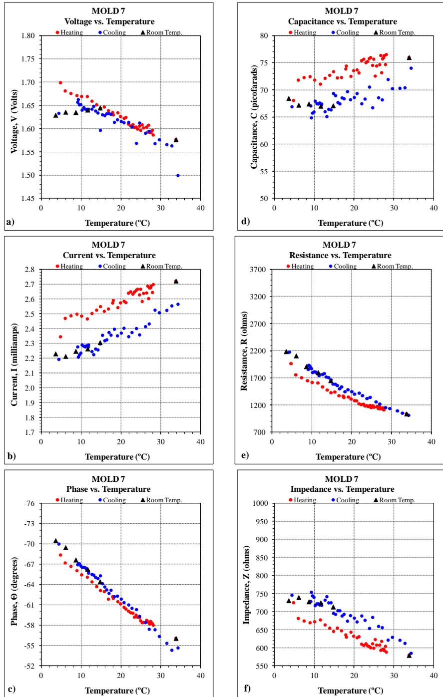
**Figure 7.11 Electrical Properties Recorded Using the EDG vs. Temperature (MOLD 7)**
