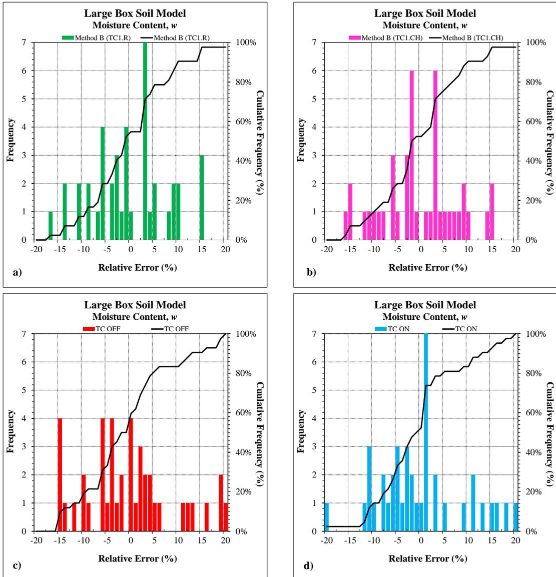
**Figure 9.36 Relative Error Histograms and CDF Plots – Large Box Soil Model (Method B)**
