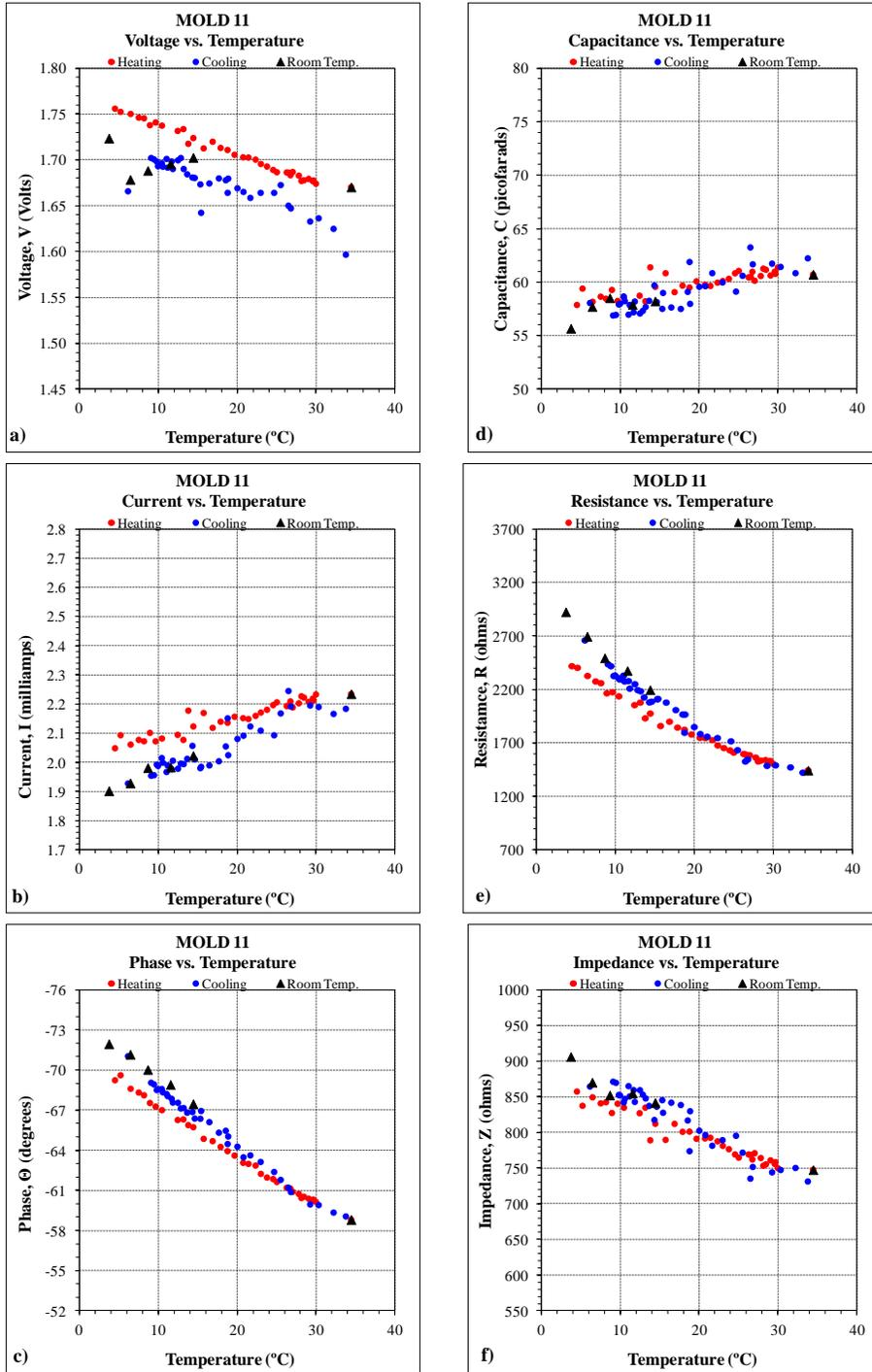
**Figure A.11 Electrical Properties Recorded Using the EDG vs. Temperature (MOLD 11)**
