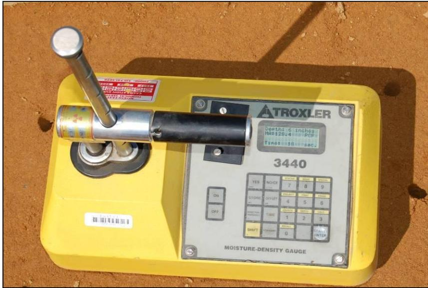
**Figure 6.8** NDG test performed in Large Box
