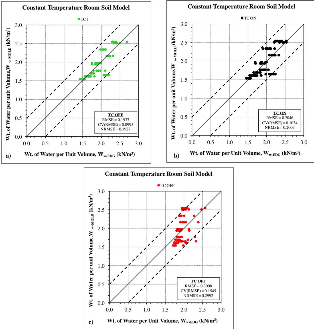
**Figure 8.6 1:1 Plots – Constant Temperature Room Soil Model**
