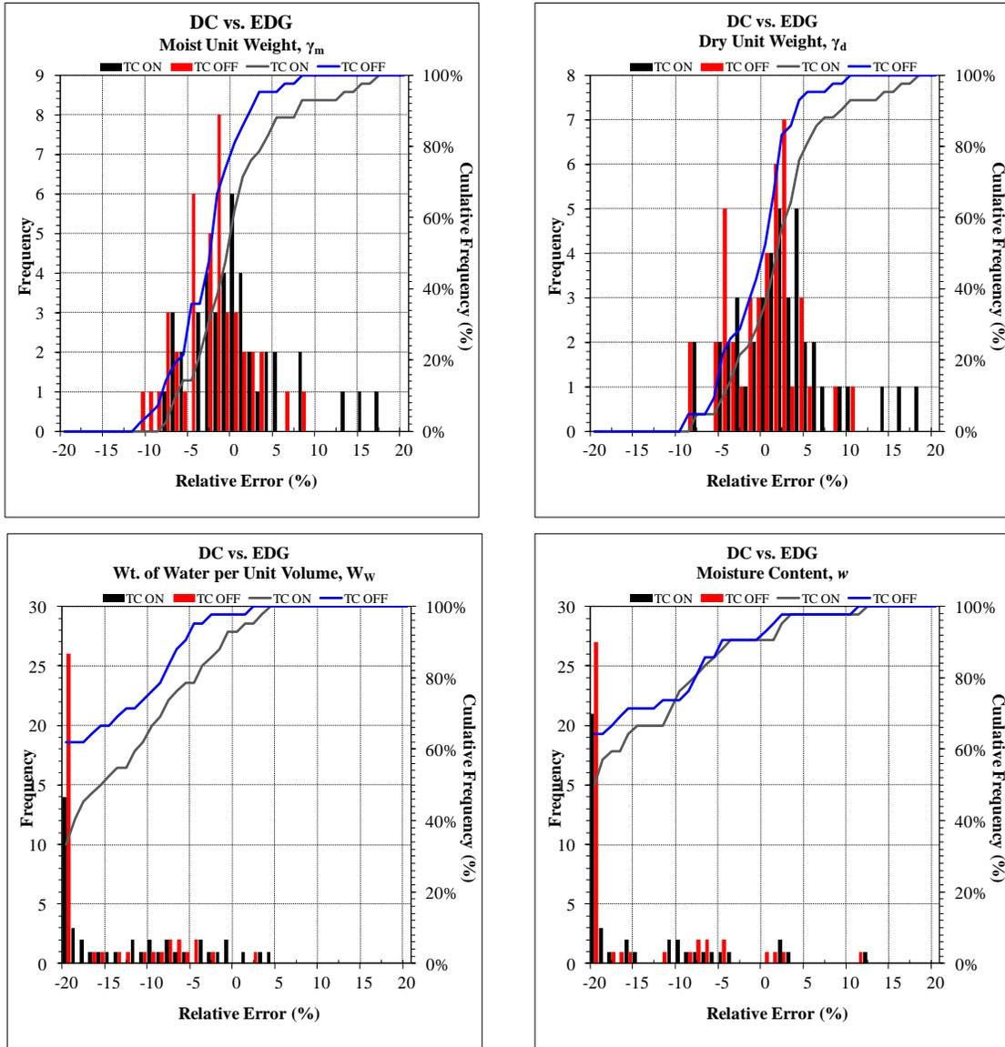
**Figure 6.23 Relative Error Histograms and CDF Plots – DC vs. EDG (Mold Soil Model)**
