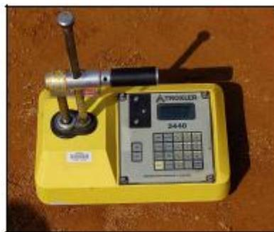
**Figure 2.1 Troxler 3440 Nuclear Density Gauge**
