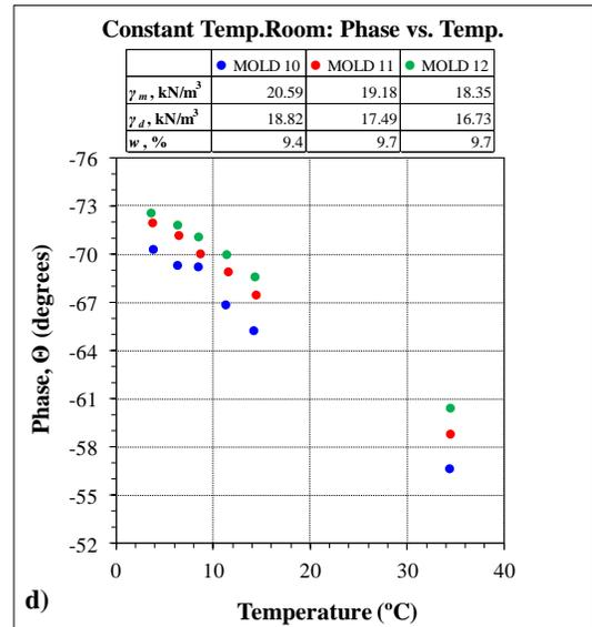
**Figure B.15 Constant Temperature Room Testing: Phase vs. Temperature**
