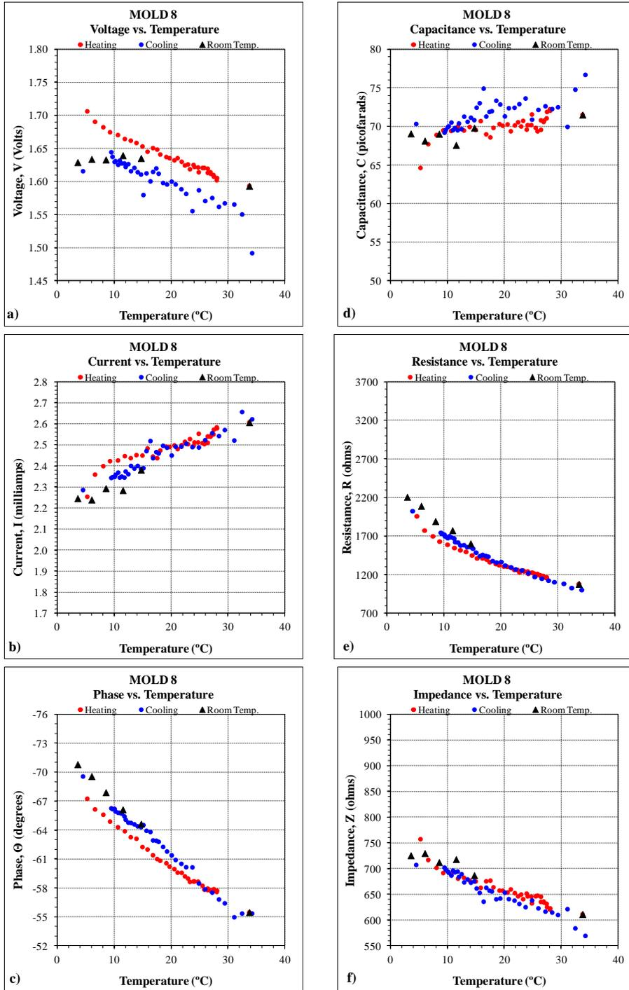
**Figure A.8 Electrical Properties Recorded Using the EDG vs. Temperature (MOLD 8)**
