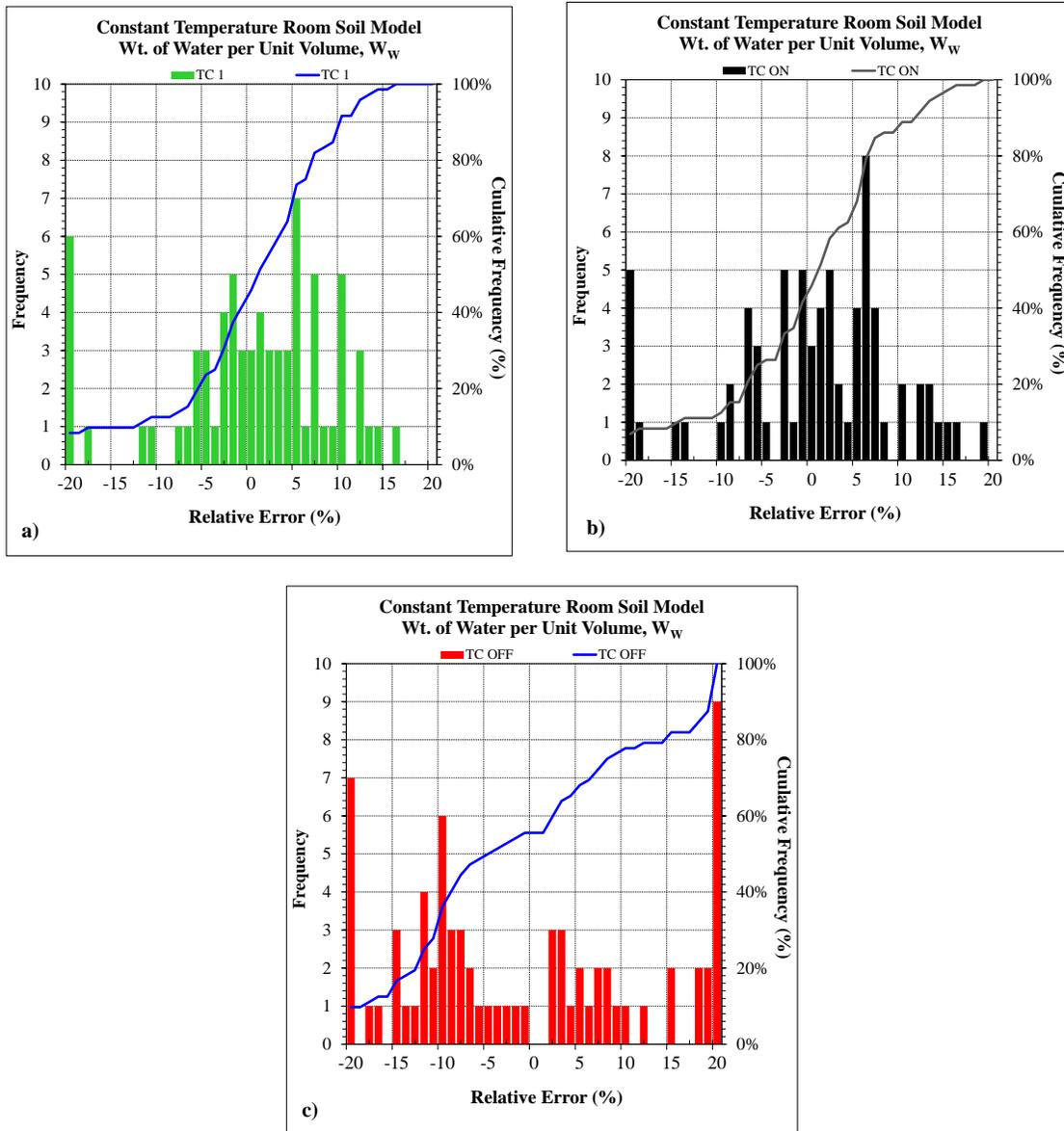
**Figure 8.14 Relative Error Histograms and CDF Plots – Constant Temperature Room Soil Model**
