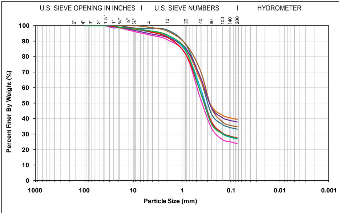
**Figure 4.3 Gradation distributions for soil samples from Dover in situ test locations**
