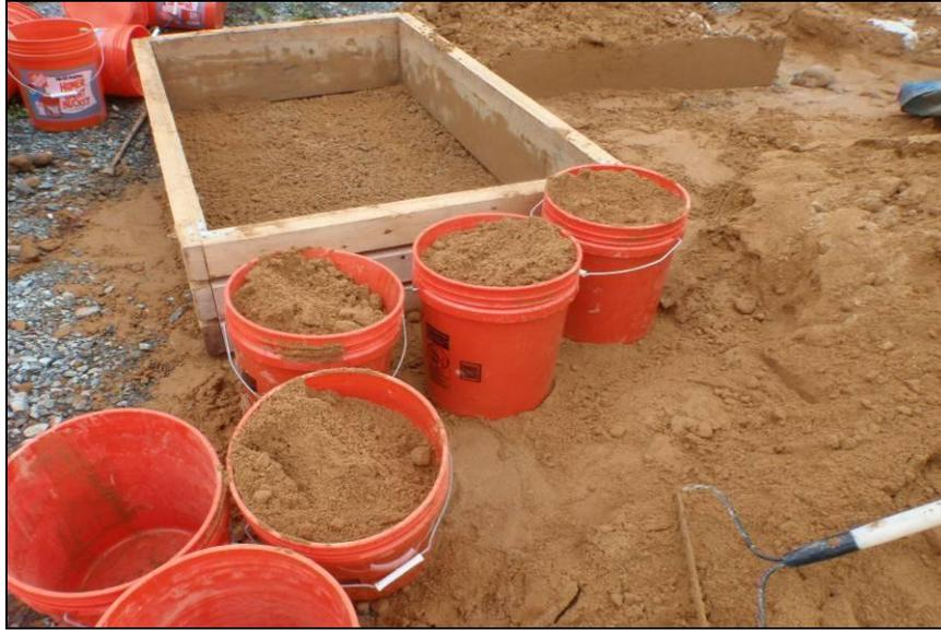
**Figure 6.4** Soil Placed in buckets for volume control
