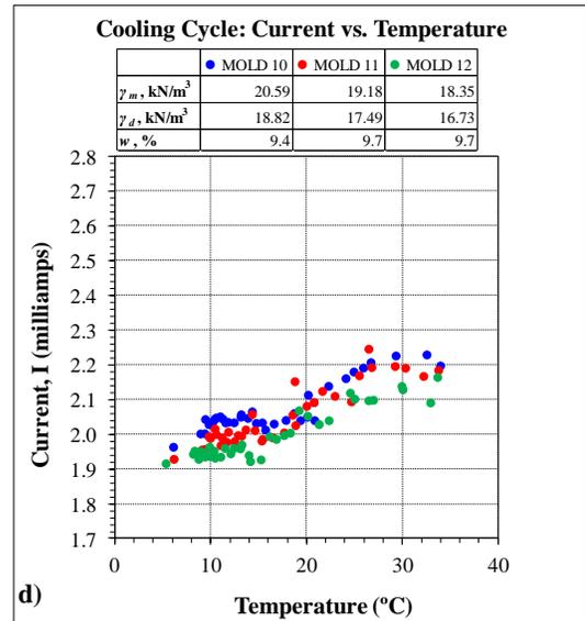
**Figure B.2 Cooling Cycle: Current vs. Temperature**
