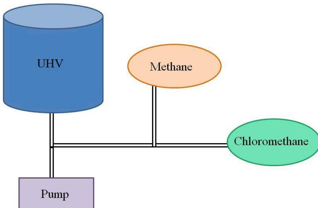
**Figure 8. Gas jet apparatus.**
