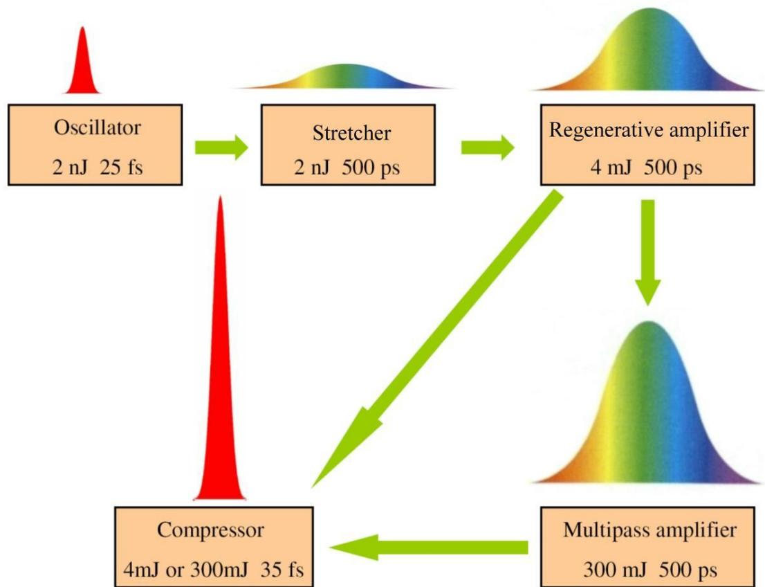
**Figure 6. Chirped pulse amplification (CPA) system scheme [3]**
