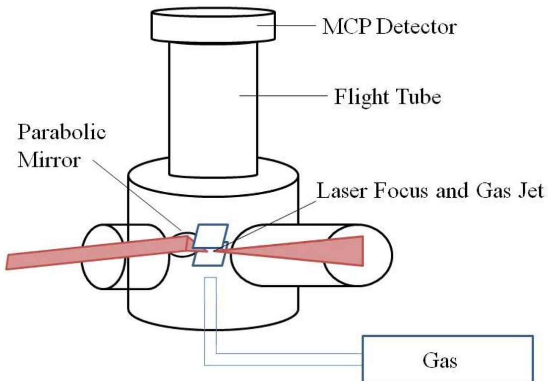
**Figure 7. Ultra-high vacuum (UHV) chamber diagram.**
