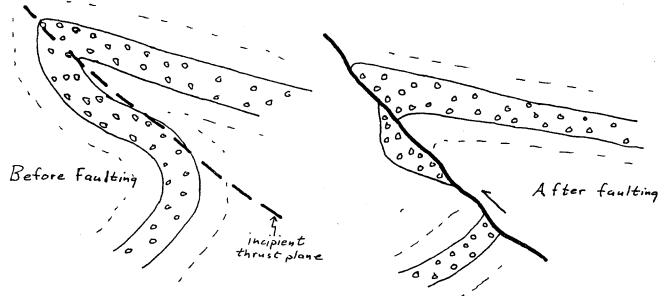
The key to the structural interpretation here is the lightcolored conglomerate bed. Try to follow it completely through the fold and across the fault; imagine what the structure would have looked like when the conglomerate was a continuous stratum.
