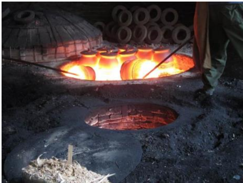
Figure 24. Orange-hot pots are removed from kiln and immediately placed into a glaze kiln (shown in the foreground).
