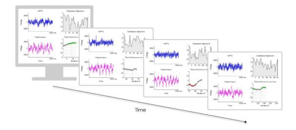
Figure 4 Schematic of the closed-loop for detecting high HPC-mPFC theta coherence in real-time. Upper left panel on screen depicts mPFC LFP (blue), bottom left panel depicts HPC LFP (magenta), top right panel depicts wideband coherence spectrum, and bottom right depicts coherence specific to the theta frequency band. Note the dynamic tracking of HPC-mPFC theta coherence in the bottom right portion of the screen with green and red signaling high and low levels of theta coherence.
