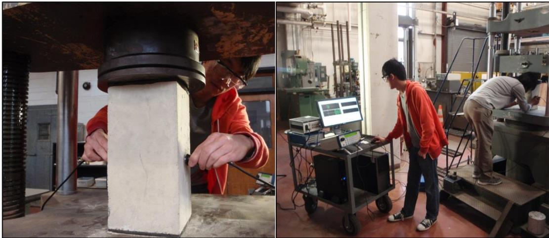
Figure 11: (left) concrete block with shear transducers and (right) compression machine and data acquisition system, DAQ
