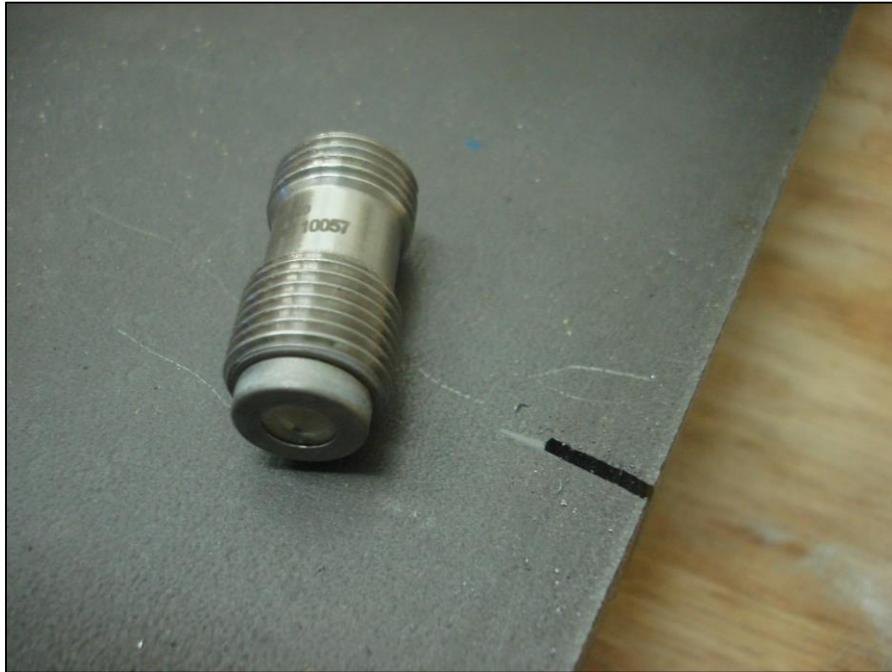
Figure 37: Point-contact sensor used in the experiment
