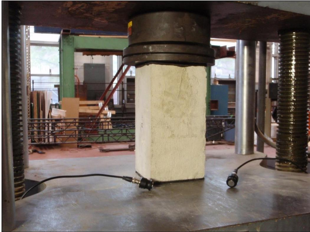
Figure 12: Concrete block specimen in compression machine with bearing pads on the top and bottom
