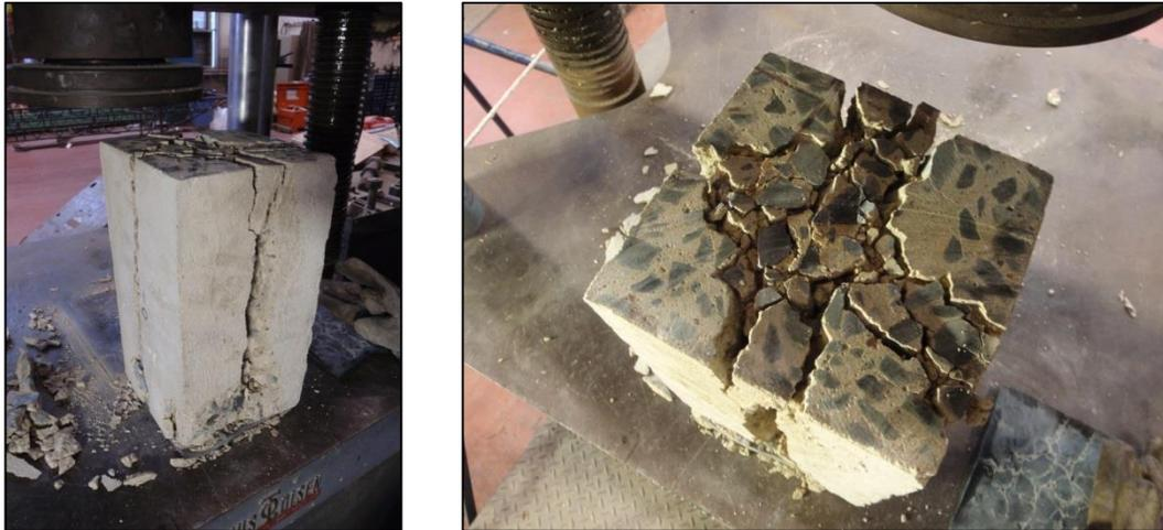
Figure 14: Concrete block 1 failure: (left) side view and (right) top view
