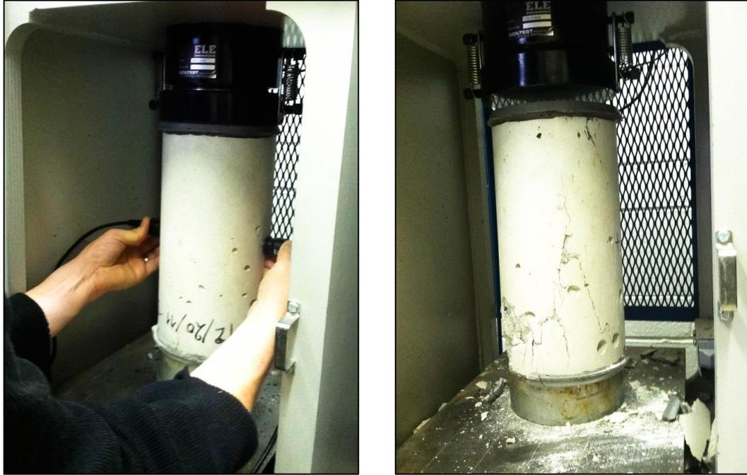
Figure 10: (left) Concrete cylinder setup and (right) same cylinder at failure
