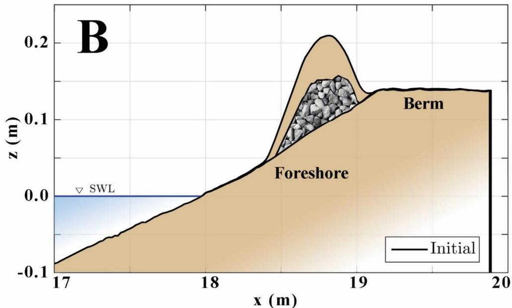
Figure 2.8: Test series buried seawall (B) initial profile
