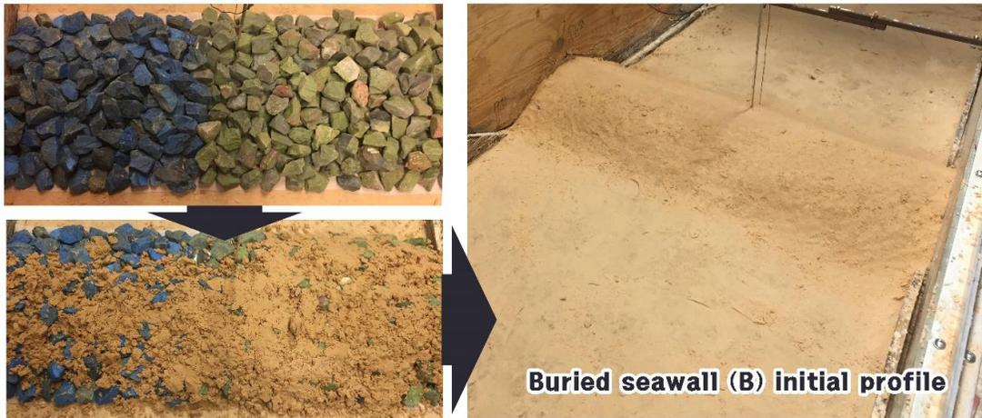
Figure 2.7: Process of building buried seawall (B) initial profile
