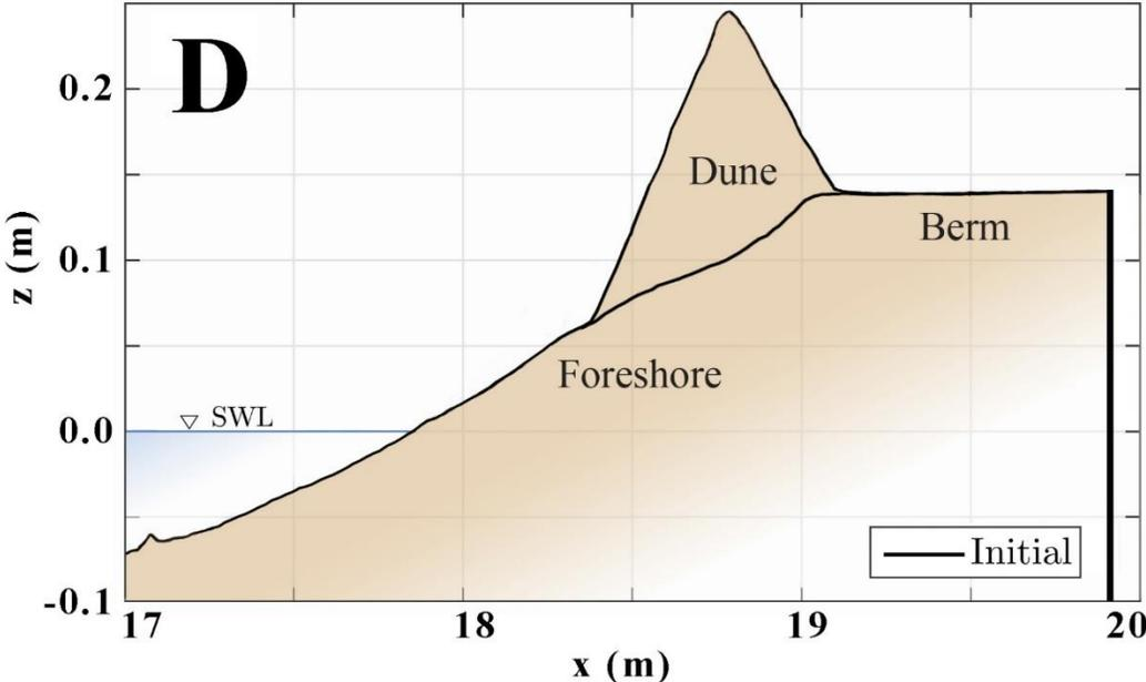
Figure 2.4: Test series dune only (D) initial profile
