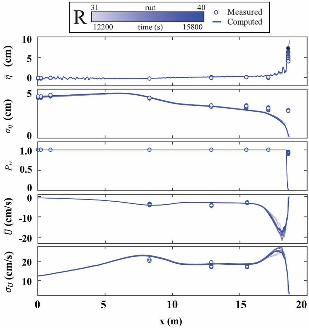
Figure 5.10: Mean and SD of free surface elevation  $\eta$  and horizontal velocity  $U$  together with wet probability  $P_w$  for 10 runs during time  $t = 12,000 - 16,000$  s in series R
