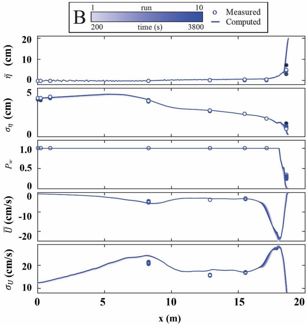
Figure 5.11: Mean and SD of free surface elevation  $\eta$  and horizontal velocity  $U$  together with wet probability  $P_w$  for 10 runs during time  $t = 0 - 4,000$  s in series B
