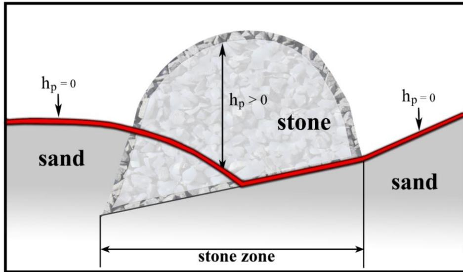
Figure 4.3: Stone porous layer of thickness  $h_p$  with no sand inside
