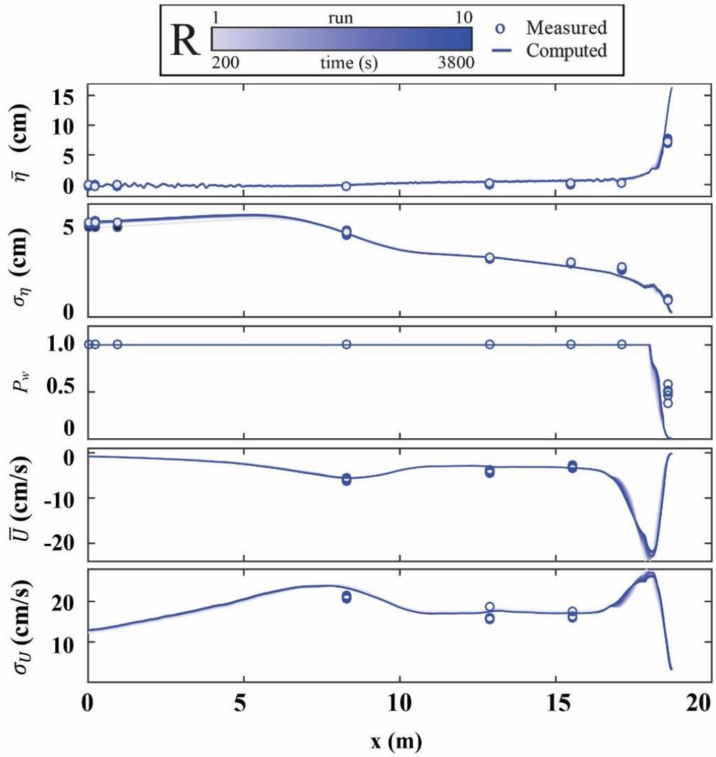
Figure 5.7: Mean and SD of free surface elevation  $\eta$  and horizontal velocity  $U$  together with wet probability  $P_w$  for 10 runs during time  $t = 0 - 4,000$  s in series R
