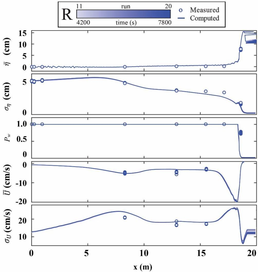
Figure 5.8: Mean and SD of free surface elevation  $\eta$  and horizontal velocity  $U$  together with wet probability  $P_w$  for 10 runs during time  $t = 4,000 - 8,000$  s in series R
