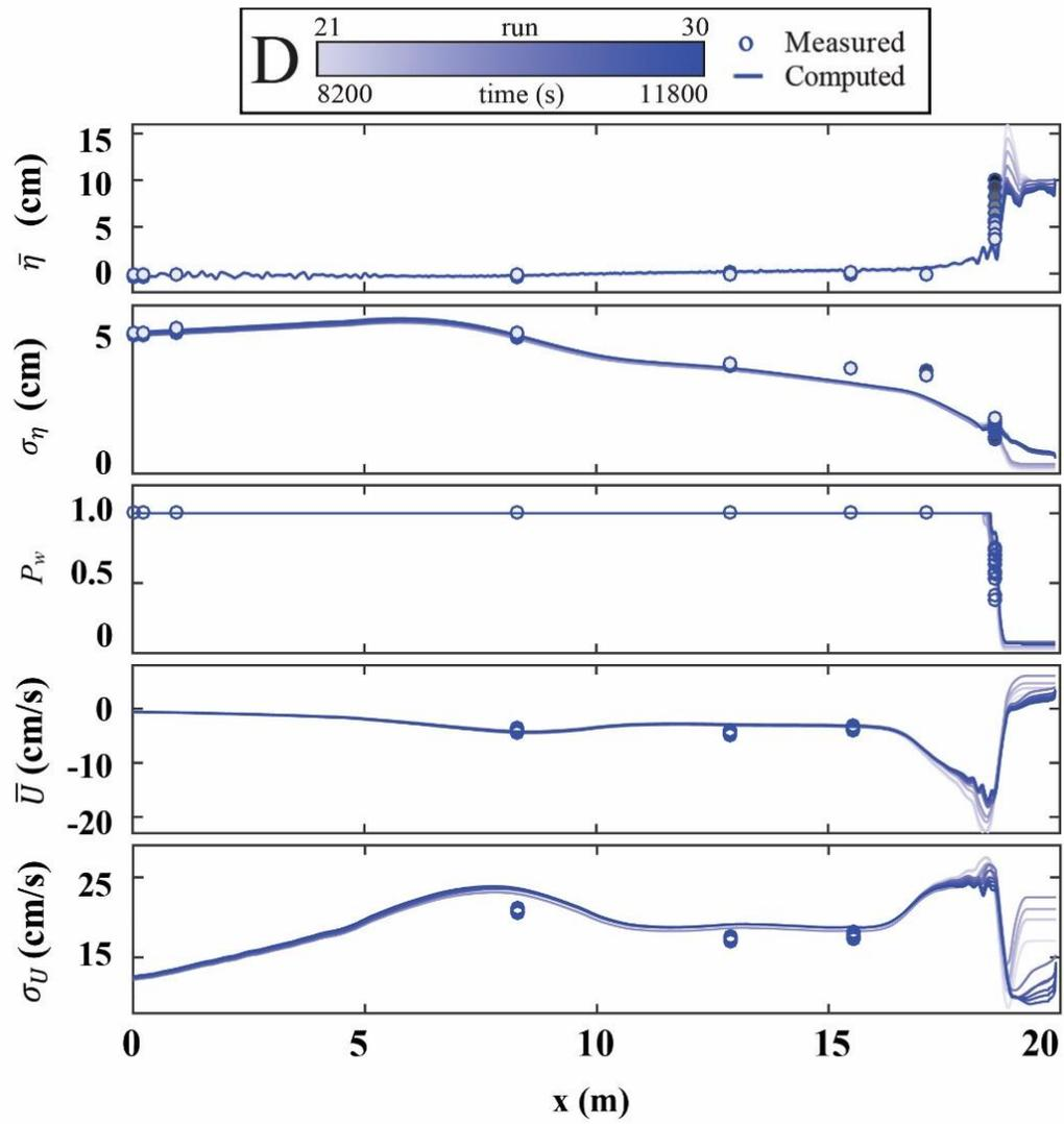
Figure 5.6: Mean and SD of free surface elevation  $\eta$  and horizontal velocity  $U$  together with wet probability  $P_w$  for 10 runs during time  $t = 8,000 - 12,000$  s in series D
