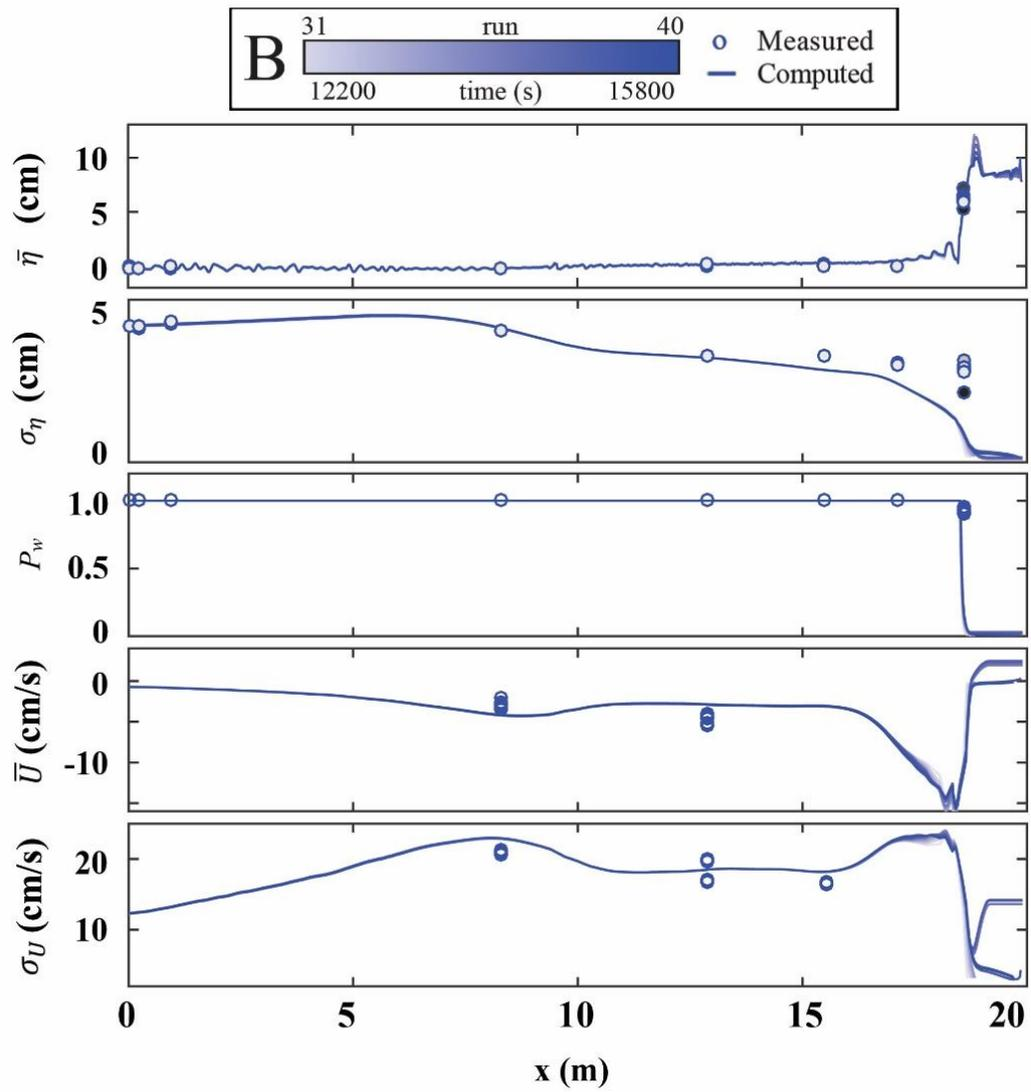
Figure 5.14: Mean and SD of free surface elevation  $\eta$  and horizontal velocity  $U$  together with wet probability  $P_w$  for 10 runs during time  $t = 12,000 - 16,000$  s in series B
