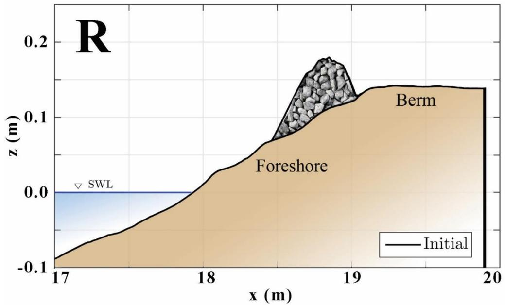
Figure 2.5: Test series rock seawall (R) initial profile
