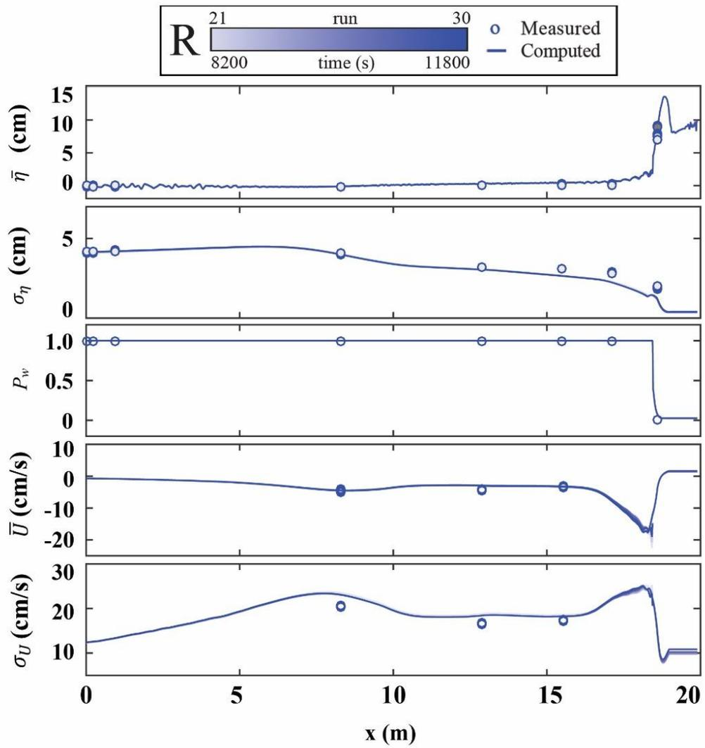
Figure 5.9: Mean and SD of free surface elevation  $\eta$  and horizontal velocity  $U$  together with wet probability  $P_w$  for 10 runs during time  $t = 8,000 - 12,000$  s in series R
