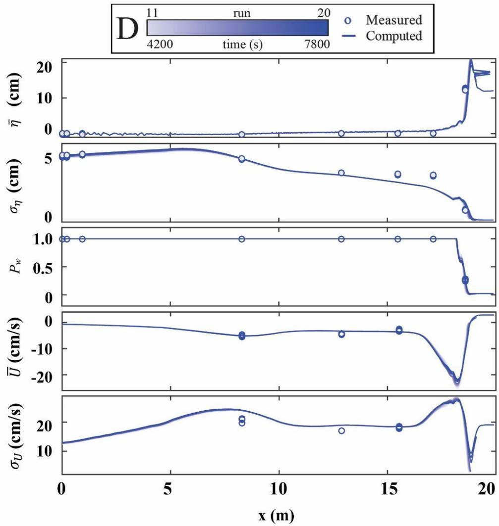
Figure 5.5: Mean and SD of free surface elevation  $\eta$  and horizontal velocity  $U$  together with wet probability  $P_w$  for 10 runs during time  $t = 4,000 - 8,000$  s in series D
