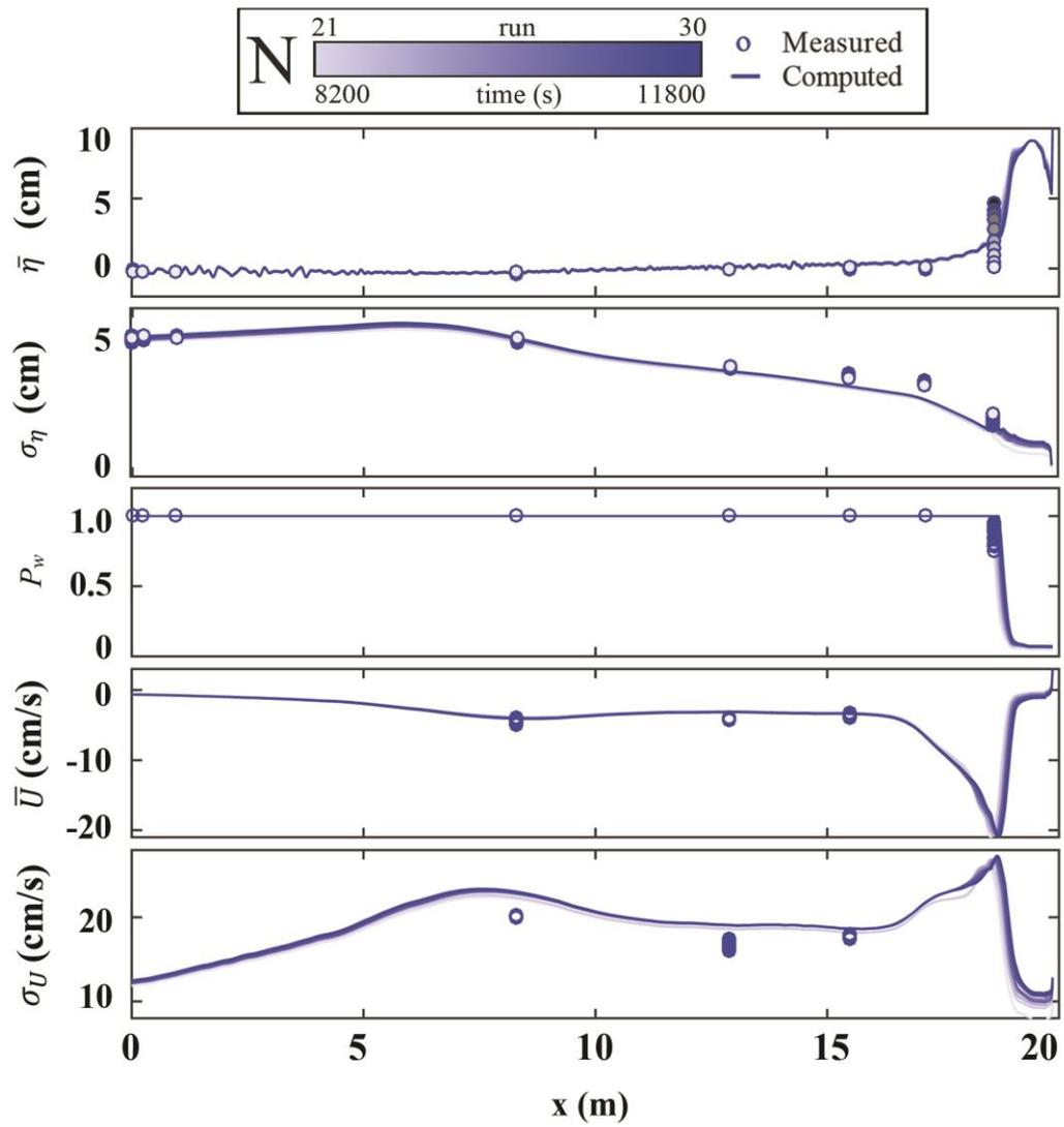
Figure 5.3: Mean and SD of free surface elevation  $\eta$  and horizontal velocity  $U$  together with wet probability  $P_w$  for 10 runs during time  $t = 8,000 - 12,000$  s in series N
