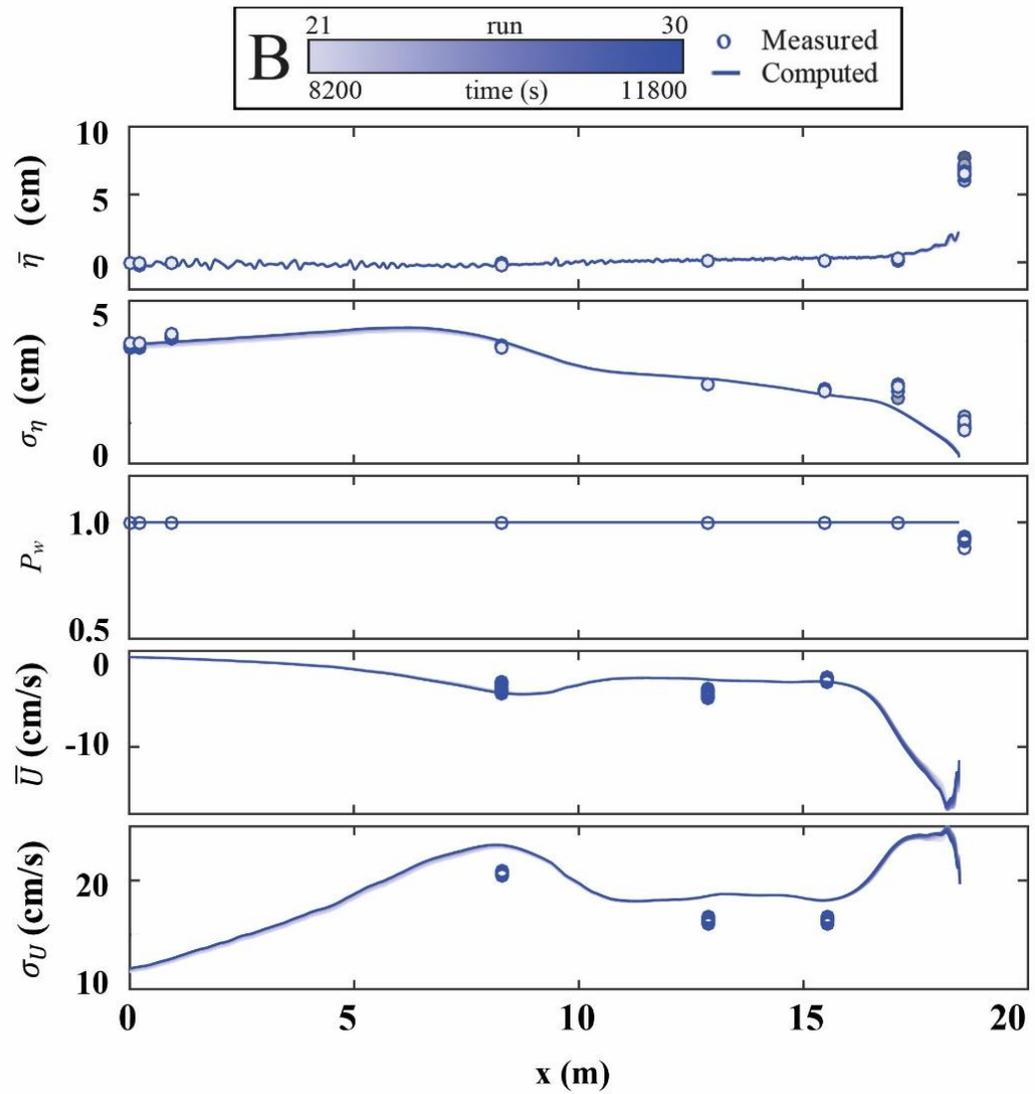
Figure 5.13: Mean and SD of free surface elevation  $\eta$  and horizontal velocity  $U$  together with wet probability  $P_w$  for 10 runs during time  $t = 8,000 - 12,000$  s in series B
