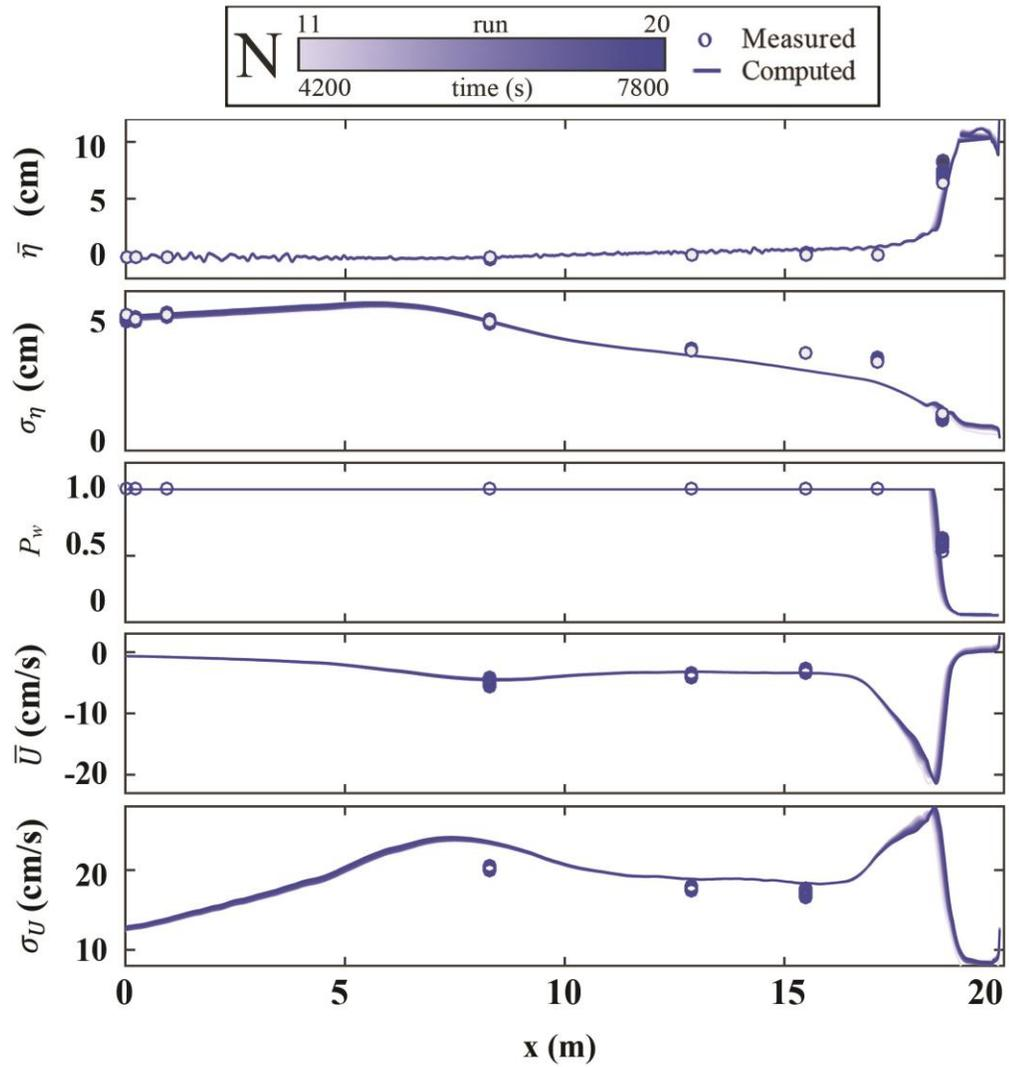
Figure 5.2: Mean and SD of free surface elevation  $\eta$  and horizontal velocity  $U$  together with wet probability  $P_w$  for 10 runs during time  $t = 4,000 - 8,000$  s in series N
