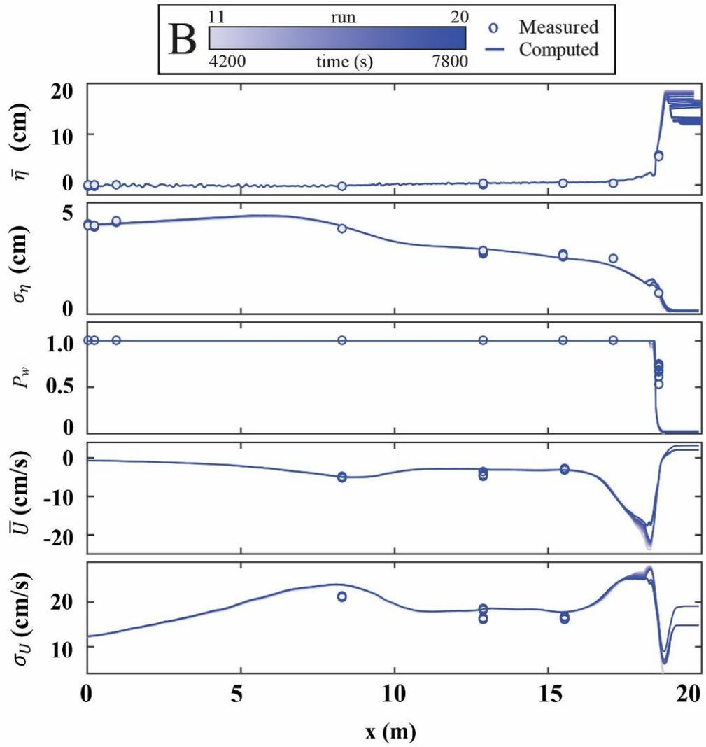
Figure 5.12: Mean and SD of free surface elevation  $\eta$  and horizontal velocity  $U$  together with wet probability  $P_w$  for 10 runs during time  $t = 4,000 - 8,000$  s in series B
