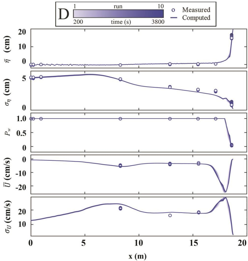
Figure 5.4: Mean and SD of free surface elevation  $\eta$  and horizontal velocity  $U$  together with wet probability  $P_w$  for 10 runs during time  $t = 0 - 4,000$  s in series D
