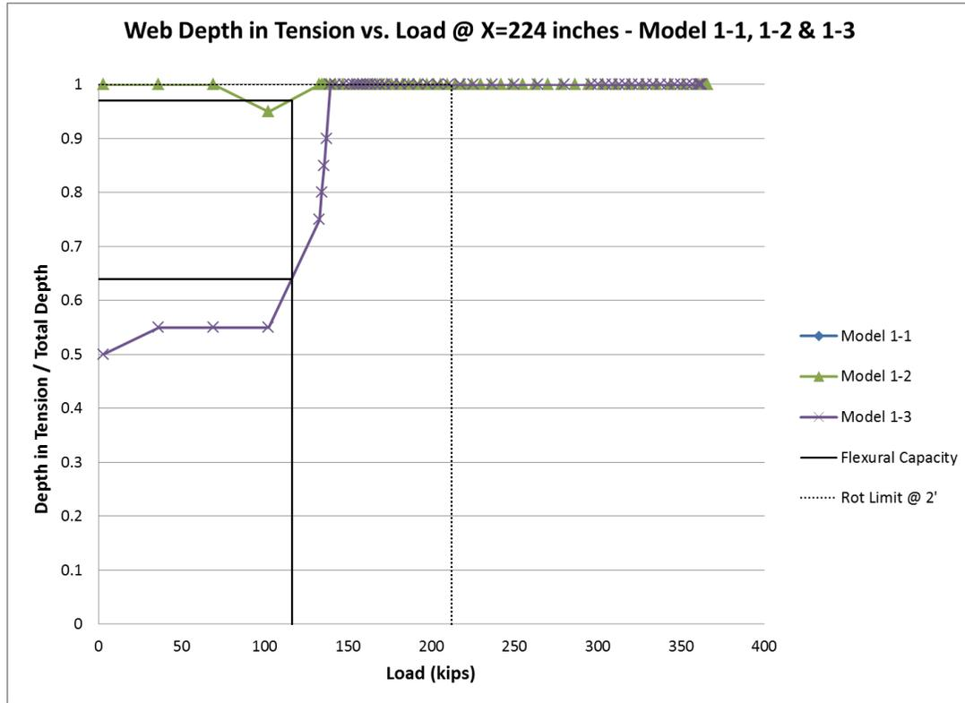
**Figure 4.12.** Load vs. web tension depth at 224 inches for Model 1-1, Model 1-2 & Model 1-3
