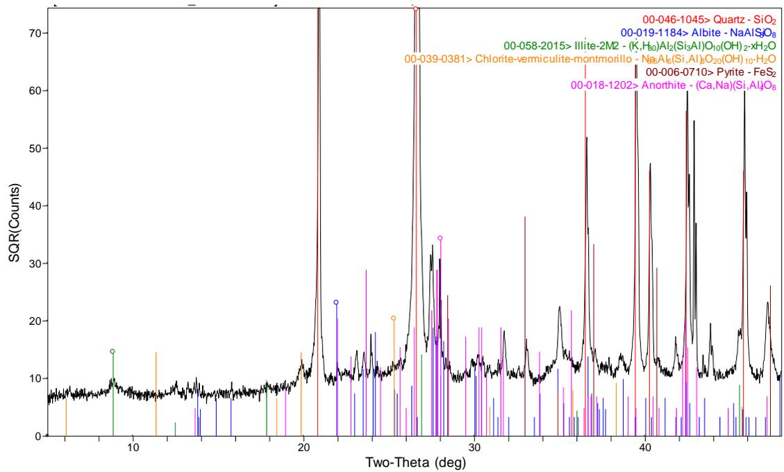
Figure 6a Mineralogical composition of sediment (0-2 cm) from site A (obtained by Tamas Varga at PNNL). Different color lines represent peaks of different minerals fitted to the measured spectra.
