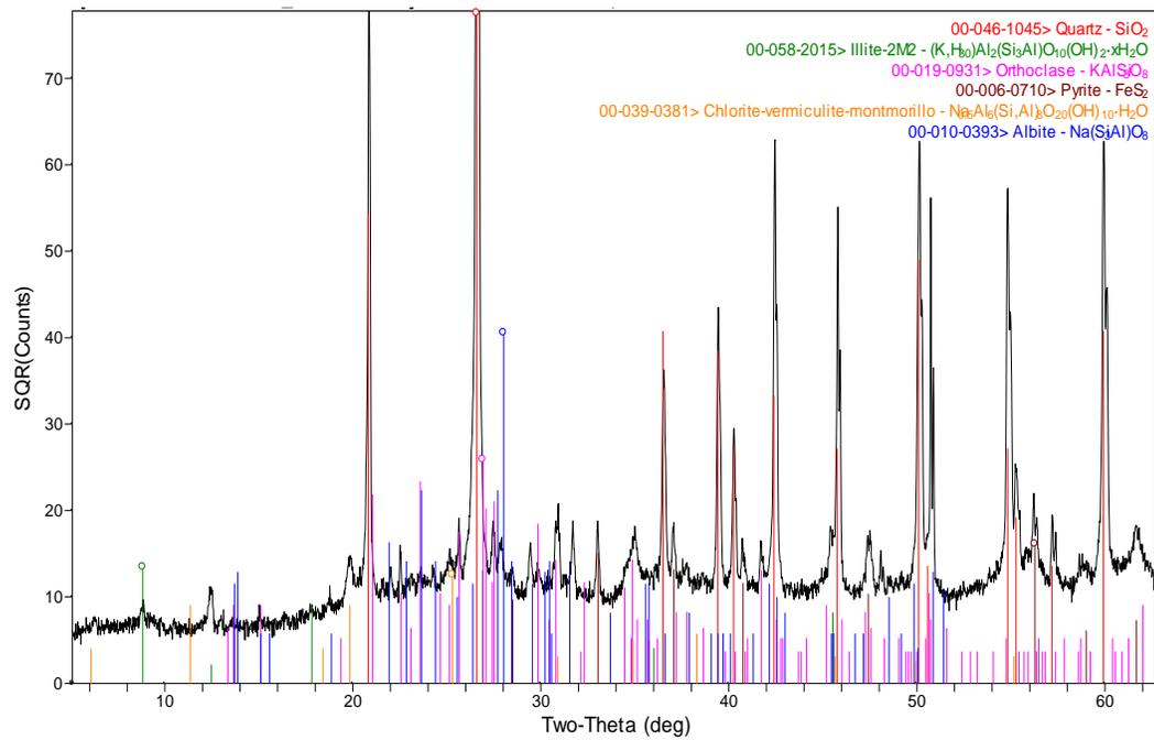
Figure 6b Mineralogical composition of sediment (0-2 cm) from site H (obtained by Tamas Varga at PNNL). Different color lines represent peaks of different minerals fitted to the measured spectra.
