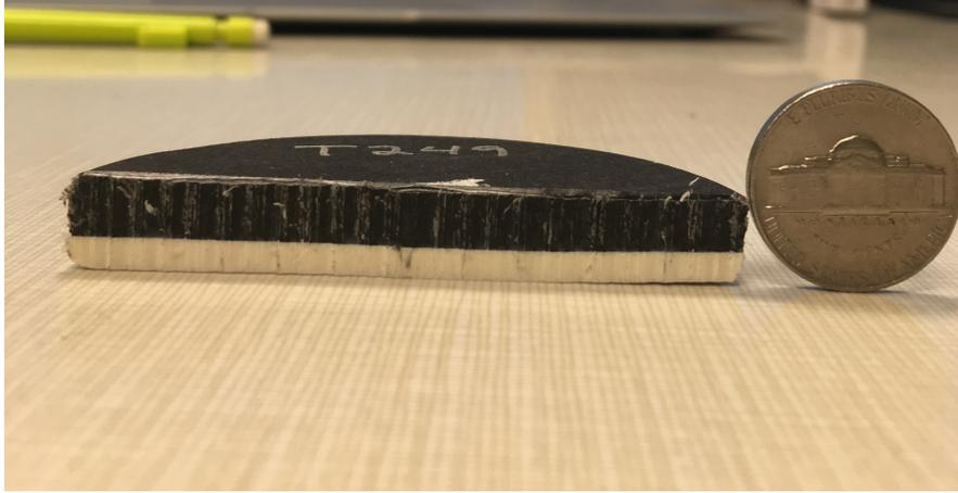
**Figure 2.4:** A piece of IceTop tank and a US nickel for scale. The black top is the outer polyethylene layer of a tank. The white bottom layer is the layer of reflective zirconium.
