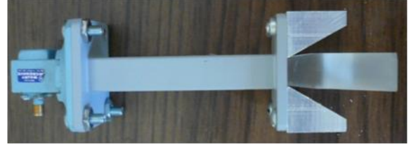
Figure 5.4 Fabricated I/O coupler.
