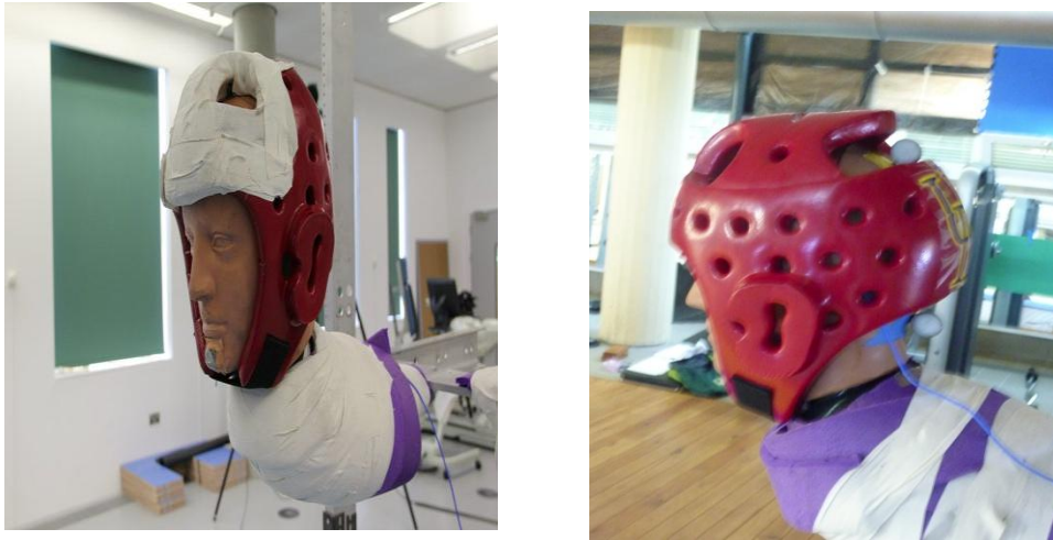
Figure 4. Reflective apex, occiput and chin markers.
