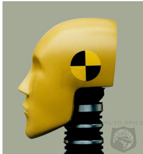
Figure 10. H3D neck with individual cervical disks.
