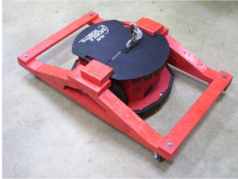
Figure 2 Pioneer 3-DX with additional stability supports
