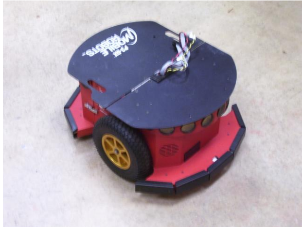
Figure 1 Pioneer 3-DX robot provided by MobileRobots, Inc.
