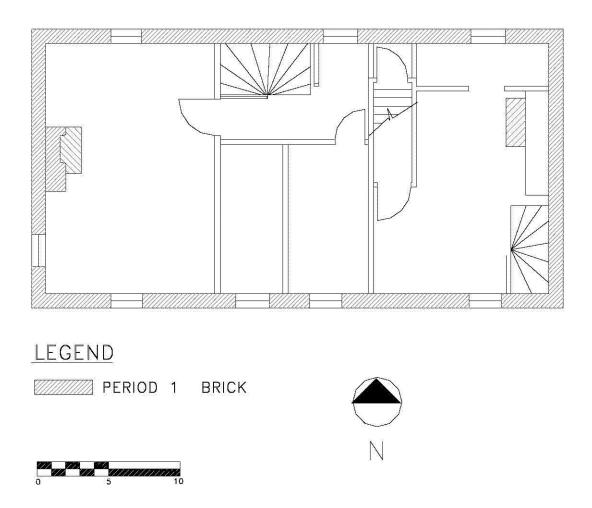
Figure 70: Mansion Farm Tenement, second floor plan.
