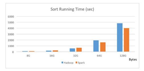
Figure 5.7: Running Time Comparison for Sort Running on Hadoop and Spark
