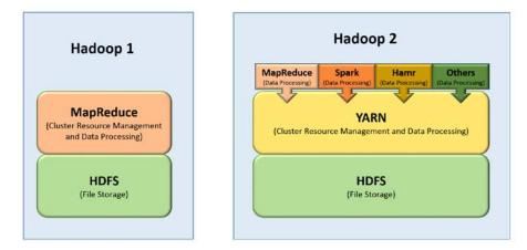
Figure 2.4: Differences between the Components of Hadoop1 and Hadoop 2
