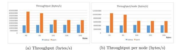
Figure 5.6: Throughput Comparison for Running WordCount on Hadoop and Spark
