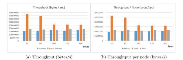
Figure 5.24: Throughput Comparison for WordCount Running on Hadoop, Spark and Hamr
