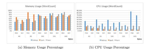
Figure 5.23: Memory and CPU Comparison for WordCount Running on Hadoop, Spark and HAMR
