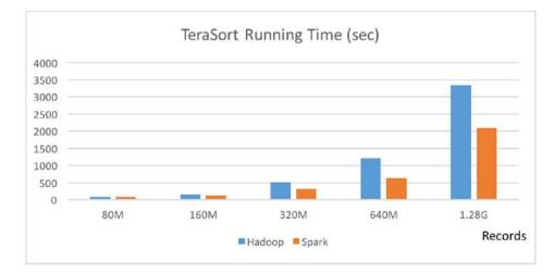
Figure 5.10: Running Time Comparison for TeraSort Running on Hadoop and Spark
