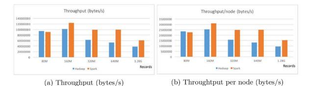
Figure 5.12: Throughput Comparison for Running TeraSort on Hadoop and Spark
