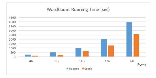
Figure 5.4: Running Time Comparison for WordCount Running on Hadoop and Spark
