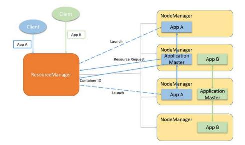
Figure 2.3: YARN (MapReduce 2.0). The cluster including one master and four slave nodes.[5] Application B submitted by the green client has ran on the cluster. The blue client just submitted Application A. The ResourceManager launched an ApplicationMaster for it on the second NodeManager. AM requested resources from RM and two containers were launched by RM. The container IDs would be sent back to AM. Application A began to execute.
