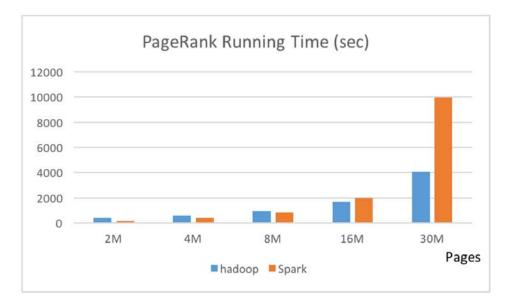
Figure 5.1: Running Time Comparison for PageRank running on Hadoop and Spark
